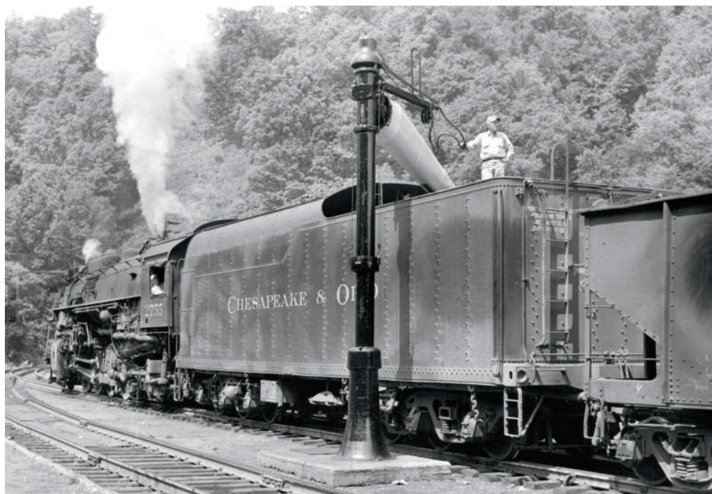
1 The prototype. The fireman has a firm grip on the spout stop as he fills the tender of C&O class K-4 2-8-4 No. 2755 with water. This Poage water column was located at Sproul, W.Va., in the southwest part of the state. Gene L. Huddleston photo
