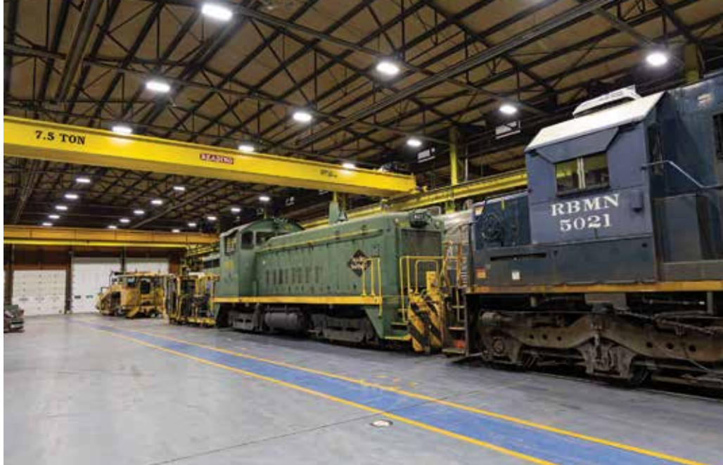
A new locomotive shop is part of the R&N's Nesquehoning campus, a former fire apparatus plant acquired by the railroad in 2022. SW8 No. 801 has positioned SD50 No. 5021 for the installation of a rebuilt prime mover.
