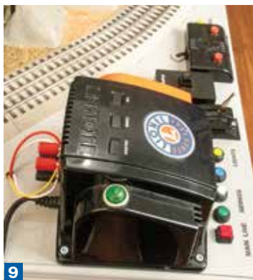
9 The control panel is located on a corner of the left table. The wires are routed underneath to the various switches, buttons, and controllers. From there they go to the track and accessories.
