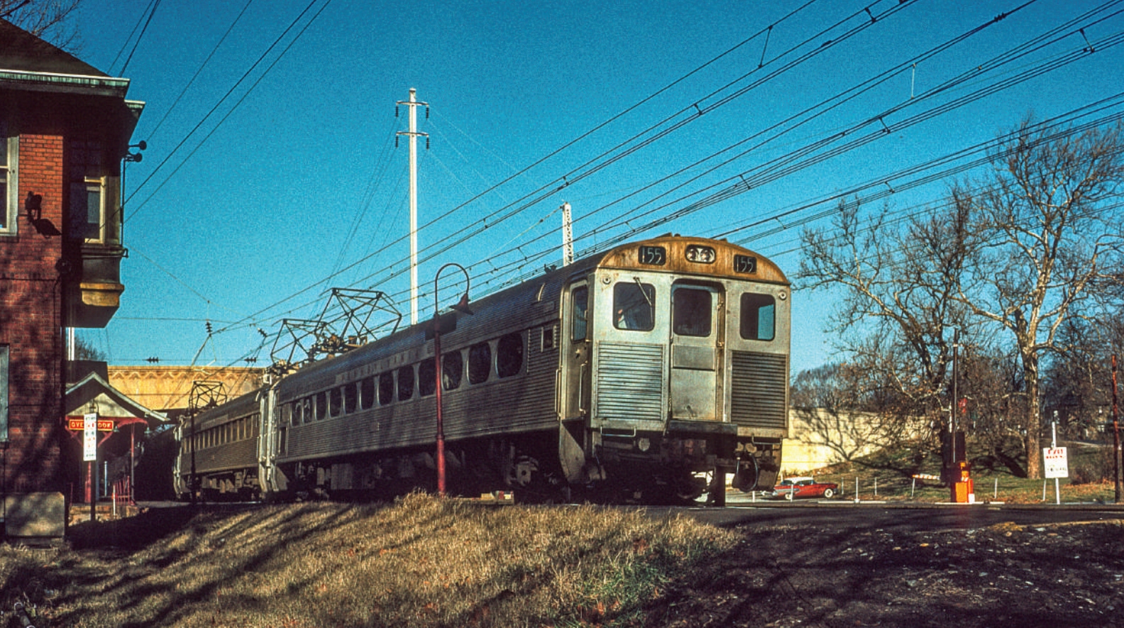
On Dec. 7, 1958, PRR Pioneer III multiple units pause at Overbrook, Pa., with an inbound train for Philadelphia's Suburban Station. The experimental Pioneer III units used full pantographs that make them easy to distinguish from the later Silverliners that used the Faiveley "half pantograph."
