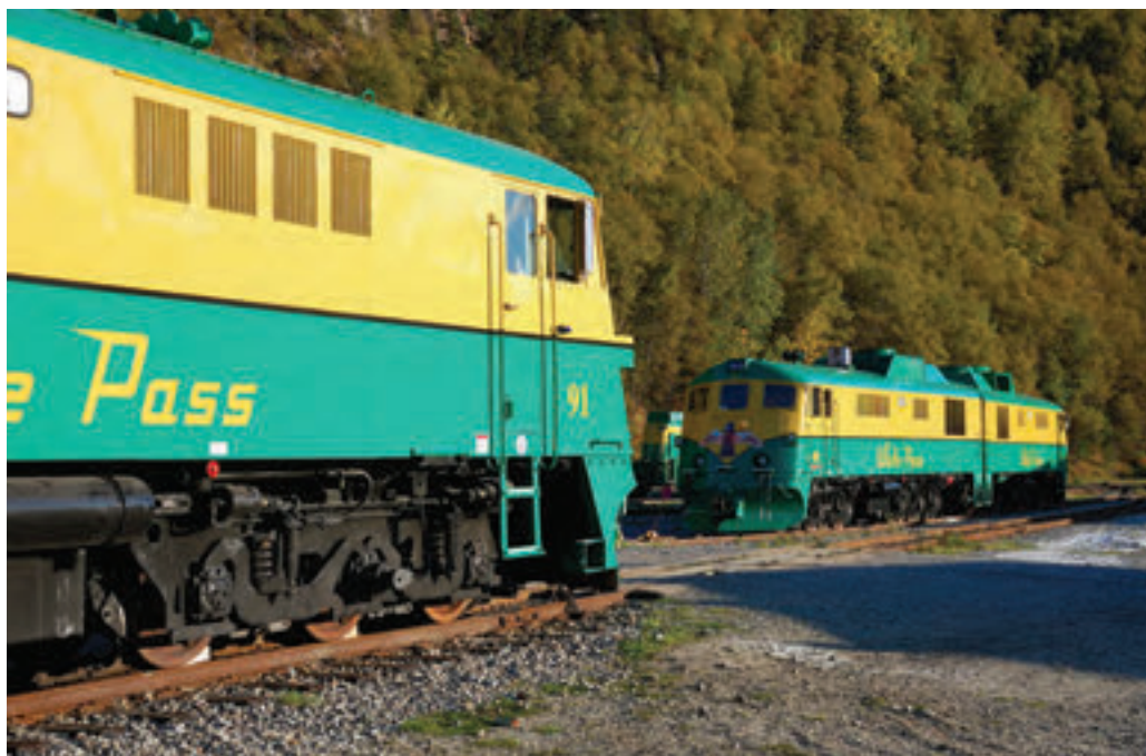
A few of the rebuilt units rest in Skagway. A significant spotting feature of these units is the streamlined fairing on the roof at the rear of the locomotives. The originals had a different appearance, as shown in the photo on page 40.
