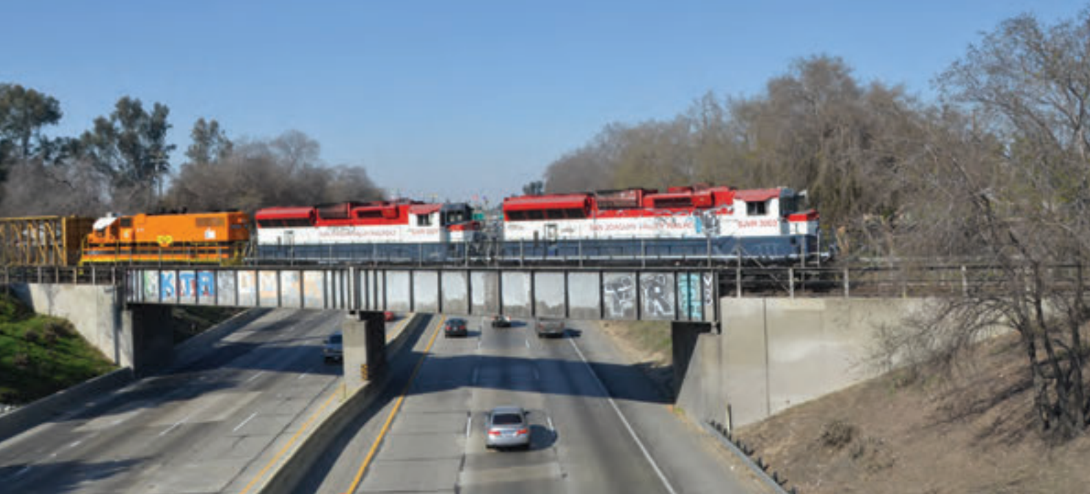
An eastbound San Joaquin Valley freight rolls through Fresno on Feb. 17, 2018 behind PR30B No. 3003. The PR30Bs are four-axle Electro-Motive units manufactured by Progress Rail with 2,995 hp Caterpillar engines aftertreatment-equipped to reach Tier 4 emission standards.
