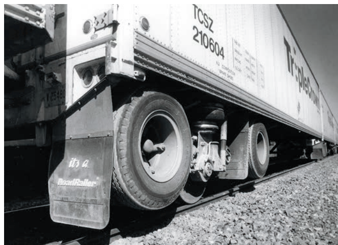
▲ Later versions of the Mark IV trailer improved weight distribution by moving the rail wheel from the end of the trailer to a location between the two highway axles. Doug Koontz
