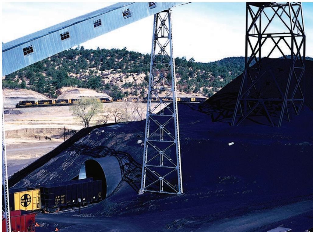
At the York Canyon Mine, to load the dedicated coal gondolas the train was pulled around a loop track that included a tunnel passing under the storage pile. The cars emerged from the tunnel — to the right of this image — fully loaded.
