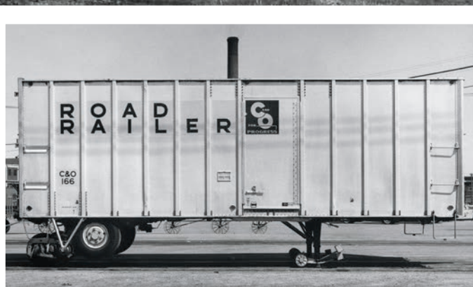
▲ The trailer-on-rail concept began with C&O's Railvan, 27-foot trailers designed to carry mail and express behind passenger trains. The prototypes debuted in 1959; trailers ran in Chicago-Detroit service into the late 1960s. Chesapeake & Ohio ► The trailers were renamed RoadRailers in 1961. John B. Corns
