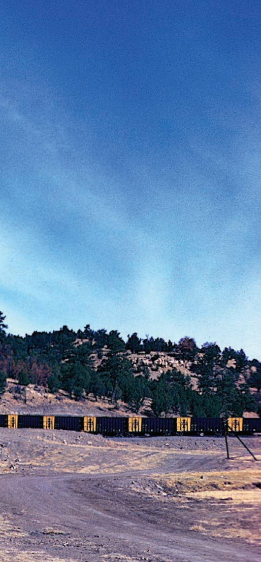
At the York Canyon Mine, to load the dedicated coal gondolas the train was pulled around a loop track that included a tunnel passing under the storage pile. The cars emerged from the tunnel — to the right of this image — fully loaded.
