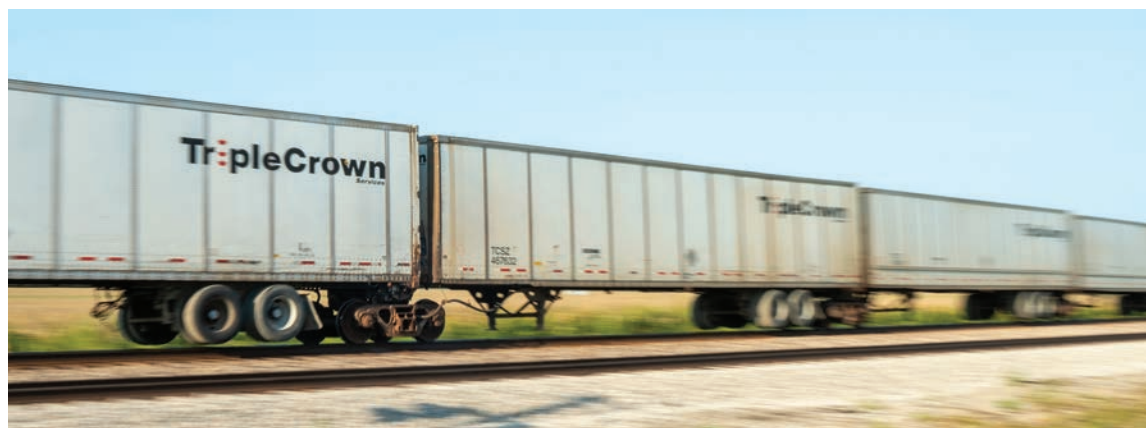
▲ A pan shot of the last run of train 255 highlights the final RoadRailer design, the Mark V that replaced the rail wheels on the trailer with standard rail bogies. Steve Smedley
