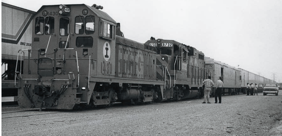
▲ An Illinois Central Gulf RoadRailer train is assembled at Johnston Yard in Memphis, Tenn., on April 1, 1982. Two company rebuilds are involved: SW14 No. 1430 is putting together the train; the road unit, No. 8732, is a GP11. The ICG operation made clear the shortcomings of the Mark IV trailers, which included their weight and the system that provided air for train brakes and to raise and lower wheels. Chuck Hinrichs
