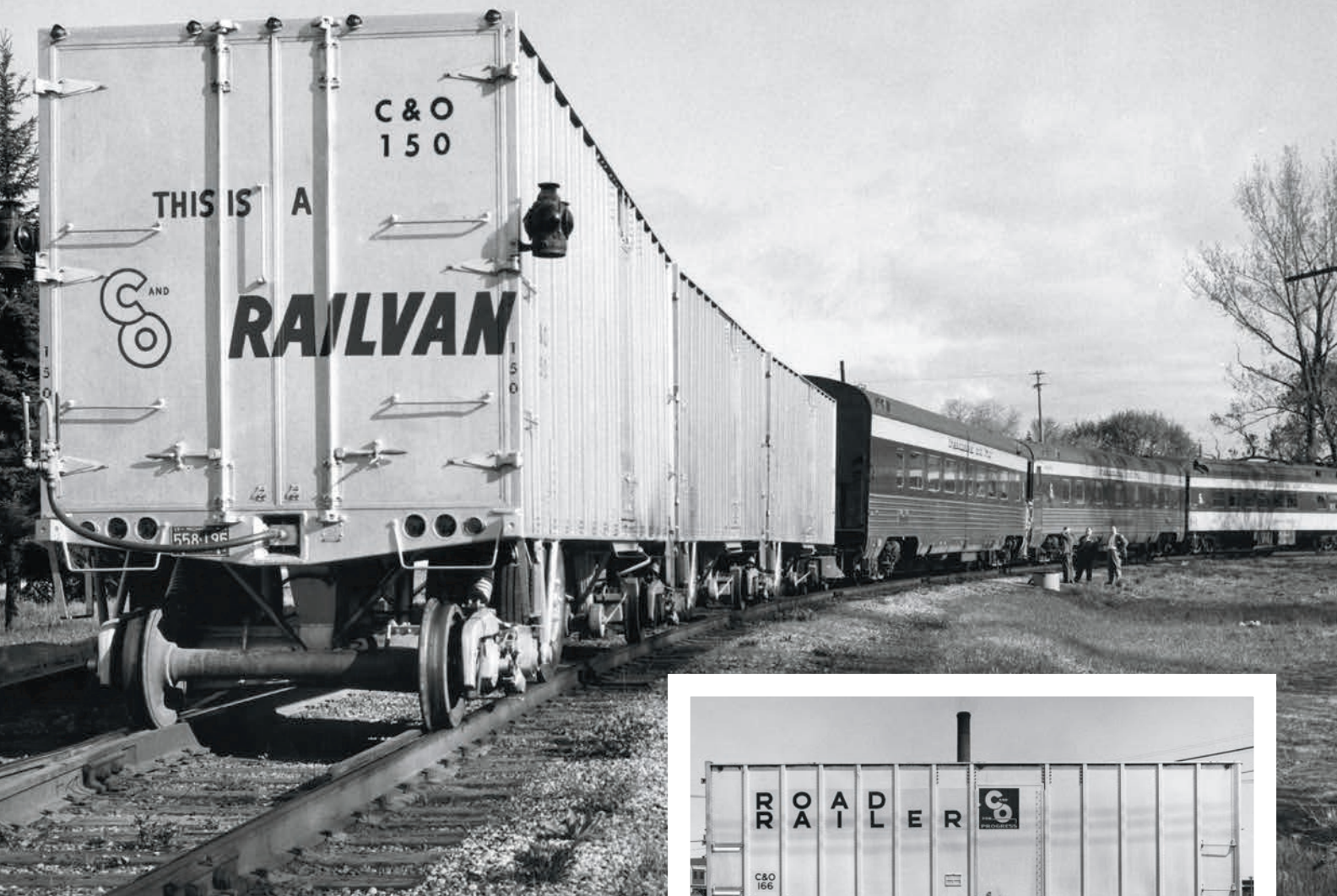
▲ The trailer-on-rail concept began with C&O's Railvan, 27-foot trailers designed to carry mail and express behind passenger trains. The prototypes debuted in 1959; trailers ran in Chicago-Detroit service into the late 1960s. Chesapeake & Ohio ► The trailers were renamed RoadRailers in 1961. John B. Corns
