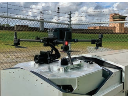
A drone awaits the call to perform a track inspection at Rice Yard. The autonomous devices can find defects without shutting down a track.
