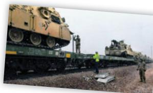
During loading and unloading, military and civilian railroad personnel work together as seen here at Fort Carson, Colo., during December 2016. The oversized dimensions of armored vehicles favor rail transport. Notice how the armored vehicle tracks lap over the side of the flatcar. Three photos, Bill Diven
