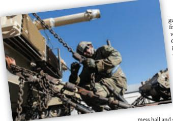
There is a method to tying a heavy armored vehicle to a flatcar for movement. The soldiers in mechanized units responsible for transportation are trained how to secure its vehicles aboard a train. Two photos, Bill Diven
