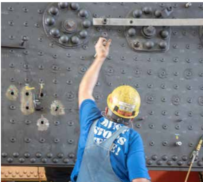
Steam shop worker Bruce Kirk checks a rigid staybolt on the engineer's side of the firebox. Such bolts allow the firebox to expand when hot. The other staybolt type is flexible and is often found on the roof.
