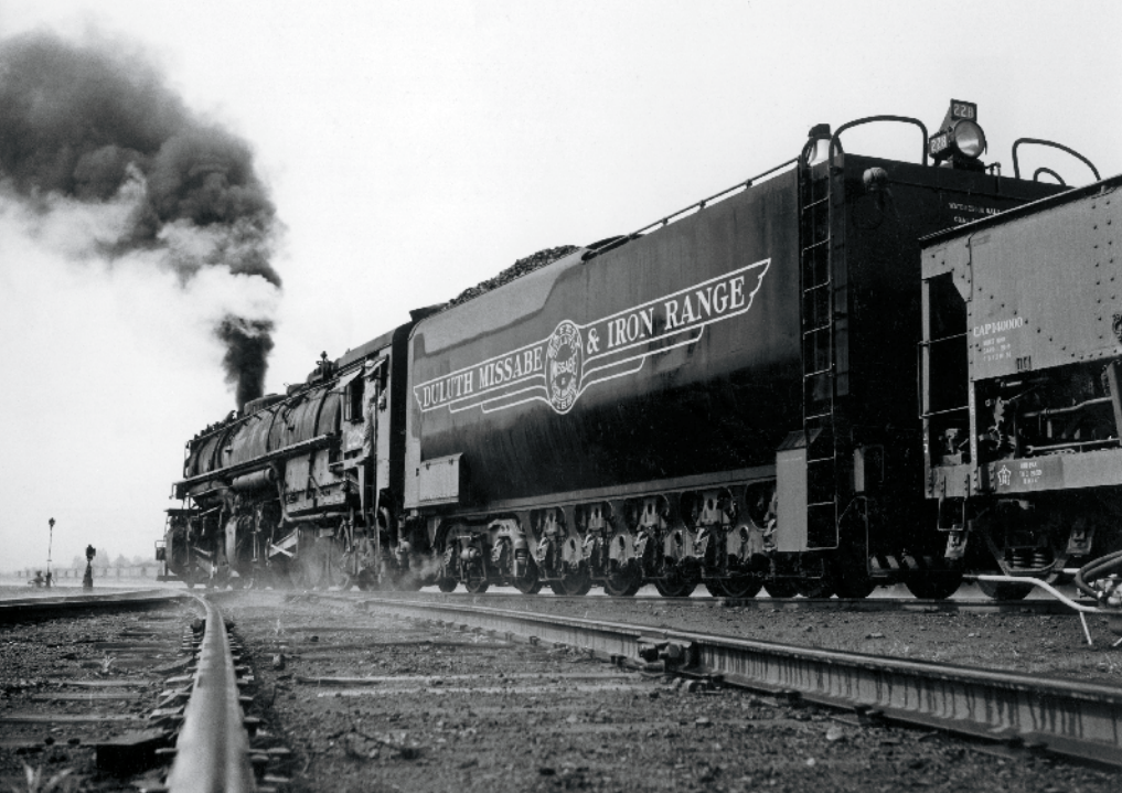
Duluth, Missabe & Iron Range M-3 class 2-8-8-4 No. 228 departs Proctor, Minn., westbound with 200 empty ore cars in August 1959 under a column of exhaust. William D. Middleton
