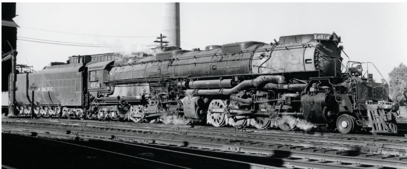
Long before it became a star, Big Boy No. 4014 was just the 15th engine of an initial order for 20 Union Pacific 4-8-8-4s completed in fall 1941 at Alco's plant in Schenectady, N.Y. On the eve of World War II, the engines were pressed into service. Emil Albrecht photo, James L. Ehernberger collection
