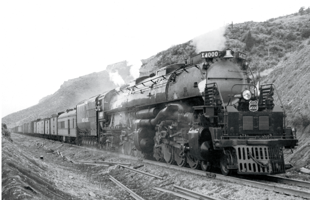
The first Big Boy, No. 4000, makes its first trip from Ogden, Utah, to Green River, Wyo., in 1941, flying white flags and with a car tucked in behind the tender to allow the mechanical department to monitor the 4-8-8-4's performance. E.C. Schmidt
