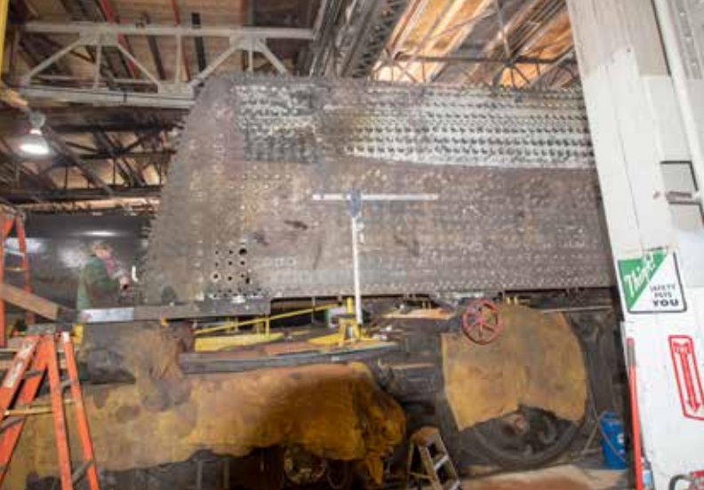
With the cab removed and the backhead exposed, work progresses on No. 4014's boiler in March 2017. Compare this image to the photos on page 42 showing the cab being installed in this area.
