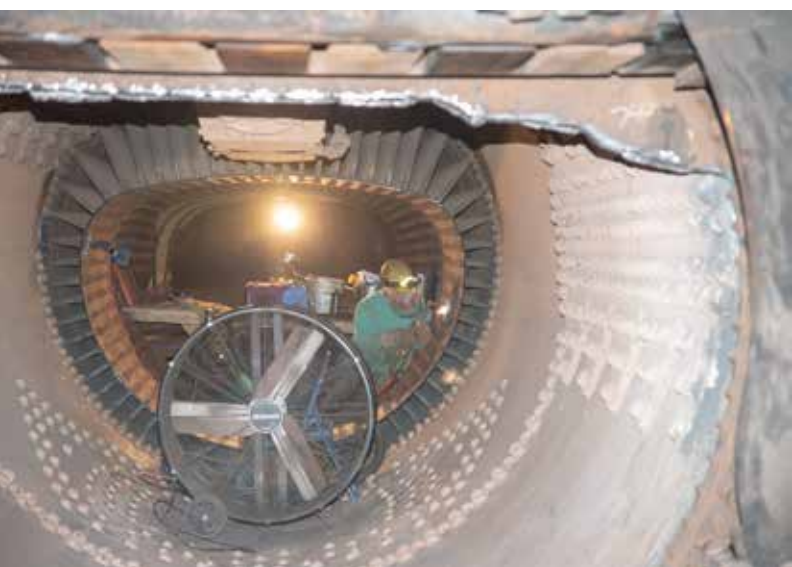
Looking down the barrel of the long boiler from the smokebox end, and with both front and rear tube sheets removed, boilermaker Jimmy Thompson uses a cutting torch to remove a staybolt.
