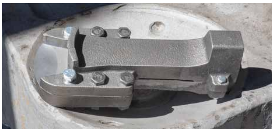
Above, UP steam shop manager Ed Dickens shows a rebuilt crosshead guide on a work bench. Note the many machines placed throughout the shop for easy access. Right: The biggest change in No. 4014 from its regular service career to restoration is the conversion from coal to oil firing. This is the burner for the oil firing apparatus. Fuel oil enters at right and is sprayed into the firebox as a mist that ignites in the air.
