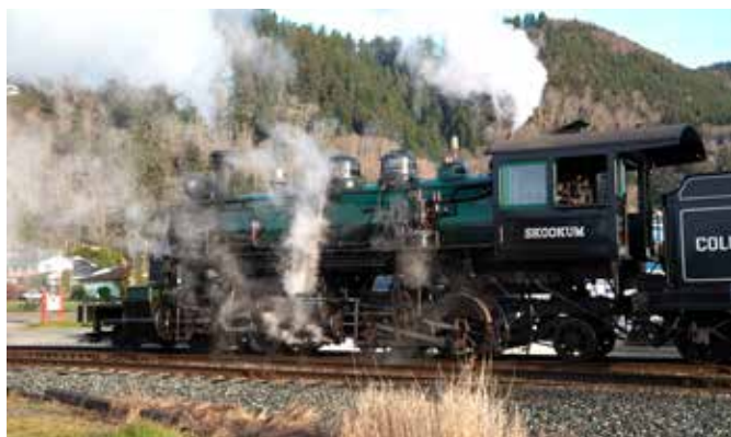
Skookum shows off its smaller high-pressure cylinders and its larger low-pressure cylinders at Garibaldi, Ore., in March 2019.
