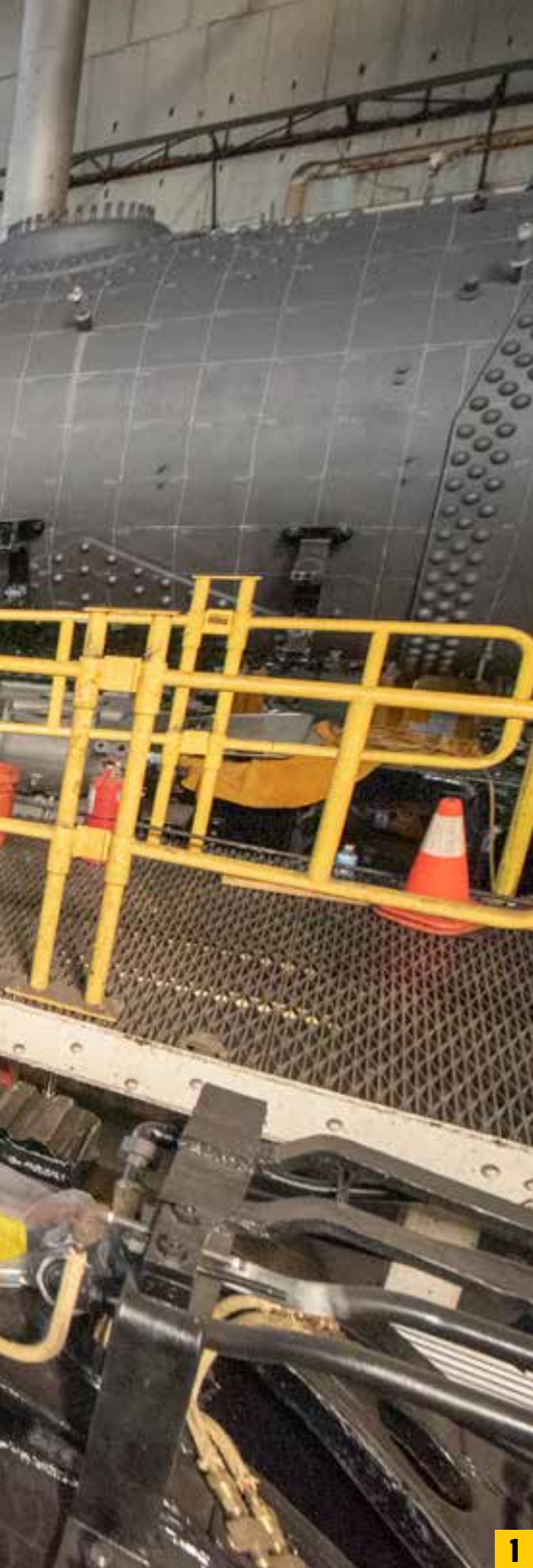
1 March 2018, and much of Big Boy No. 4014's front engine frame has been completed. Lubrication lines, inaccessible once the boiler is reattached, are wrapped in light-brown insulating covers. The boiler sits one track over to allow workers to make progress on both portions at the same time. The grid on the boiler is made in soapstone so that each section can be tested for integrity. Mechanical lubricators have green tops. The perspective is from near the second set of cylinders looking forward. 2 The restored backhead of the locomotive shows firedoor, studs for appliances, numerous staybolts. The backhead is jacketed and insulated before controls, water glasses, and other items are installed. 3 Staybolts by the box are placed in containers for transfer from the machine shop to the shop floor. 4 Garland Baker with the computer-controlled machine that cuts staybolt threads. The massive Big Boy may be a 1941 product that was state of the art for its time, but some of its parts were made with the most modern of machines.
