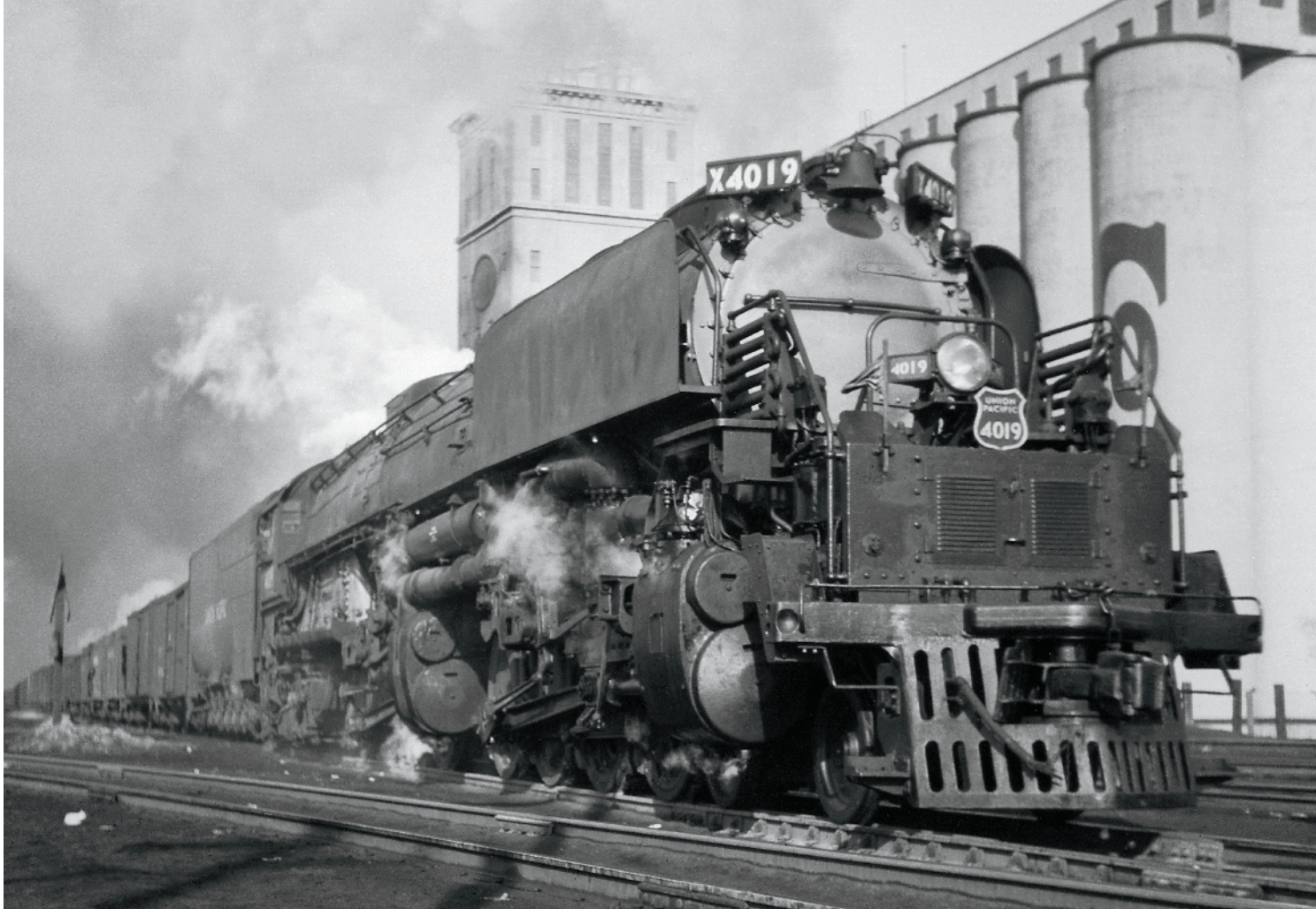
Union Pacific continued to look for ways to improve the Big Boys throughout the locomotives' lifespan. No. 4019, leaving Ogden on Jan. 19, 1946, sports "wind wings," or smoke deflectors. Emil Albrecht, James L. Ehernberger collection
