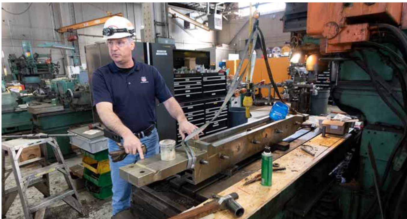
Above, UP steam shop manager Ed Dickens shows a rebuilt crosshead guide on a work bench. Note the many machines placed throughout the shop for easy access. Right: The biggest change in No. 4014 from its regular service career to restoration is the conversion from coal to oil firing. This is the burner for the oil firing apparatus. Fuel oil enters at right and is sprayed into the firebox as a mist that ignites in the air.
