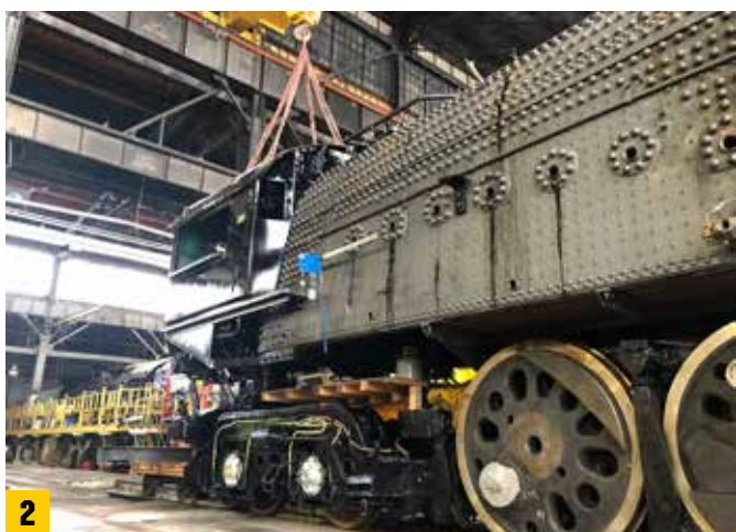
1 Cab installation. With boiler work completed, the boiler and frame reattached, the crew cab is placed on the finished backhead. 2 A new shop crane eases the rebuilt and painted cab into place in February 2019. The blue flag indicates presence of shop workers on or under the engine. The circular pattern of rivets reinforces areas for air to be admitted to the firebox to aid in combustion. 3 Once more, Big Boy looks more like its old self. Note the rebuilt trailing truck that is pictured on page 35. Light-colored piping carries lubrication lines. The UP steam shop crew praises the new overhead crane installed to aid in the Big Boy and all future projects. Four photos, Union Pacific
