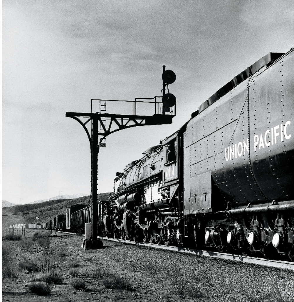
The Big Boy's seven-axle Centipede tenders held 24,000 gallons of water and 28 tons of coal. The tender with No. 4014, shown as it is taken to Pomona, Calif., for display, was originally delivered with locomotive No. 4015. Stan Kistler
