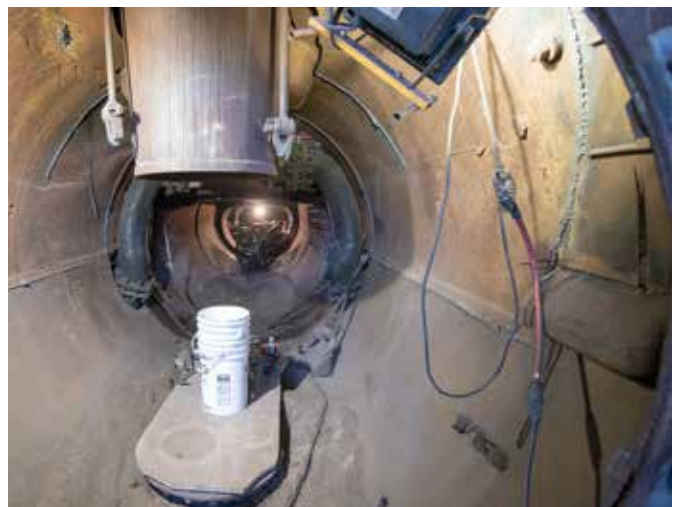
The smokebox interior shows fabricated design, smokestack, and live steam tubes running from the superheater header. Plastic buckets sit on a covering where the exhaust nozzles are normally found.
