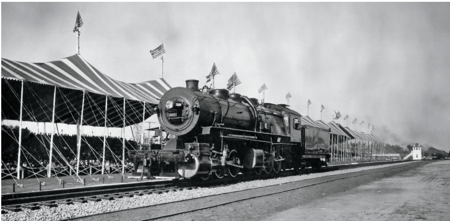
America's first Mallet, Baltimore & Ohio 0-6-6-0 No. 2400, rolls past the reviewing stand at the Fair of the Iron Horse near Baltimore in 1927 to celebrate the railroad's centennial. The locomotive, built in 1904, saw years of service on Pennsylvania's Sand Patch grade. Baltimore & Ohio
