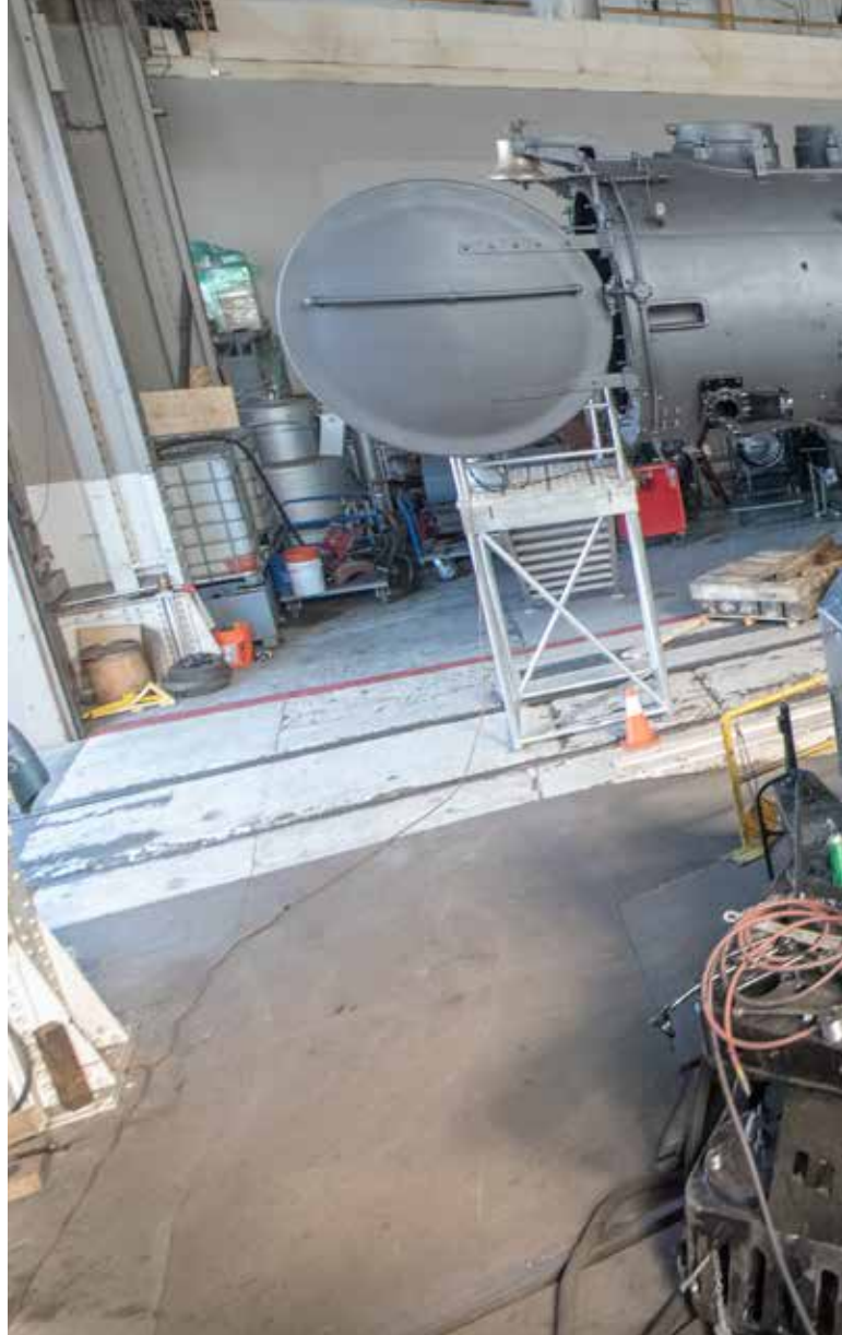
Above, in a scene unimaginable only a few years ago, No. 4014's boiler and front engine share space inside the Cheyenne backshop. New lubrication lines (light colored strands) have already been run on the engine.
