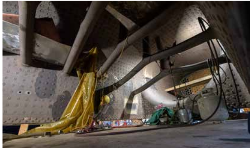
The Big Boy firebox, from the engineer's side looking forward toward the smokebox, shows multiple circulator tubes coming off the crown and sidesheets, staybolts, combustion chamber, and rear tube sheet.
