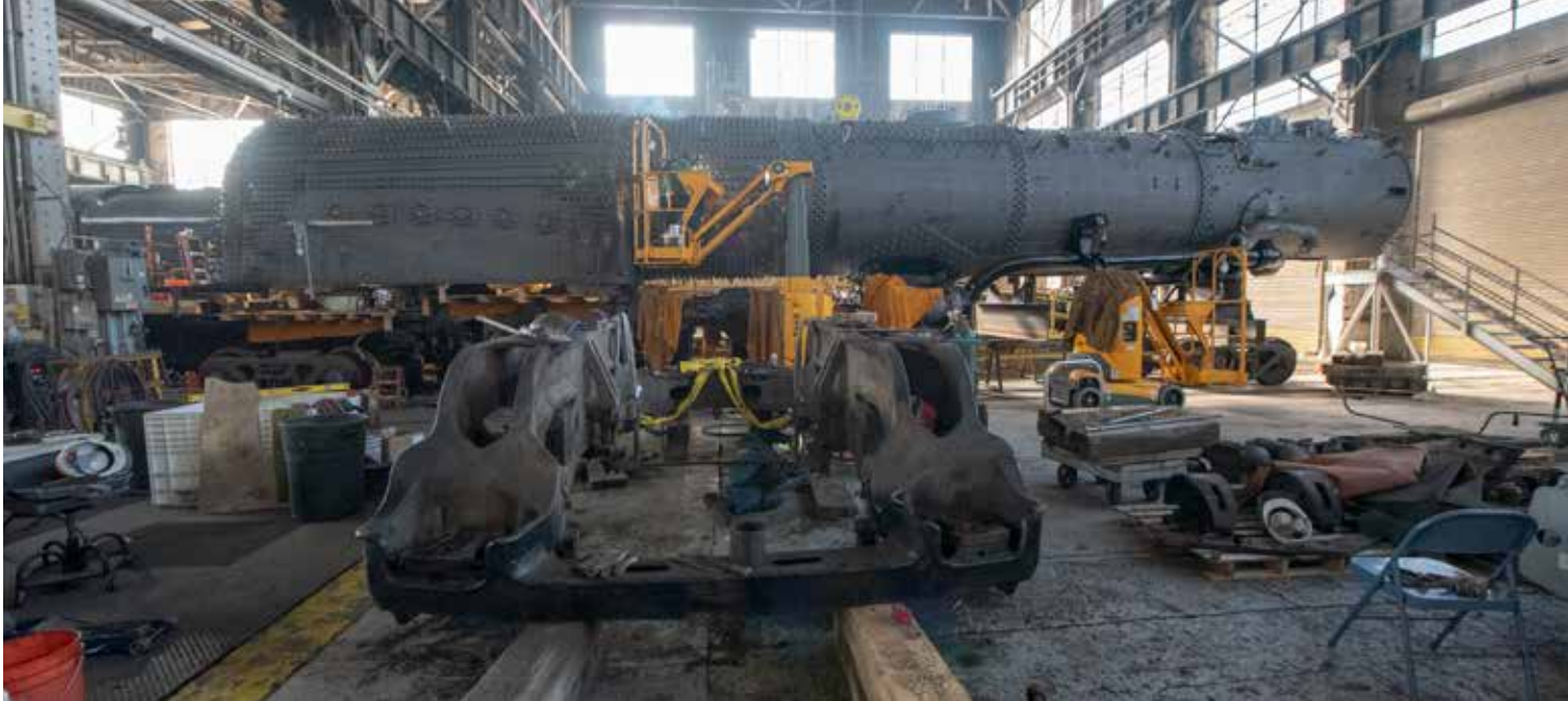
Left, we are looking across three sets of drivers in June 2018 that have just returned from quartering and installation of new tires at Pennsylvania's Strasburg Rail Road. In rear is the boiler backhead.
