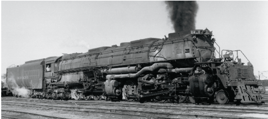
Twin pillars of smoke mark the double smokestacks that were adopted as standard for freight power. Hidden are the many changes inside the elongated smokebox that over the years were modified to improve drafting and reduce the chance for lineside fires. TRAINS collection
