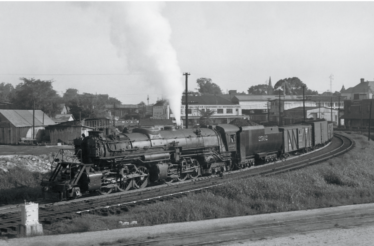
Seaboard Air Line 2-6-6-4 No. 2502 leads a freight at Raleigh, N.C., in 1941. Seaboard's 10 such locomotives predate Norfolk & Western's arguably more famous entries by a year. They operated in fast freight and passenger service north of Hamlet, N.C. TRAINS collection
