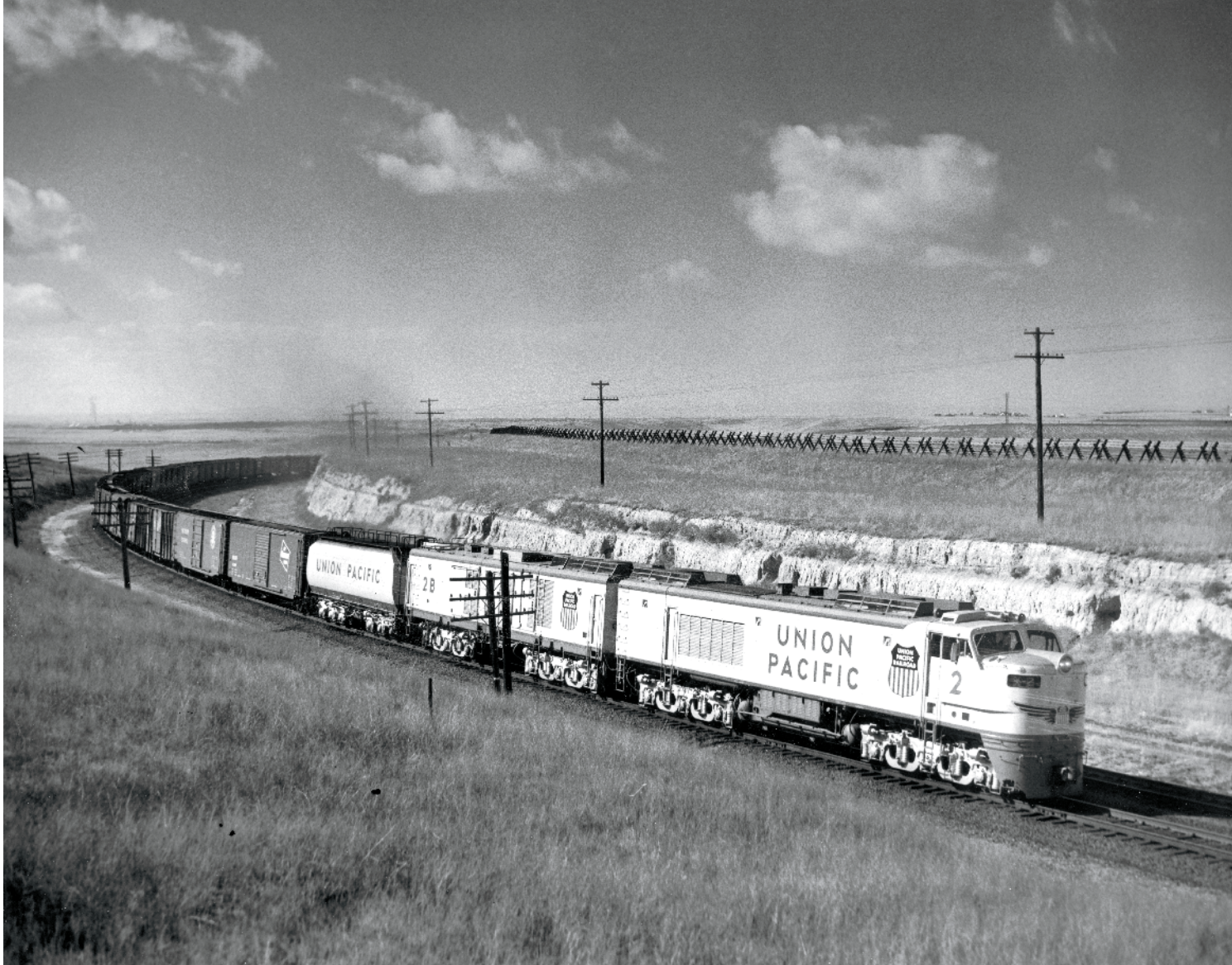
Gas-turbine-electric No. 2 hustles a freight east through Archer, Wyo., in October 1958. The 8,500-hp set was the newest such technology on the railroad at the time. Stan Kistler
