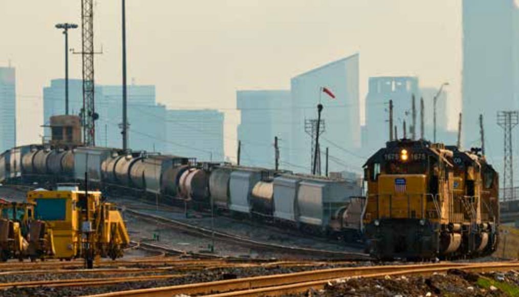
Cars are shoved over the hump at Houston's Englewood Yard. At a time when other railroads are eliminating humps, UP is building its 15th, Brazos Yard, in central Texas. Tom Kline
