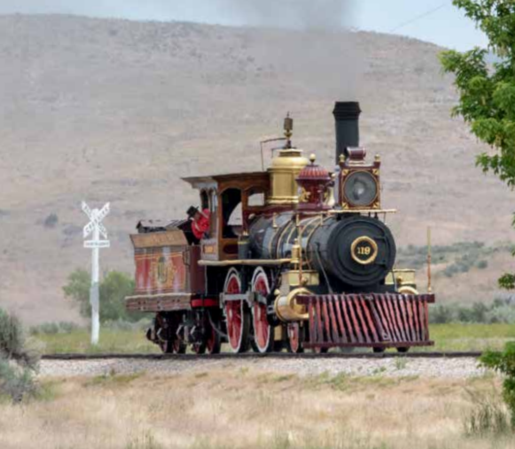
No. 119 makes a demonstration run at the Golden Spike National Historic Site. The coal-burning locomotive was built in California in the 1970s and placed into service in 1979.
