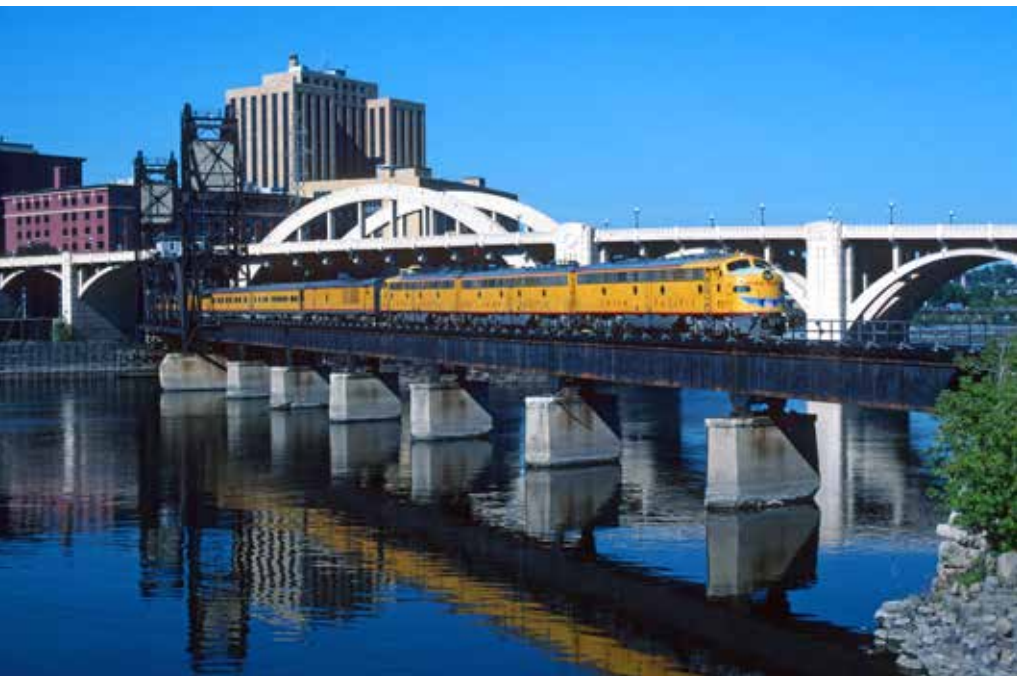
The executive Es, led by No. 951, cross the Mississippi River at St. Paul, Minn., in September 1999. The units have been repowered with EMD 645s, making them into streamlined GP38-2s.
