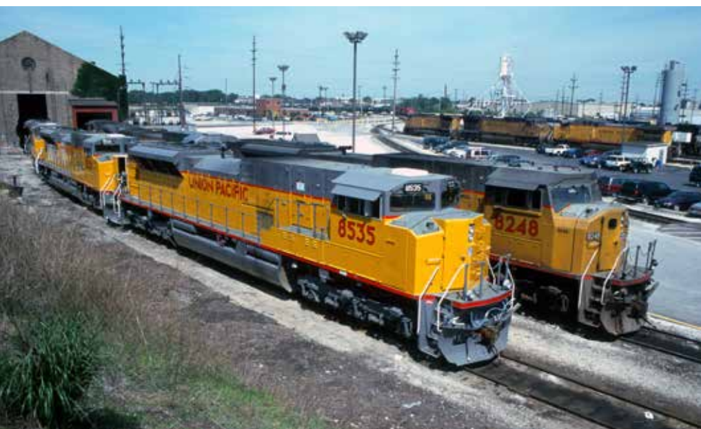
In June 2000, a trio of new 6,000-hp SD90MAC-Hs are parked next to a convertible SD9043MAC built two years earlier. No. 8248 is still on UP's roster today, renumbered to No. 3772.
