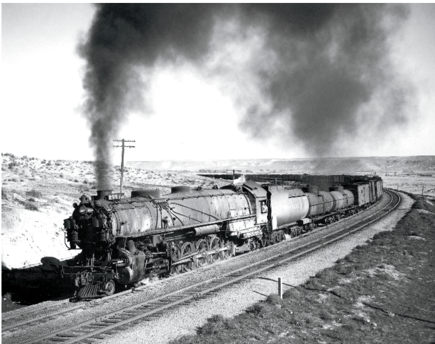
A 4-12-2, a wheel arrangement unique to the Union Pacific, starts up Medbury Hill just west of Hammett, Idaho, in October 1957. The freight train has 75 cars and two 2-8-2s pushing.
