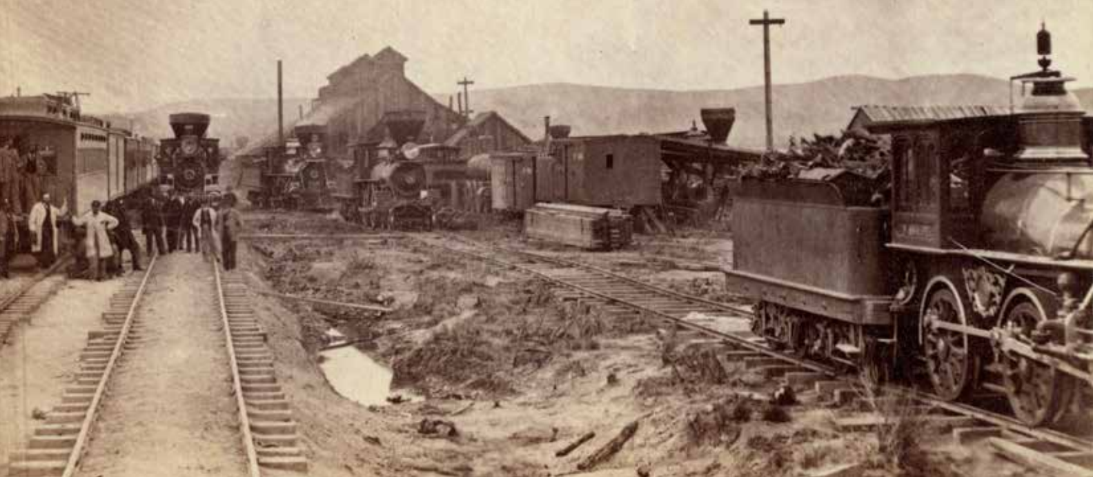
There are eight balloon stacks from early Central Pacific power, plus the engine to the right, as well as two boilers and cabs in this image. At left is Gov. Stanford's special. The location is the machine shop at Carlin, Nev. Alfred A. Hart, Department of Special Collections, Stanford Libraries collection
