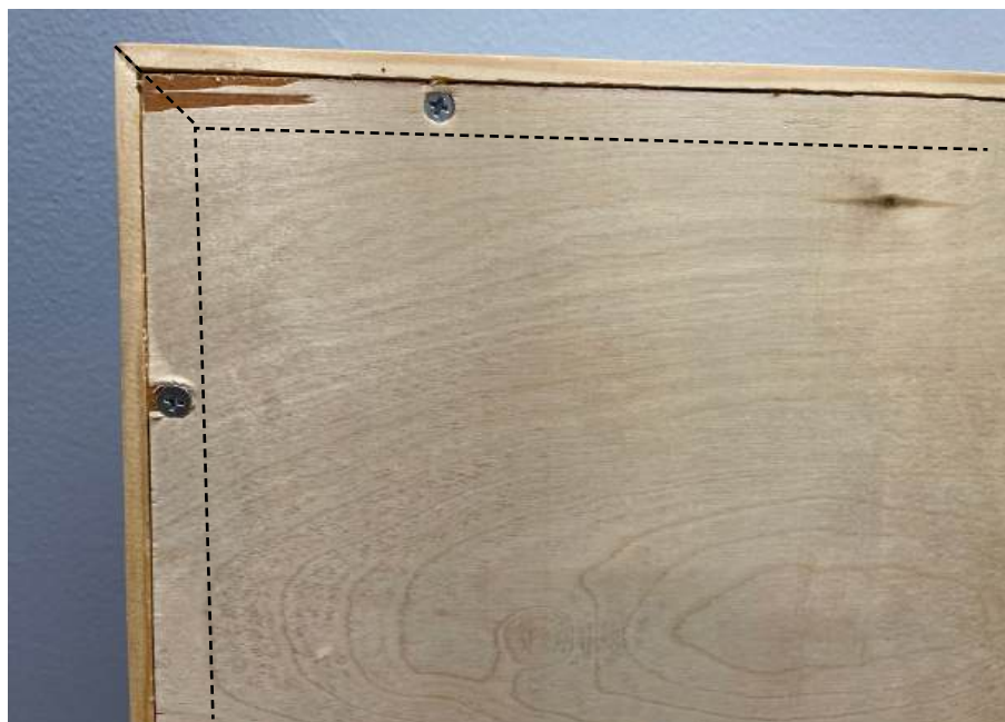
❶ The back of the case is shown with its mitered corner and rabbeted frame. The dashed lines indicate the edges of the frame pieces that are partially covered by the plywood back.
