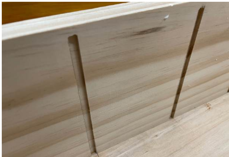
5 Dado grooves in the wood frame add extra horizontal support to the Plexiglas shelves. They're notched to fit inside the grooves.
