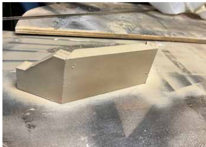
2 Next, Chris built bridge abutments from ¾"-thick plywood and secured everything using wood glue. Then he spray-painted the abutments with Rust-Oleum Camouflage Khaki.
