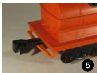
This model has a new coupler-support bar fabricated in three sections (the main bottom piece and the two small projections coming down to it). The repair was painted to match. This bar is .080" thick, whereas the original was .125" thick.
