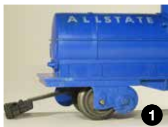
This Marx four-wheel plastic car has a broken coupler-support bar as well as a damaged truck side. It’s ready for repair!
