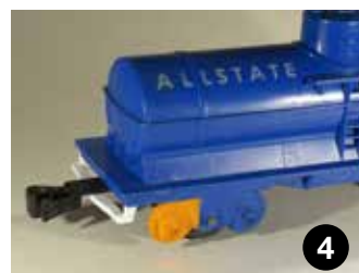
Then it was time to add a new coupler-support bar made from sheet styrene. He also glued in a section of simulated truck side.
