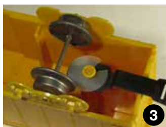
He next added a spacer on the coupler pin between the coupler and the head of the pin to hold the coupler higher.
