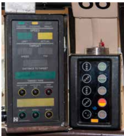
The XITCS display, at left, and UP cab signal display as they were installed in the cab of Amtrak P42 No. 66 during the Dwight-Pontiac 110-mph demonstration. Compare this with the current system shown at right.
