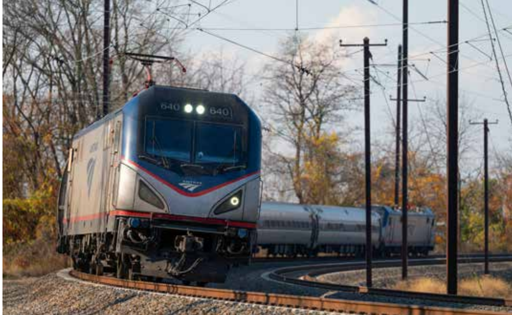
Keystone No. 666, led by Siemens ACS64 No. 640, sweeps through Gap, Pa. Keystones are usually push-pull sets with a cab control car at one end. This set has ACS64s at both ends.
