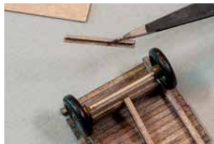
6 Two pieces of 3/32" angle stock enclose the axle.
