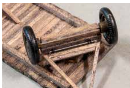
8 A wire link between the front axle and the drawbar lets it pivot two ways.
