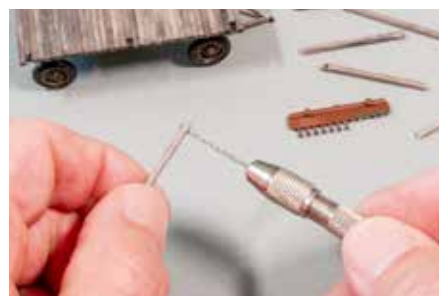
9 Lou drilled holes in the vertical posts for nut-bolt-washer castings.
