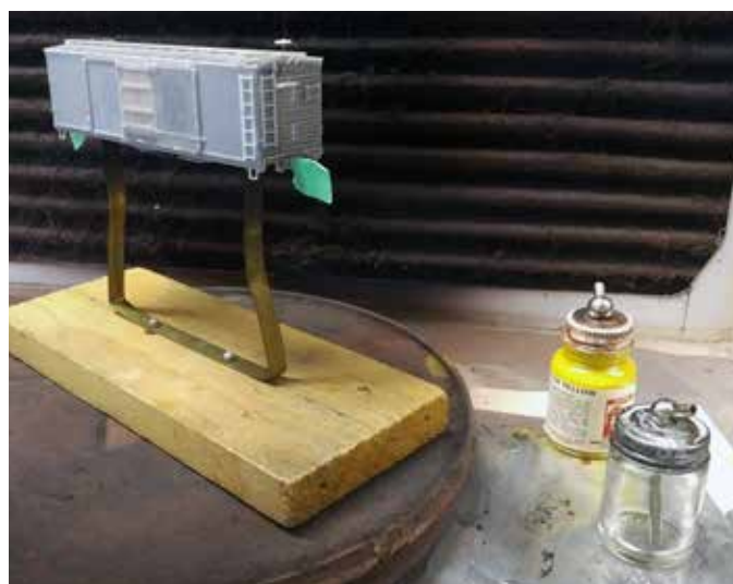
② A simple solution. David used punched steel strapping, a wood block, and screws to make this painting jig for his resin freight cars. The green masking tape is covering the couplers.
