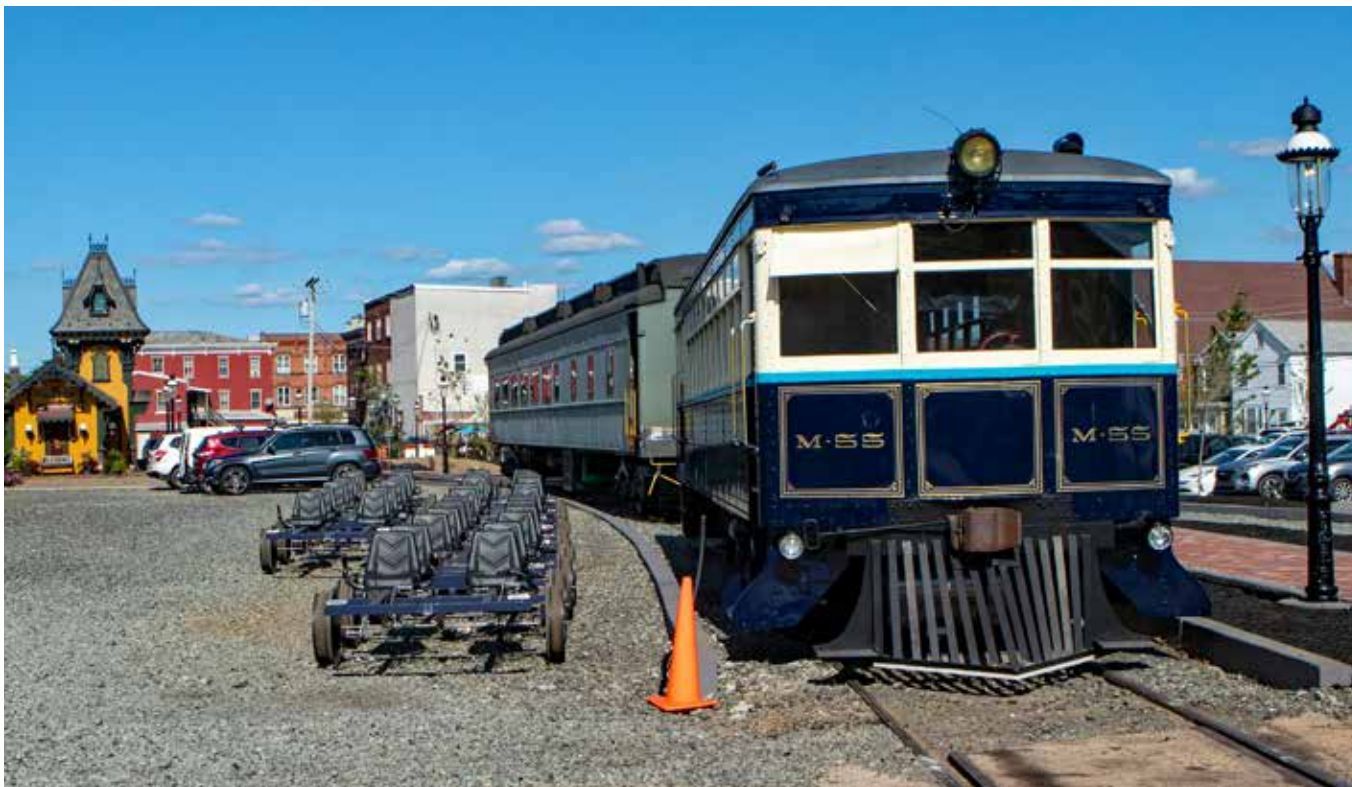
Showing its new Colebrookdale paint scheme, Doodlebug M-55 is at the railroad's Boyertown yard on Sept. 6, 2021. Built by J.G. Brill in 1930, the car's 34-passenger capacity is ideal for smaller parties. The motorcar is also occasionally used for rail bike events as the conveyance that returns riders to Boyertown. The rail bikes can be seen next to the M-55.
