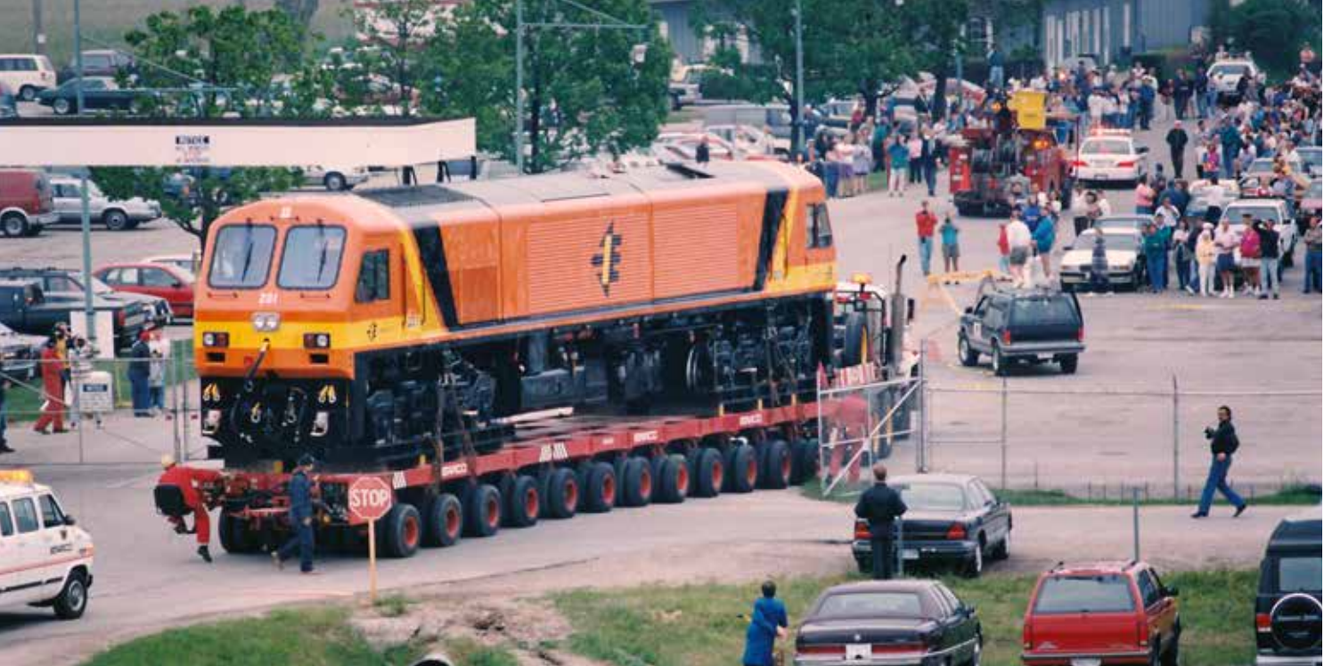
To transport Irish Rail's locomotive No. 201 from the Diesel Division General Motors Canada Limited plant to the London, Ontario airport, No. 201 moved on a special truck trailer with rails on it set at the Irish Rail track gauge of 5 feet 3 inches. Diesel Division General Motors Canada Limited
