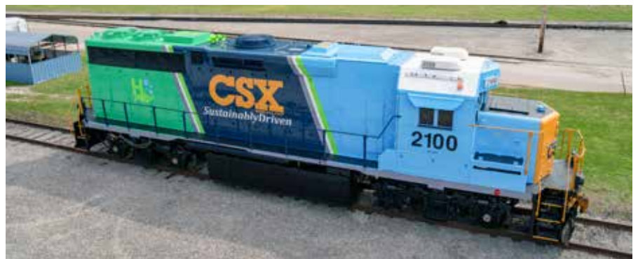
CSX GP38H2 No. 2100 was converted at the railroad's Huntington Shop from a diesel built for Baltimore & Ohio in 1972, using a kit provided by CPKC. CSX
