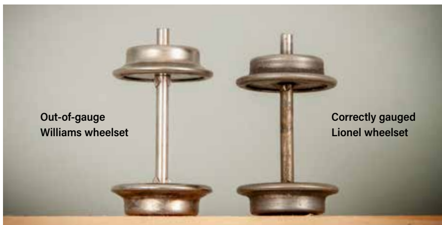
Figure 2. When placed side by side with a Lionel wheelset from the 1930s, the Williams axle (left) appeared to be forcing the wheels too far apart for them to roll easily on modern T-shaped rails.
