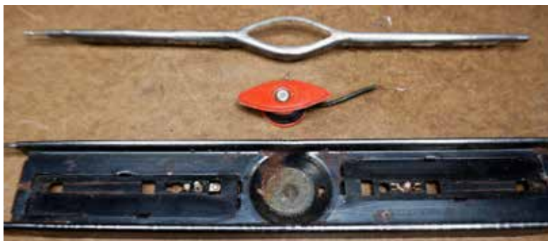
Fig. 1. A vintage Lionel Uncoupling Track David picked up at a local train show provides an electromagnet for this project. It didn't take him long to remove the red magnet from the track.
