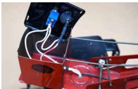
Fig. 3. Here you can see the type of thin and flexible wire David used and how he ran it through the end of the boom on the crane and then through the grommet hole where the crane rotates.
