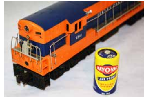
The Lionel No. 2341 Jersey Central Train Master was one of several diesels from the 1950s that used a battery to power its horn. Designers preferred the small batteries rather than track power for reasons explained here. Photo courtesy Peter Campo
