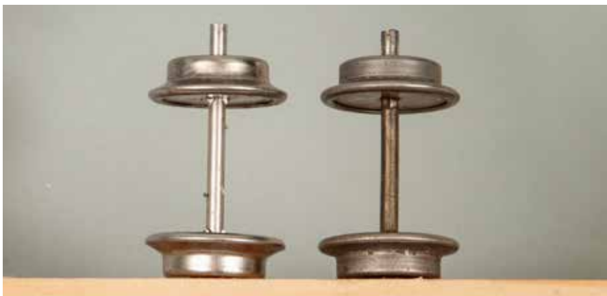
Figure 4. Once the width between the wheel stops on the Williams axle (left) had been modified to match the original Lionel axle on the right, the author felt confident they would operate smoothly and properly on any brand of O gauge track.
