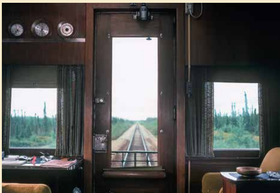
The dials above the window at left show the air brake pressure, the time, and the train's speed. The view out the back is typical of the Meander River Subdivision near the 60th parallel.
