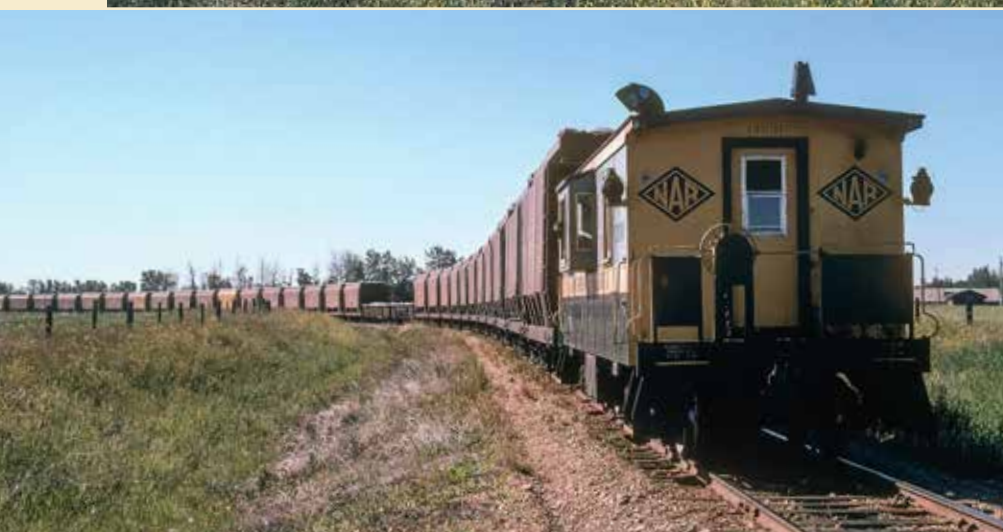
Turning the camera, one sees some of the CN's newer 100-ton center-dump ore cars, brought down from Pine Point Mine by the GSLR's triweekly train.
