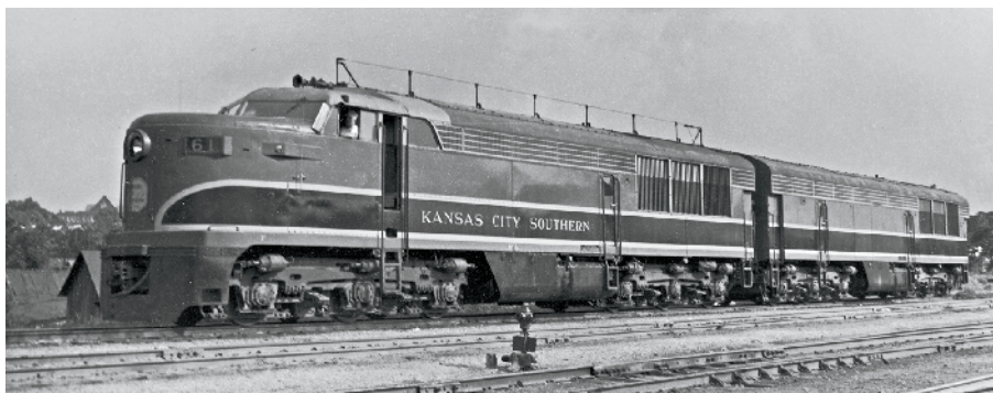
Kansas City Southern was one of seven buyers of 2,000 hp Fairbanks-Morse "Erie-built" units. The units derived their name from their assembly at General Electric's facility in Erie, Pa., when FM didn't have capacity at its Beloit, Wis., plant. A three-year-old cab-booster set rests at Shreveport, La., in July 1949. Harold K. Vollrath
