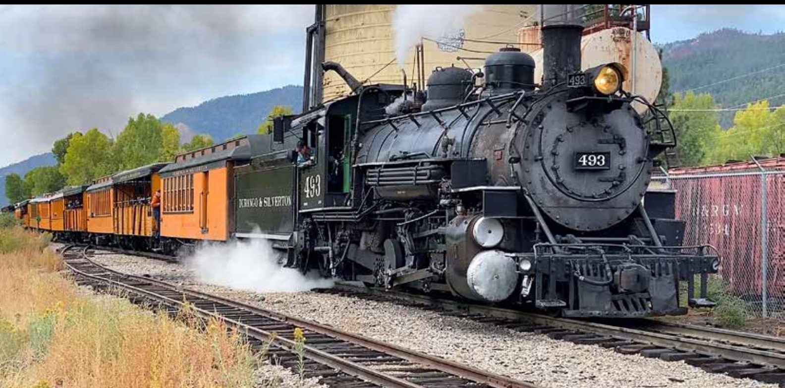
No. 493, passing Hermosa, was at one time thought to be junk and not worth rebuilding. By replacing rigid stay bolts with “flexies,” a number of deficiencies were corrected. The K37 is rated for three more cars than the K36s. Two photos, Lawrence Biemiller
