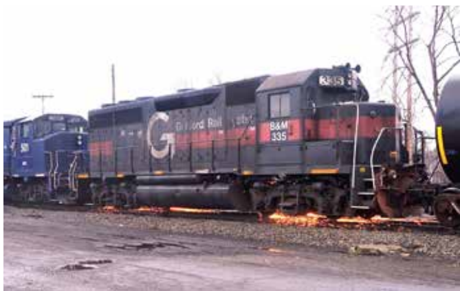
▲ WHEEL CREEP A Pan Am Railway GP40 loses its footing at a higher speed, causing a shower of sparks. The slippage could damage the traction motors, wheel, or the rail. One way to decrease wheel creep is with high-adhesion trucks. Union Pacific No. 5355, a General Electric ES44AC, rides on Hi-Ad trucks introduced with the Dash 9 series in the early 1990s. Left, Robert A. Stein; right, Jeff Wilson
