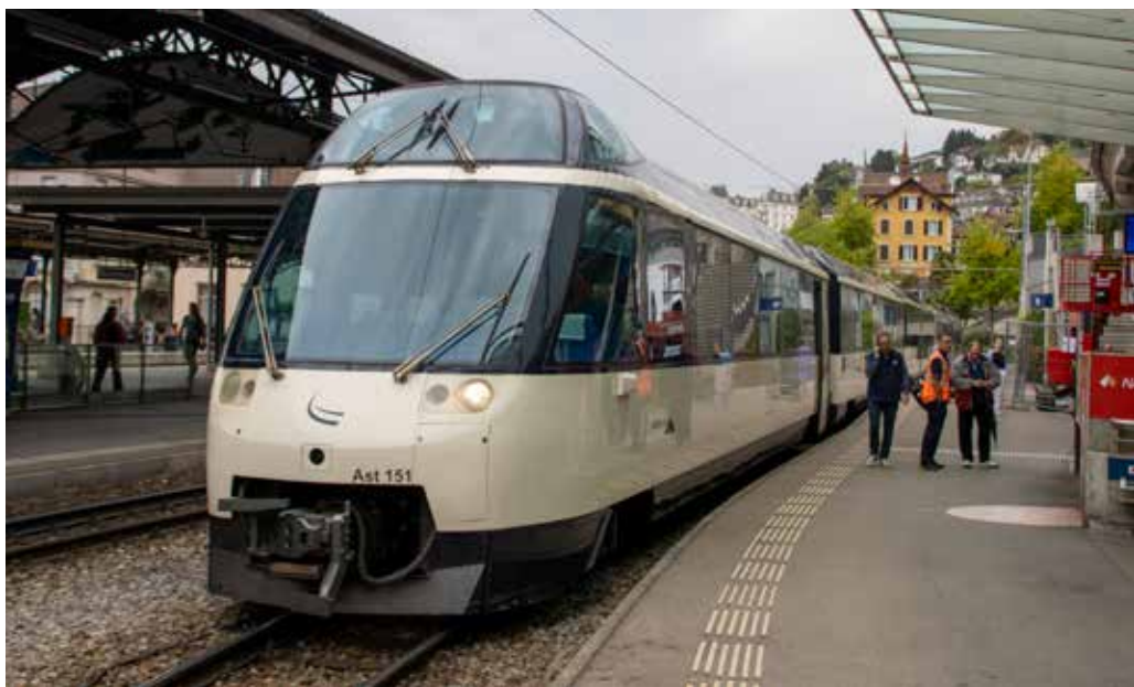
One of MOB’s Panoramic trainsets, which provide a driver’s view in the front row by moving the actual driver above the seating area.
