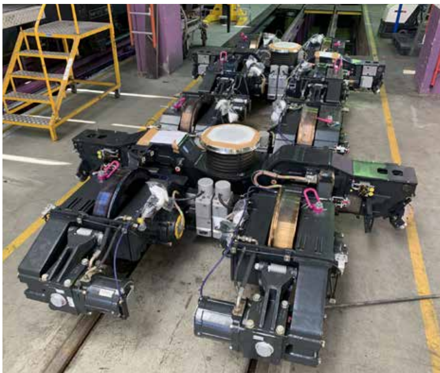
One of the complex wheelsets for a GoldenPass Express car. The key to the technology is that the frame expands; wheels are on stub axles rather than two to an axle. MOB-GoldenPass
