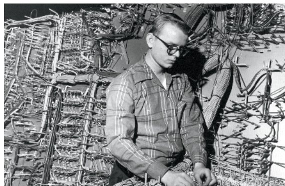
▲ EXANE WIRING There are miles of wire inside a diesel locomotive. Being better suited to the locomotive environment, Exane wire extended running life to more than 50 years.
