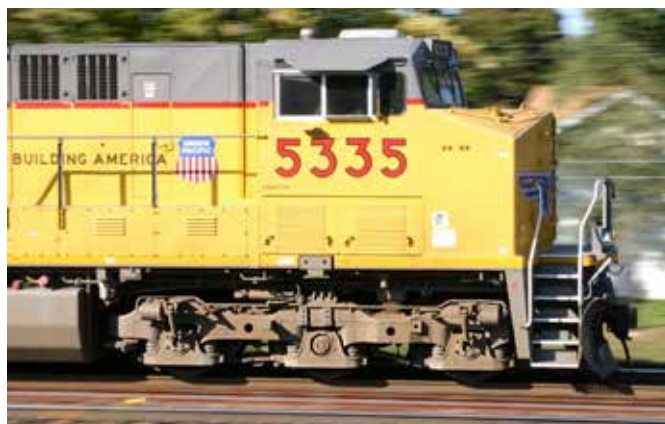
▲ WHEEL CREEP A Pan Am Railway GP40 loses its footing at a higher speed, causing a shower of sparks. The slippage could damage the traction motors, wheel, or the rail. One way to decrease wheel creep is with high-adhesion trucks. Union Pacific No. 5355, a General Electric ES44AC, rides on Hi-Ad trucks introduced with the Dash 9 series in the early 1990s. Left, Robert A. Stein; right, Jeff Wilson
