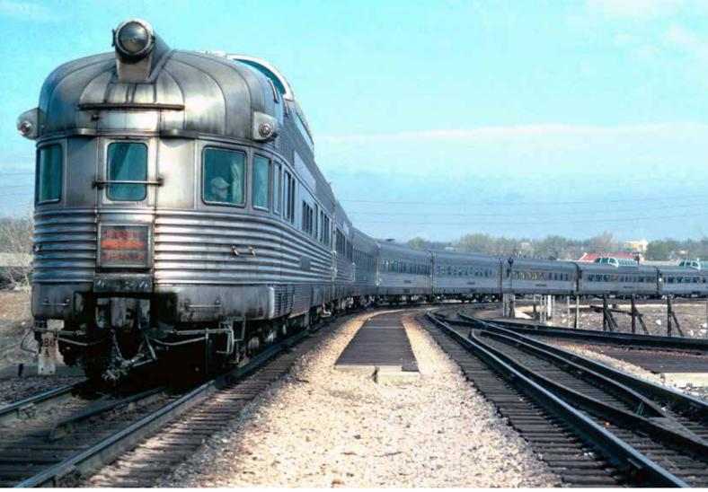
After the westbound California Zephyr arrived in Denver on the Chicago, Burlington & Quincy, its E units were cut off and a switcher dragged the train through the wash rack, then backed it into Union Station yard. A switchman maintains a look-out from the observation car. Steve Patterson
