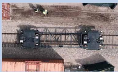
An overhead view of the Parallel Systems intermodal car makes clear its lightweight framework, as well as its lack of couplers. Cars are powered by battery-powered traction motors on each truck.
