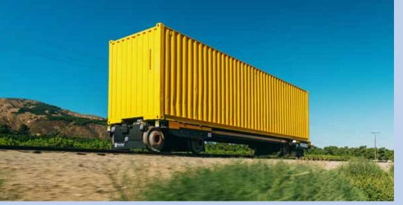
Parallel's second-generation prototype car can carry a container 500 miles on a single battery charge. It is designed to assemble into platoons of 10 to 50 cars, but has bumpers, not couplers. Four photos, Parallel Systems
