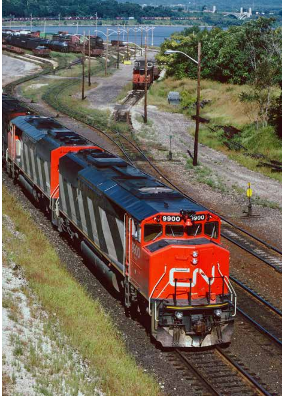
CN 9900 and 9901, designated SD50AF, were two of four SD60s built 3½ years prior to the first production units for CN. A print of this photo hung briefly in GMDD's corporate offices until it strangely disappeared over the 1988 Christmas shutdown.
