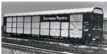
In later years, railroads including the Southern Pacific would switch to fully enclosed auto racks to deter vandalism. Portec Inc.
