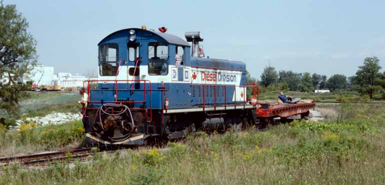
The GMDD switcher was this SW8 with no roster number. It emerges from the plant with an empty flatcar to be returned to CP's nearby Crumlin siding. Essential parts from EMD at LaGrange, Ill., were shipped by rail and interchanged to CP in London.
