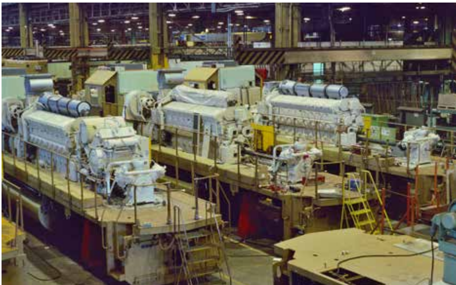
Three Cotton Belt GP60s have their prime movers affixed and await various additions such as water and lube oil reservoir assemblies. Three-cylinder, two-stage compressors are in evidence at the rear of the units, which are connected directly to a driveshaft.
