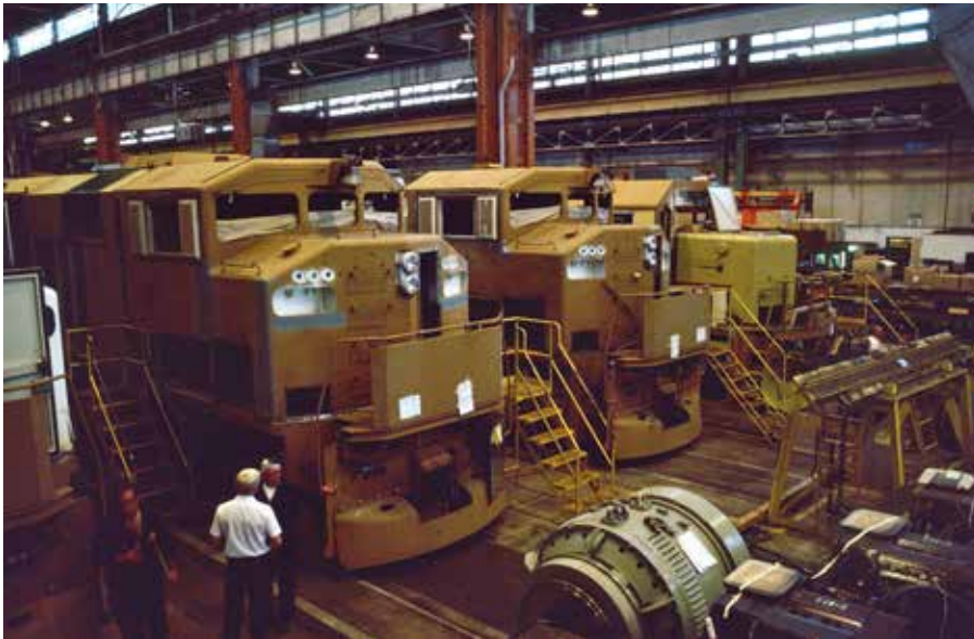
There's a lot to see as a design engineer confers with one of GMDD's shop floor workers. Multiple GO units, the nearest in some degree of paint, sit near the exit doors at the north end of the plant. Three traction motors and an alternator assembly are to the right foreground.
