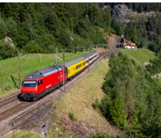
A train with a track geometry car (yellow coach) makes its way through Wassen.
