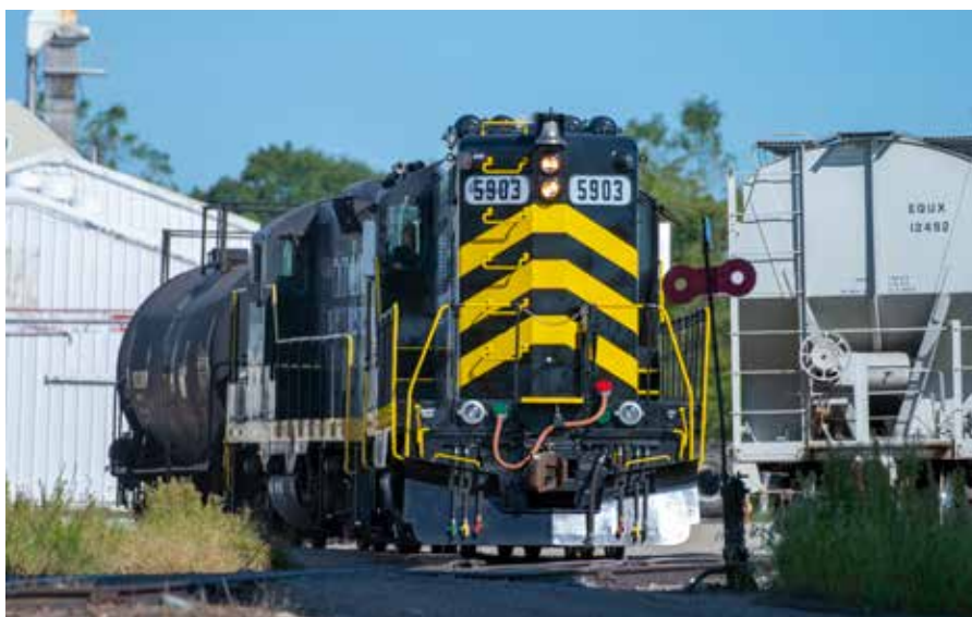
Engineer Jeffrey James spots liquid fertilizer loads at Ceres Solutions near the end of the line in Coldwater, Mich. on Sept. 19, 2019. GP9 No. 5903 was built for the Cleveland Union Terminal Railroad in April 1954. It was rebuilt by the Indiana Northeastern shop forces in Hudson, Ind., with a GP9H designation. The "H" stands for Hudson shops.
