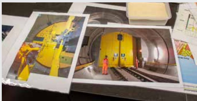
Among displays at Amsteg were these photos of the airtight door damaged by the derailment (at right) and the temporary door, normally for maintenance, that allowed some operation to resume.
