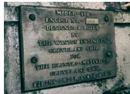
The builder’s plate attached to Montana Western No. 31’s engine indicates it’s a Winton model 106 — a “straight-six” power plant.
