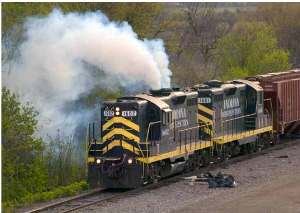
The railroad's two elderly statesmen at the time, ex-Reading Co. GP7s Nos. 1602 and 1601, clear carbon buildups as the crew goes to work on April 16, 2012. The two locomotives worked on the Hillsdale County Railway during the 1976 startup. No. 1601 was rebuilt by the Hudson (Ind.) shop. No. 1602, the first to wear this number on the INR, was retired and is now a parts source.
