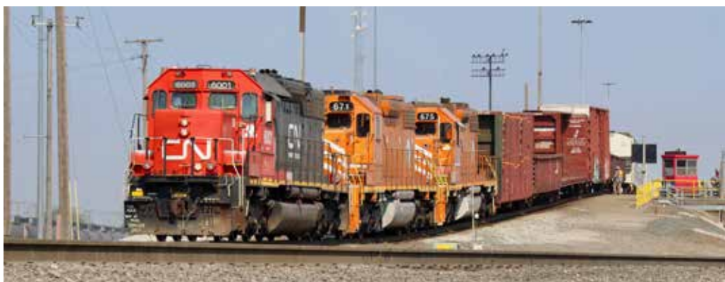
A three-unit hump set has nearly completed shoving a Western Canadian merchandise train over the Kirk Yard hump in Gary, Ind., on May 24, 2023. The pair of EJ&E SD38-3s were among the 38 locomotives CN acquired along with the railroad in 2009.
