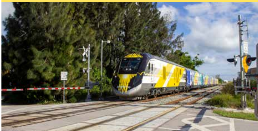
Quad gates have been installed at Shimonek Lane and every crossing without a roadway median. When the approaching train — wrapped with advertising promoting the start of Orlando service — triggers the quad gates, the exit gates are the last to lower.
