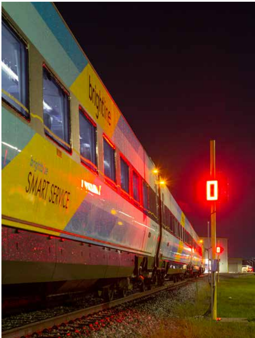
On the first day of revenue service, a BrightGreen trainset is still dripping from its trip through the washer at the “Basecamp” servicing facility in Orlando. The “0” indicator tells the engineer to stop while the nose of the rear locomotive is washed by rolling brushes.
