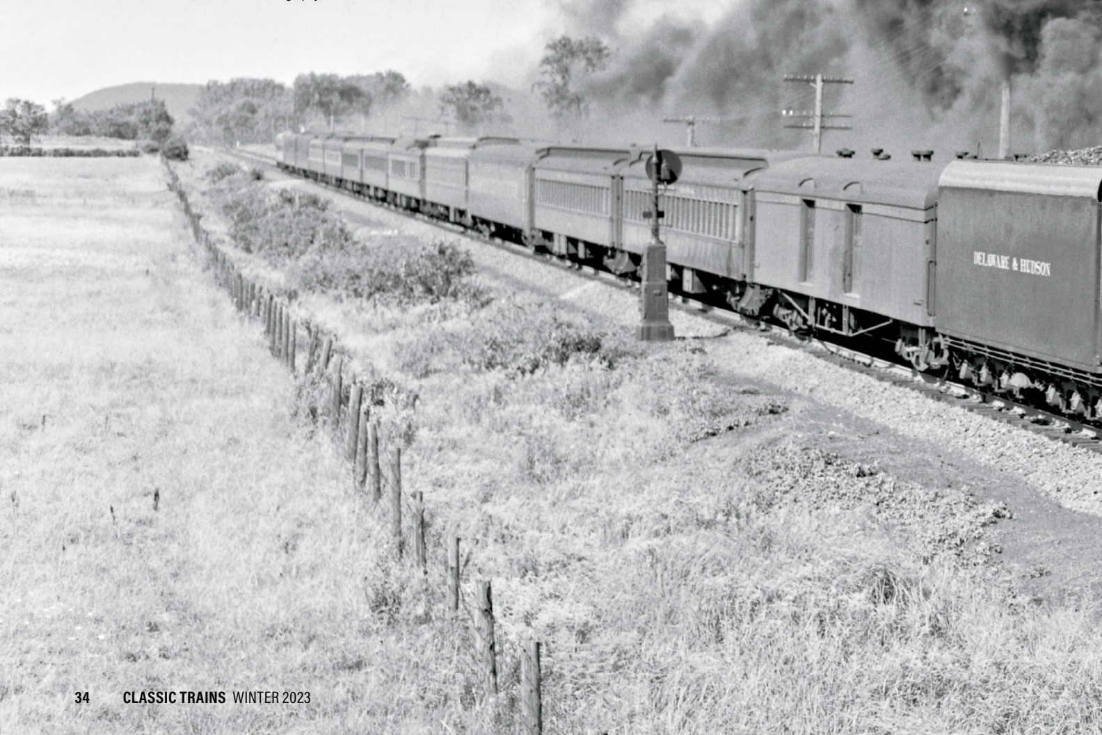
K class 4-8-4 No. 302 handles Train 34 with 13 cars south of Whitehall, N.Y., on Aug. 17, 1952. The "elephant ear" smoke lifters appear to be doing their job here.
