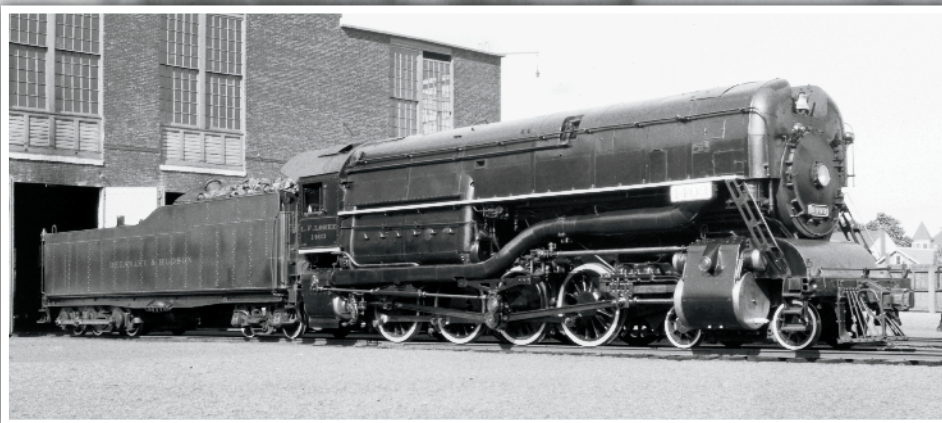
Experimental E-7 class 4-8-0 No. 1403 L. F. Loree , named for the D&H's president at the time, poses at Colonie Shops in 1935. Loree worked to push the 2-8-0 type to its maximum when other roads sought newer designs. Donald W. Furler, Center for Railroad Photography & Art collection
