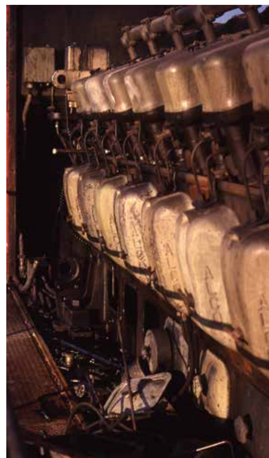
Removal of the engine hood of CP M636 4724 affords easy access for mechanics to remove salvageable parts from the forever stilled 16-cylinder 251 engine.
