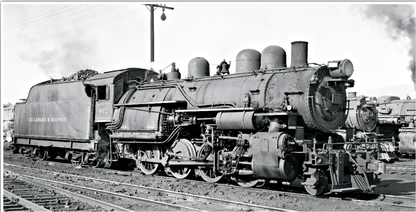
Anthracite coal piled high in its tender, 2-8-0 No. 912 displays its wide firebox at Carbondale, Pa., on Sept. 15, 1951. Donald W. Furler, Center for Railroad Photography & Art collection
