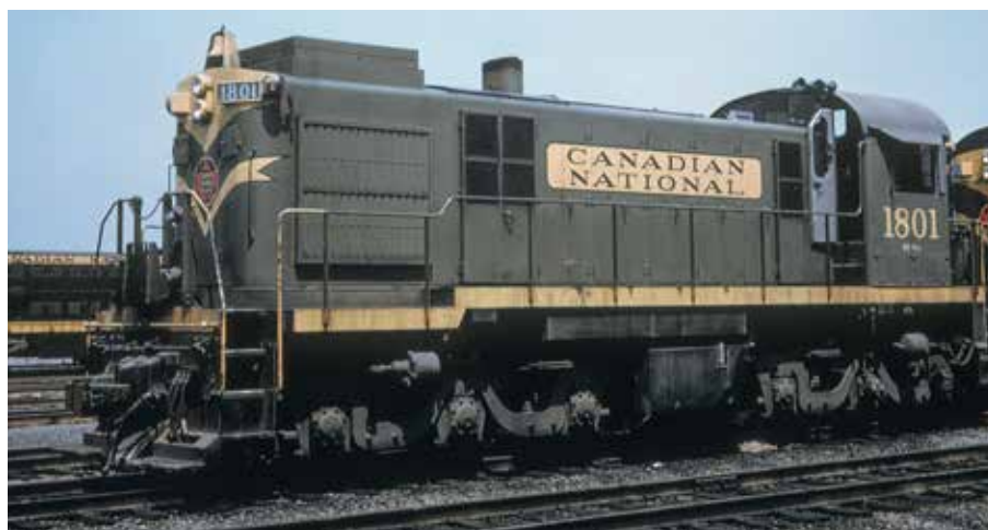
The diminutive RSC24 diesel locomotives look like a switcher, but with a stubby nose.
