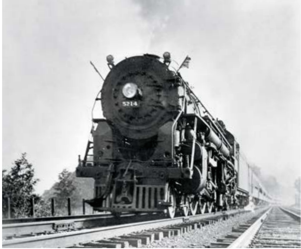
The 20th Century Limited, NYC's all-Pullman flagship between New York and Chicago, ran with 4-6-4s after 1927. Green flags on Hudson 5214 indicate a following section — not uncommon for the Century.
