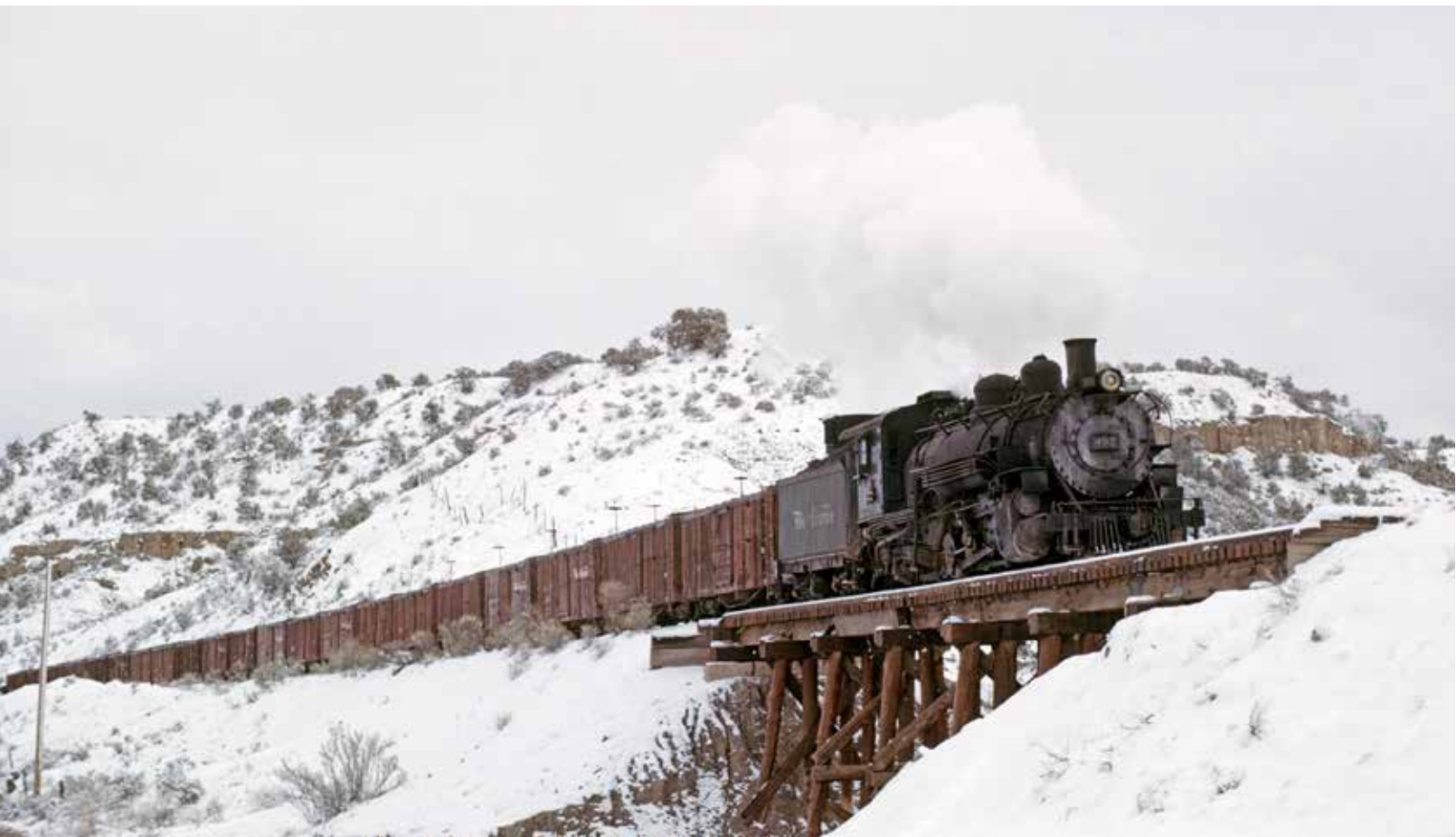
Fresh snow is abundant on the north end of the Farmington Branch as No. 492 heads south with its consist. The 490-series K-37s, heaviest engines on D&RGW's narrow-gauge lines, were rebuilt from standard-gauge 2-8-0s in the 1920s.
