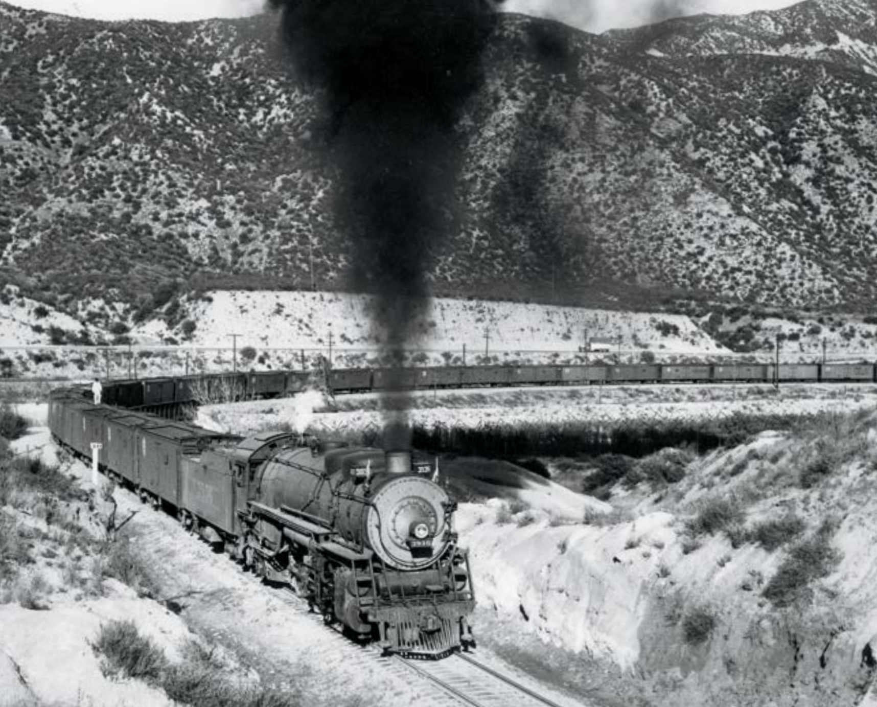
Santa Fe Railway No. 3936, one of 140 heavy 2-10-2s the road received from Baldwin between 1919 and '27, tramps up Cajon Pass with California oranges. This scene is from the 1940s, but the hardware — a plodding freight hog hauling ice-cooled reefers — would be familiar to railroaders of the Standard Era.
