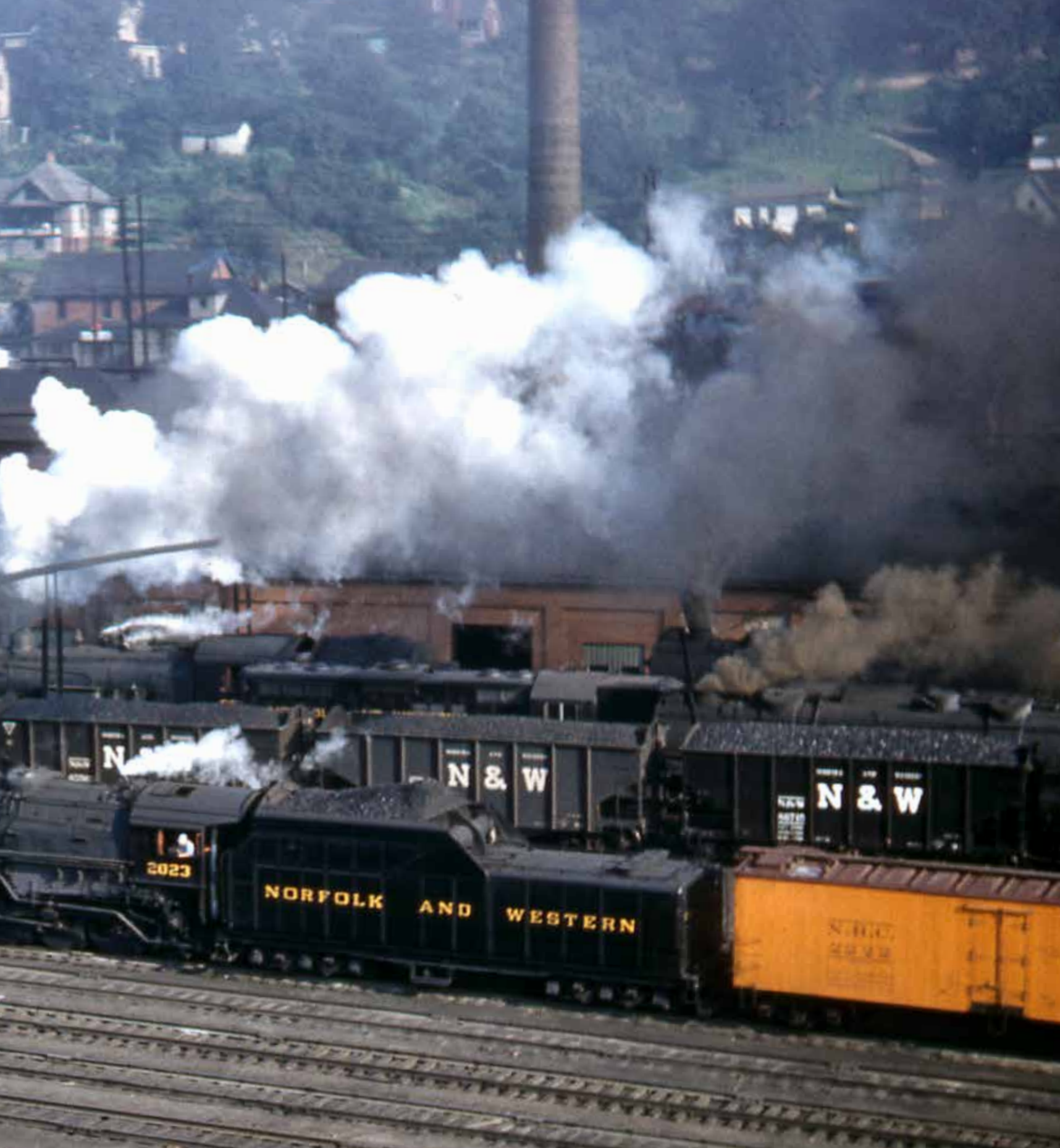
No Class I railroad kept faith with steam longer than the Norfolk & Western, which didn't buy a diesel locomotive until 1955. And no road was a better friend to the 2-8-8-2 Mallet — N&W rostered 227, more than any other carrier, and built them until 1952, decades after the type had fallen from general favor. N&W 2023, pictured at Bluefield, W.Va., in 1958, is a class Y3, one of 50 built for N&W under USRA auspices in 1919. Robert A. Caflisch, Helen Caflisch collection
