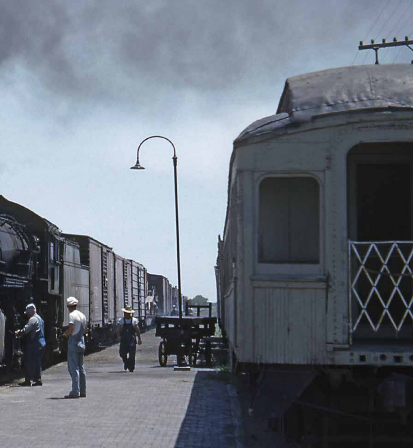
At Socorro, N. Mex., 75 miles south of Albuquerque on the Santa Fe's line to El Paso, 2-10-0 No. 2566 has just come off the Magdalena branch as mixed train 44. Now, the white flags are up and the train will run as an extra north to Belen to tie up. The Decapod is a former Kansas City, Mexico & Orient engine built by Baldwin in 1925. This sun-drenched scene of small-town railroading was recorded in June 1953. Stan Kistler
