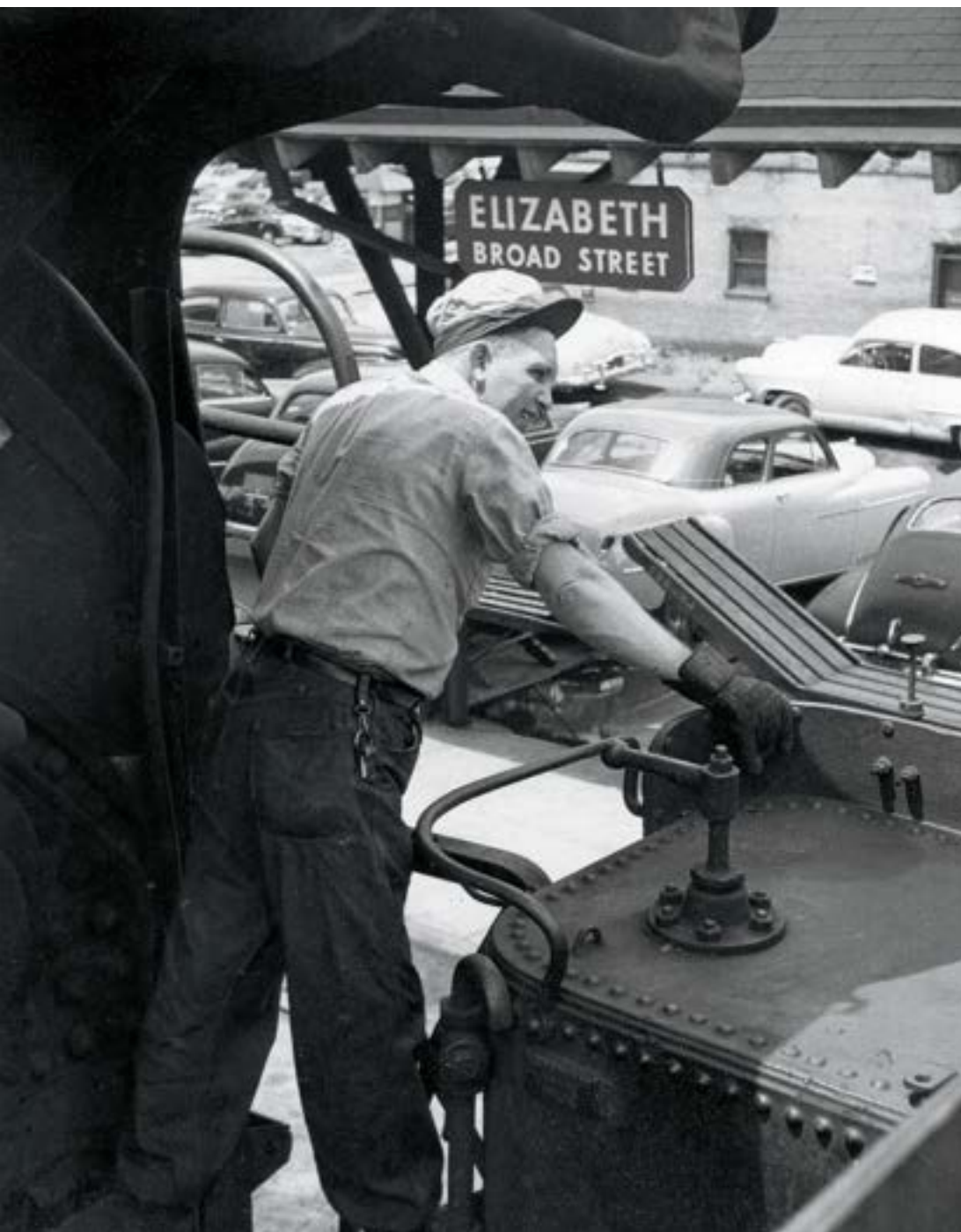
Ballinger watches for the highball at Elizabeth in the time-honored pose that, more than any other, perhaps, captures the spirit of railroading aboard a Camelback. His job is complicated by the fact that while firing he is actually standing on the deck of the trailing tender. Synchronization is needed.
