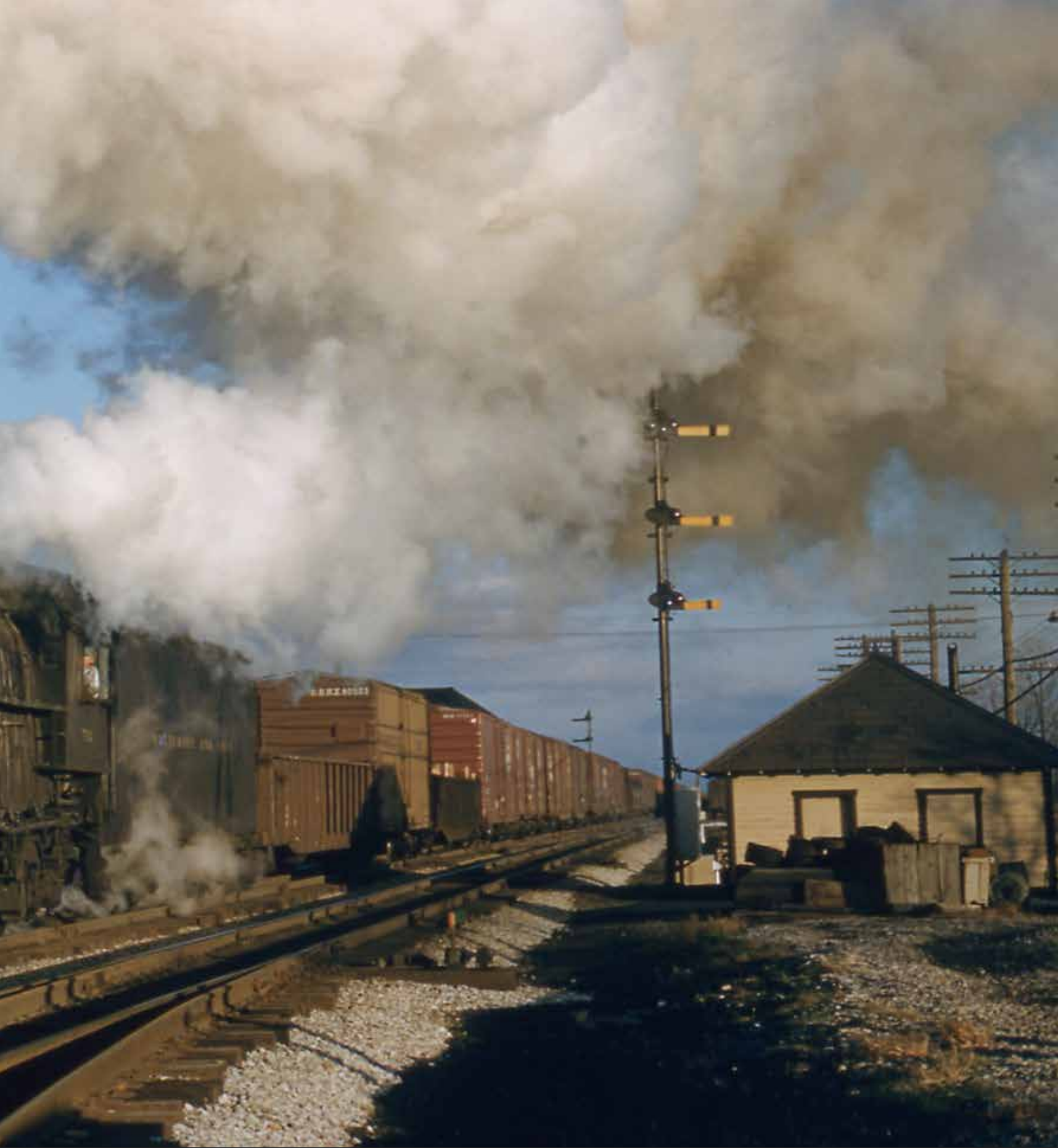
With dirty white extra flags snapping in the wind generated by its headlong rush westward, Baltimore & Ohio 4-8-2 No. 702 storms through Attica Junction, Ohio, on November 24, 1957. B&O built 40 of these class T-3 dual-service Mountains, Nos. 5555-5594, using the boilers from old Pacifics and Mikados during 1942-48. The road's general renumbering in 1956 put them into the 700 series. A diesel pioneer, B&O entrusted fast freights to 4-8-2s after other roads had vanquished steam. Frank Tatnall
