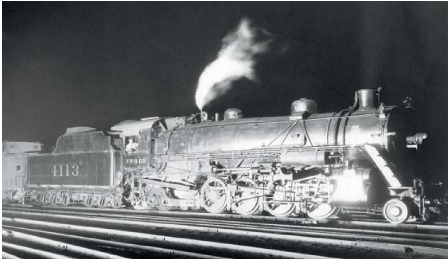
The USRA's influence extended far beyond the World War I agency's 26-month lifespan, notably in locomotive design. Thousands of engines, some built decades later, were direct descendants of standard USRA types. The Frisco's 65 2-8-2s of 1923-26, for example, were near-copies of the USRA heavy Mikado.
