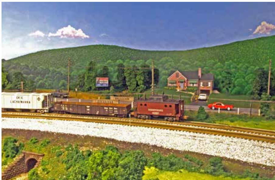
4. West of Mifflin Interlocking, the railroad drops down to two tracks on a three-track right-of-way. The space previously occupied by the torn out tracks is now used for a service road. Originally four tracks, the railroad was reconstructed with centerlines increased from 13 to 16 feet, and vegetation began to encroach in this scene re-creating the 1960s.
