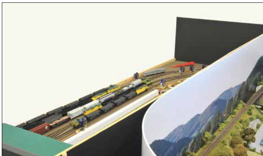
Removing the valance reveals the staging tracks and the Peco SmartSwitch servo motors that operate all of the staging turnouts. The scenic backdrop is a photo printed on flexible foam board, which allows it to be curved at each end.
