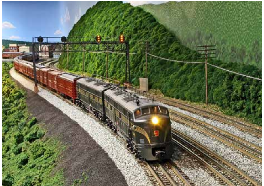
2. Tangent track was in short supply on the Middle Division as it meandered along the banks of the Juniata River. Most of Neal's railroad consists of alternating curves connected by short tangents. Note the sharp ballast edge and cinder shoulder in this scene modeling the 1950s.
