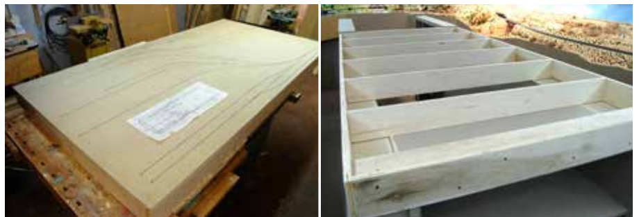
These photos show the track plan being transferred to the Homasote roadbed and the basic framework that supports the roadbed.
