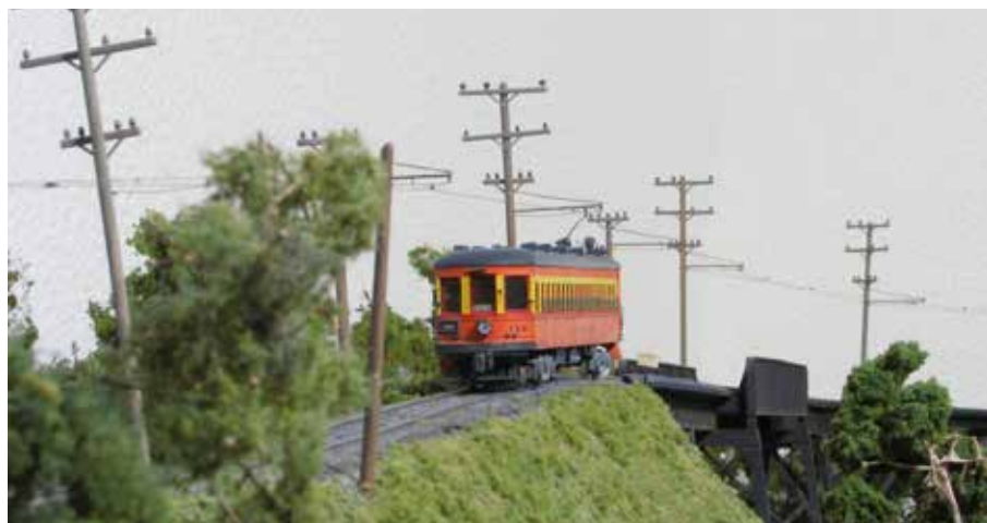
3. The downgrade past the bridge is one of the few spots on the line to Augustyn where the interurban isn't alongside a road. The grade here is about 6 percent, which is probably a little more than prototypical, but is visually acceptable.
