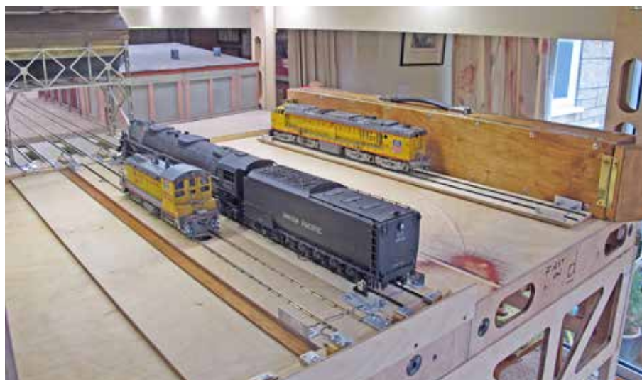
The offstage area has a three-track docking port/turntable. At right is a locomotive on a cassette. At center is a turntable that accommodates three cassettes (two are shown). The cassettes ease the task of moving heavy locomotives.
