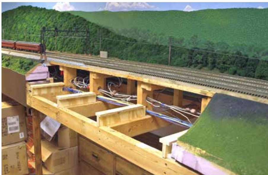
5. Most landforms are laminated pieces of 2"-thick extruded-foam insulation board from 2 to 5 feet in length. Here, one section has been removed to show the 8" high risers lifting the roadbed off the benchwork. The fill cross-section has a prototypical 3:2 slope.
