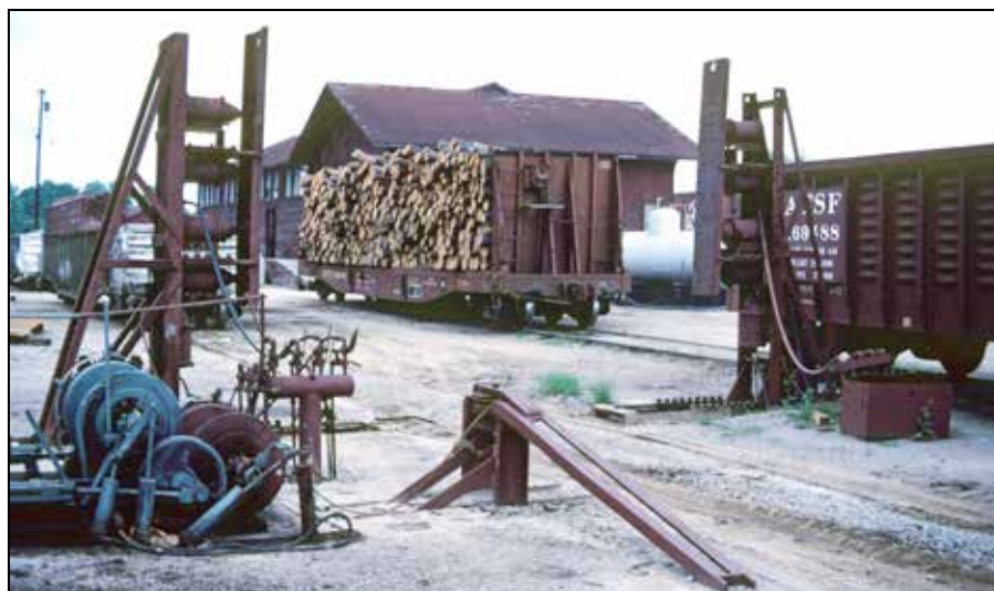
This pulpwood load shifter in the Santa Fe yard at Silsbee was used to straighten the pulpwood that was loaded onto flat cars.
