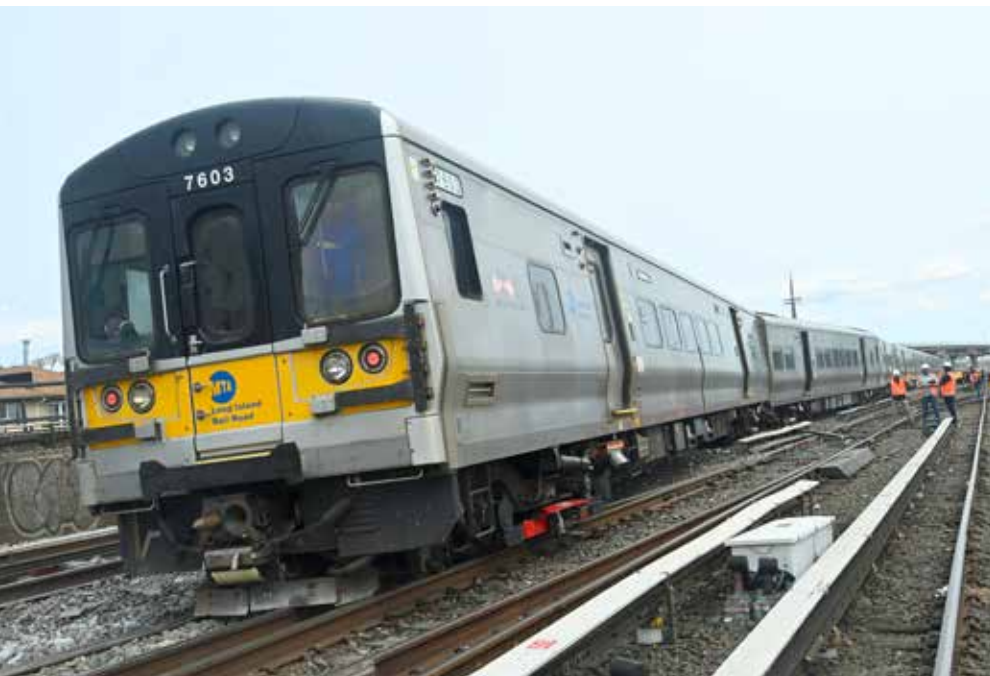
Workers examine Long Island Rail Road Train No. 722 after it derailed at 54 mph in Queens, N.Y., on Aug. 3, 2023. Thirteen people were injured. An investigation determined the switch was incorrectly lined, but a wiring fault led dispatchers to believe otherwise. MTA/Marc A. Hermann
