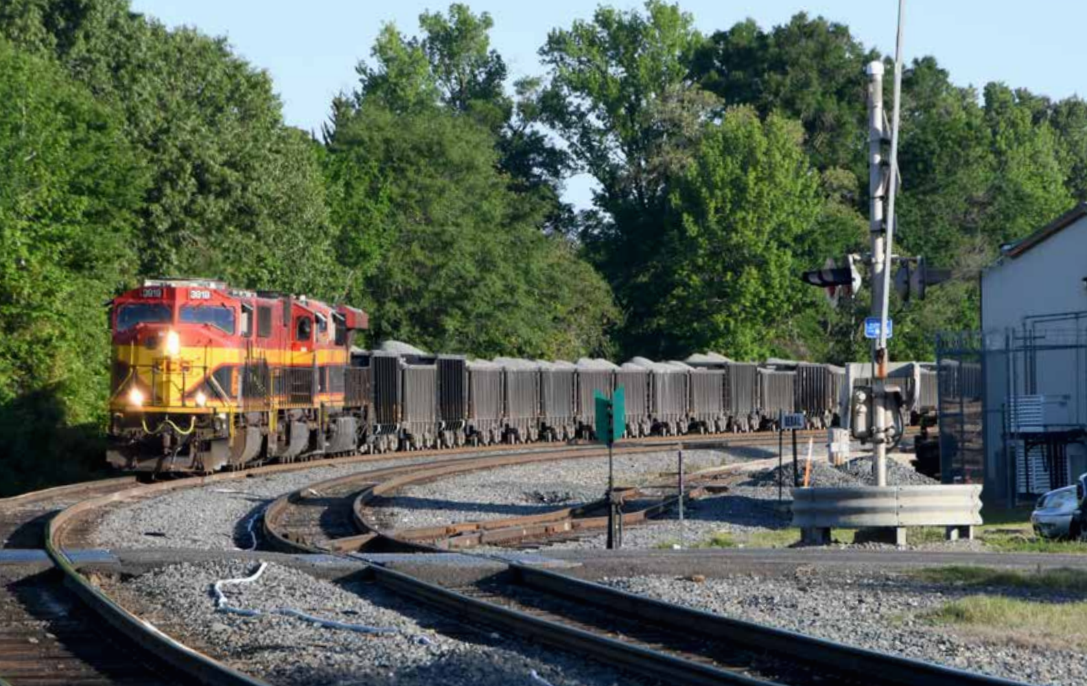
A loaded rock train waits in downtown Blanchard, La., 6 miles north of Shreveport Yard, on April 16, 2023. Blanchard is a holding point for trains needing access to or bypassing the yard. Notice the white air hose on the ground between the tracks. It supplies air to trains that need to clear the main line and cut for the two crossings in town. It's usually not a good sign if you need a portable air hose outside a major rail yard.
