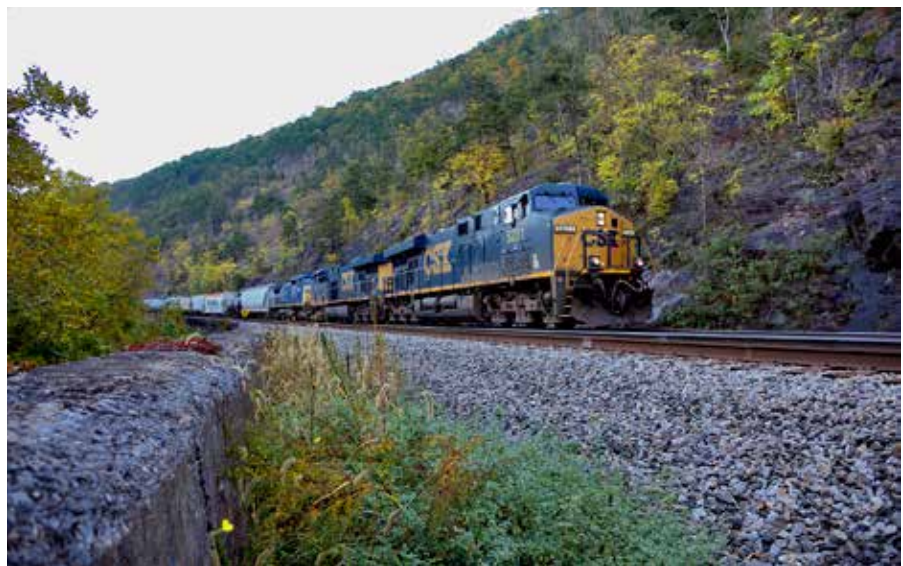
ES40DC No. 5231, a 2005 GE product, leads three locomotives hauling a train along the top of the wall with a touch of fall color in evidence during October 2016. Engineers developed a moving gantry to deliver concrete for the wall from a plant about a half-mile away.
