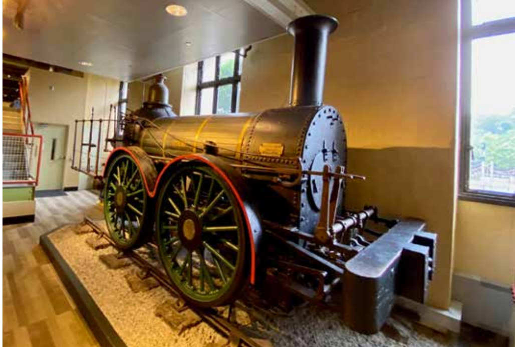
Weighing only 8½ tons, the 25-hp Philadelphia & Reading Railroad Rocket , built in 1838, is among the oldest preserved North American steam locomotives. Rocket has been transferred to the Railroad Museum of Pennsylvania from Philadelphia's Franklin Institute. Patrick C. Morrison
