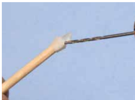
8 Using a toothpick to securely hold the round light allowed Thomas to be able to drill a hole in the casting near the mounting post.
