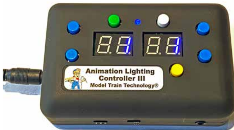
❶ The Model Train Technology LED Scene Controller can control 16 light ports with numerous lighting effects. Photo courtesy Model Train Technology
