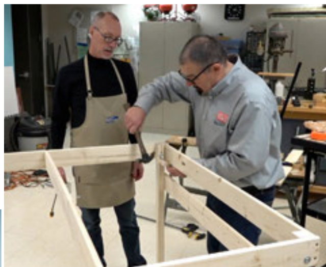
David Popp (left) and Hal Miller made the frame from standard 1 x 4 and 2 x 2 lumber with a ¾" plywood top. We designed our train table (shown below) to be sturdy yet easy to assemble.
