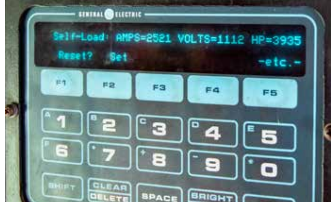
Throttle wide open (far left), former CSX Dash 8-40C 7640 performs a Notch 8 self-load test as it's readied for the road in GECX lease service. Vital statistics appear on the digital display panel in the cab (above), and on a weathered builder's plate (left) dated August 1990.
