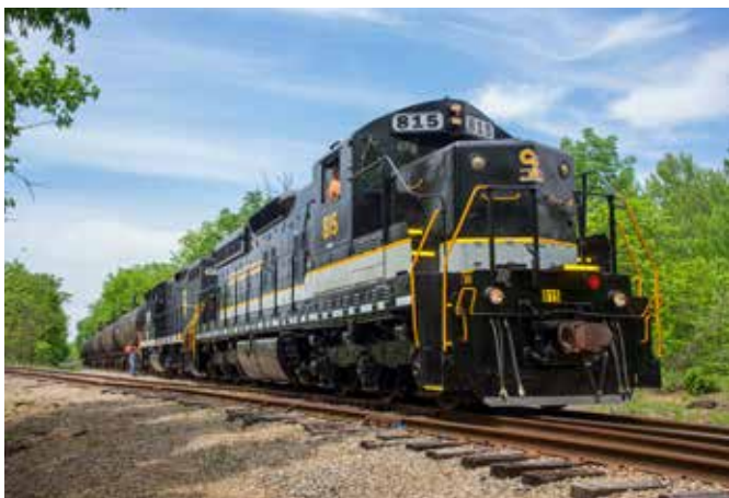
Fresh from the Olin shop, former Duluth, Missabe & Iron Range SDM No. 815 received new paint, as well as a rebuilt main generator, alternator, and 645-series engine.
