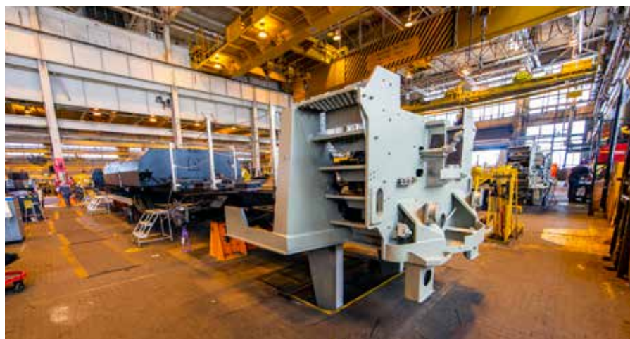
Retracing its path through its Erie birthplace, the rebirth of NS 8808 as AC44C6M 4006 begins as the main platform is refitted in Station 1 of Building 10. Two photos, Greg McDonnell
