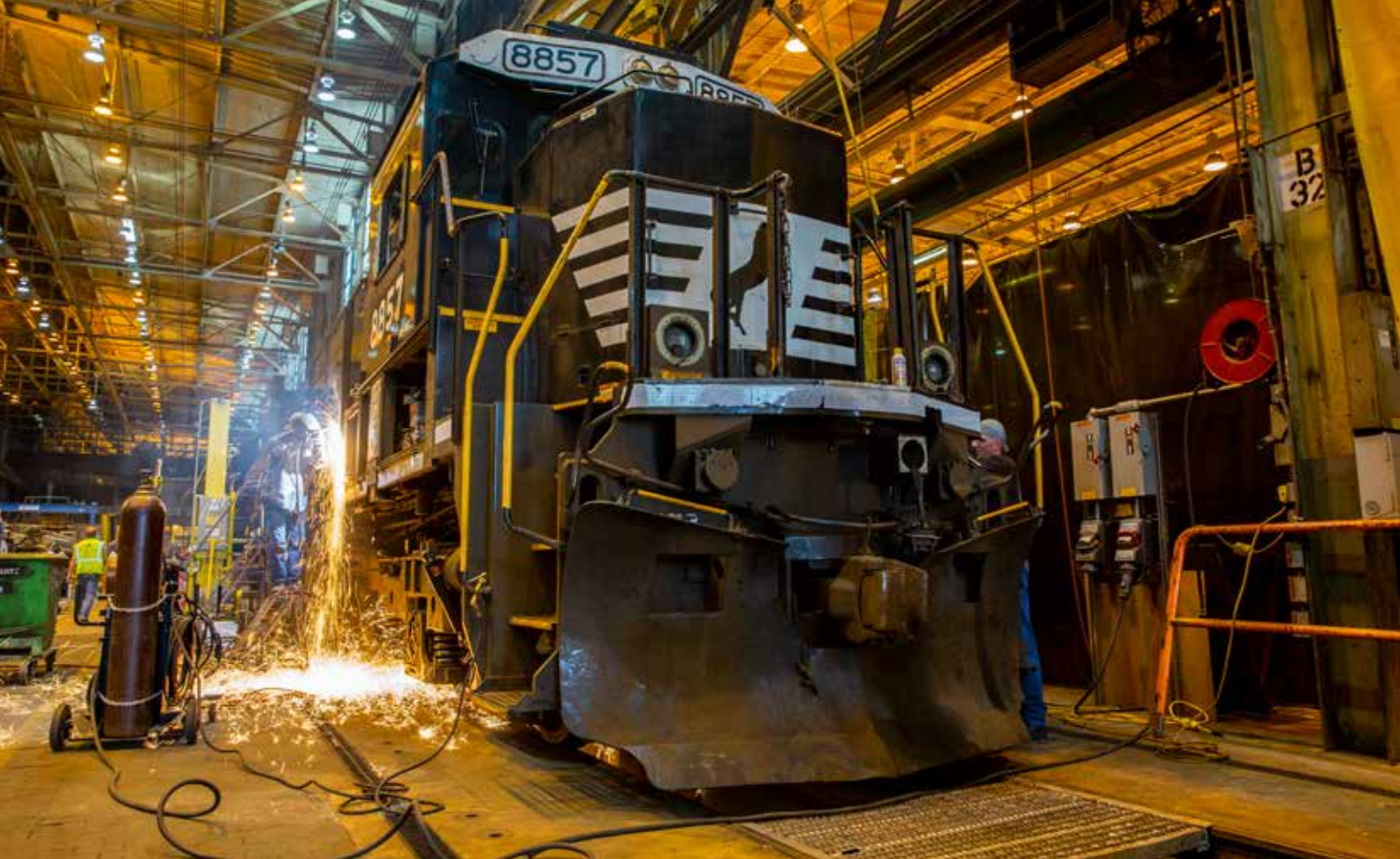
Workers at GE Erie cut away the cab of NS 8857 in preparation for its DC2AC makeover as AC44C6M No. 4011. The transformation will include new A.C. traction motors, EVO electronics, and a new operator cab.
