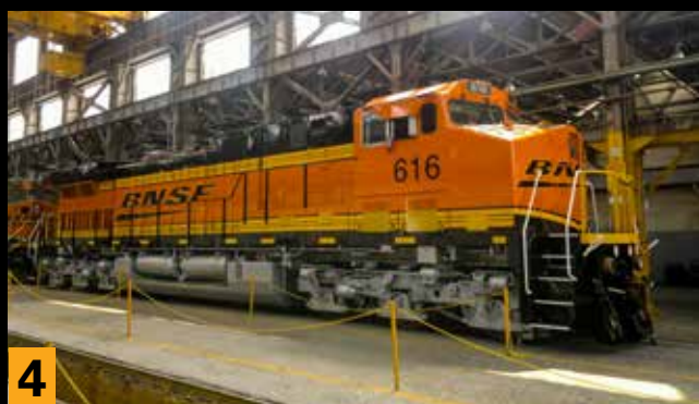
1. DC2AC prototype BNSF 616 enters the shop at San Luis Potosi, Mexico, as a tired Dash 9-44CW in faded warbonnet paint applied at Erie in 1994. 2. Crews at SLP separate the body from the frame in preparation for a complete rebuild. 3. BNSF 616, stripped to a bare platform, awaits its rebuild. 4. BNSF 616 debuts as an A.C. traction, A1A-A1A AC44C4M. Four photos, GE
