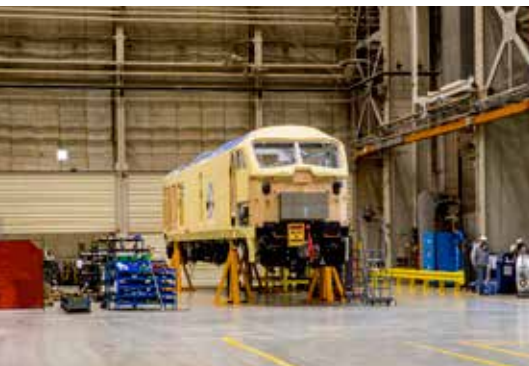
Monocoque carbodies for the F125 are shipped to Muncie from Vossloh in Spain. Three photos, Greg McDonnell
