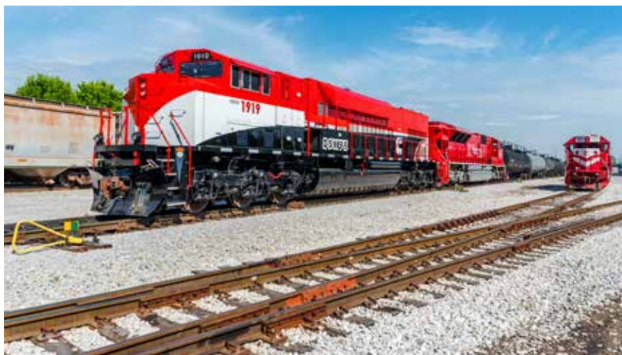
Cummins QSK95-powered HTL4200AC No. 1919, built from UP SD90MAC II No. 8559, tests in road service on the Indiana Rail Road in June 2016. Kevin Burkholder
