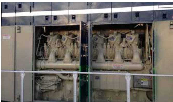
EMD's new Tier 4-compliant, four-cycle 12-1010J prime mover is the heart of the SD70ACe-T4 and 'P4.
