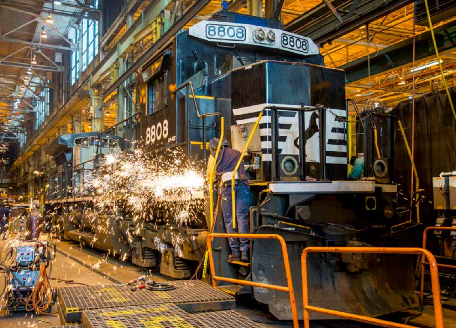
Sparks fly as crews at Erie cut away the standard cab and nose of NS 8808 in preparation for DC2AC conversion. The locomotive will receive an all-new wide-nose operator cab as part of its rebuild to AC44C6M No. 4006. GE: Steve Gerbracht
