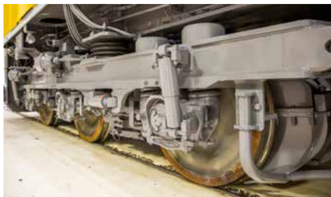
SD70ACe-T4 features include single-axle controls and the new fabricated-frame HTCR-6 truck. Greg McDonnell
