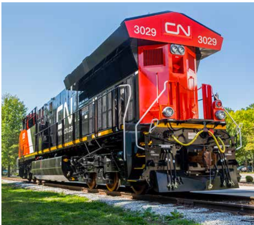
Rear view of CN ET44AC 3029 at GE Erie in September 2015 shows off the massive radiators that form one of the most distinguishing external features of the company's new Tier 4 Evolution Series locomotives. Greg McDonnell
