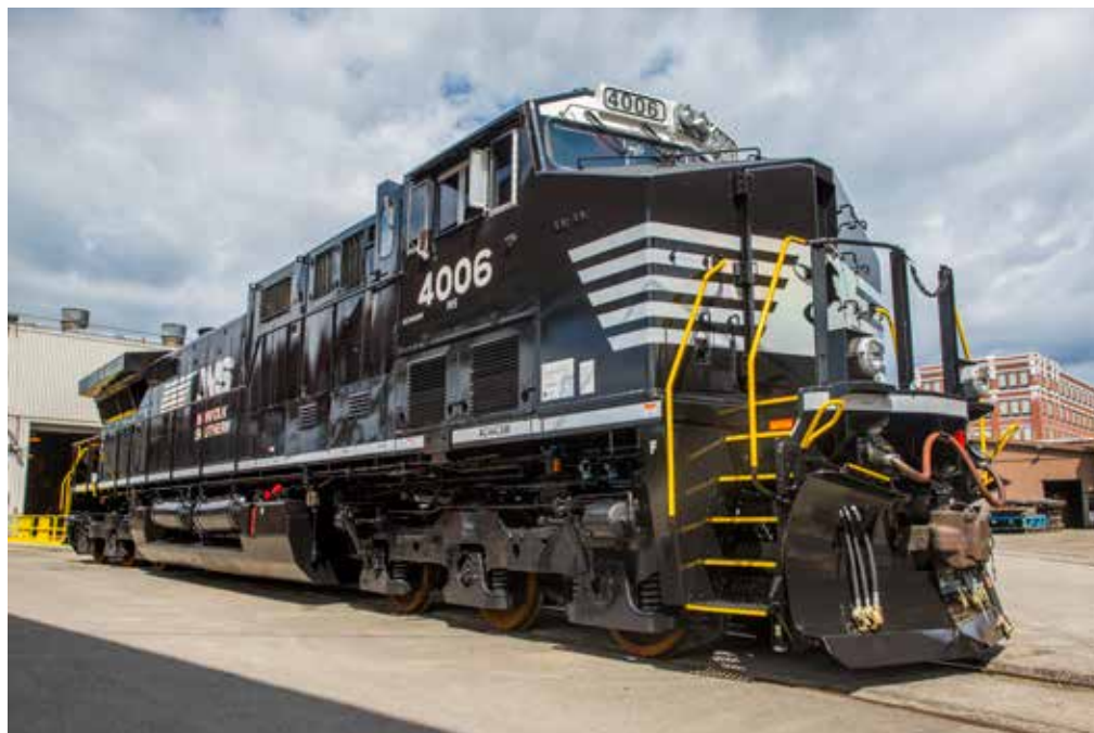
Its DC2AC transformation complete, NS 4006 (formerly NS 8808) poses outside Building 26 at Erie as it undergoes pre-delivery tests on June 27, 2016. Greg McDonnell
