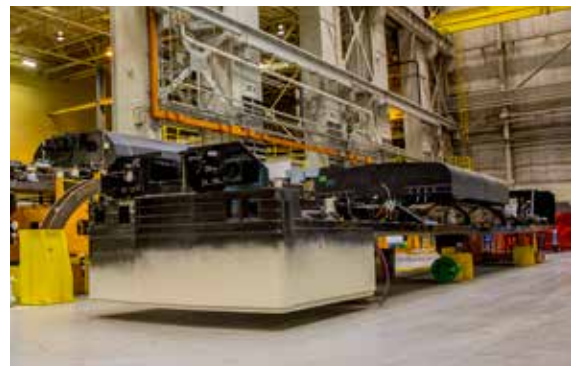
Frames for Metrolink F125s are rolled upside down to be outfitted with piping and wiring.
