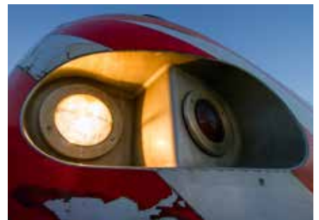
Metra MP36PH-3S No. 411 shows off its inset ditch and marker lights.
