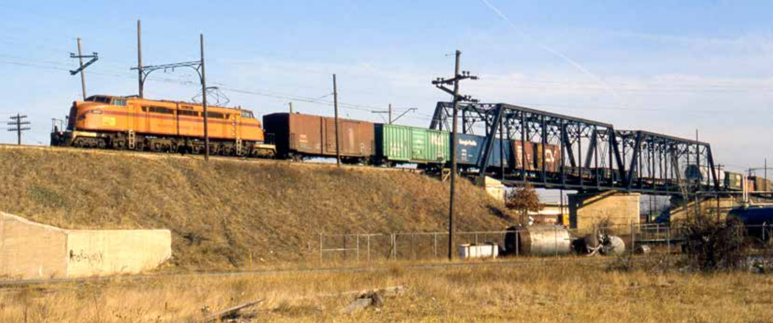
In 1949, South Shore purchased three of 20 massive 2-D+D-2 "Little Joes" built by GE for the Soviet Union but never delivered. No. 803 leads a westbound freight over the Penn-Wabash bridge in Gary. Lou Gerard
