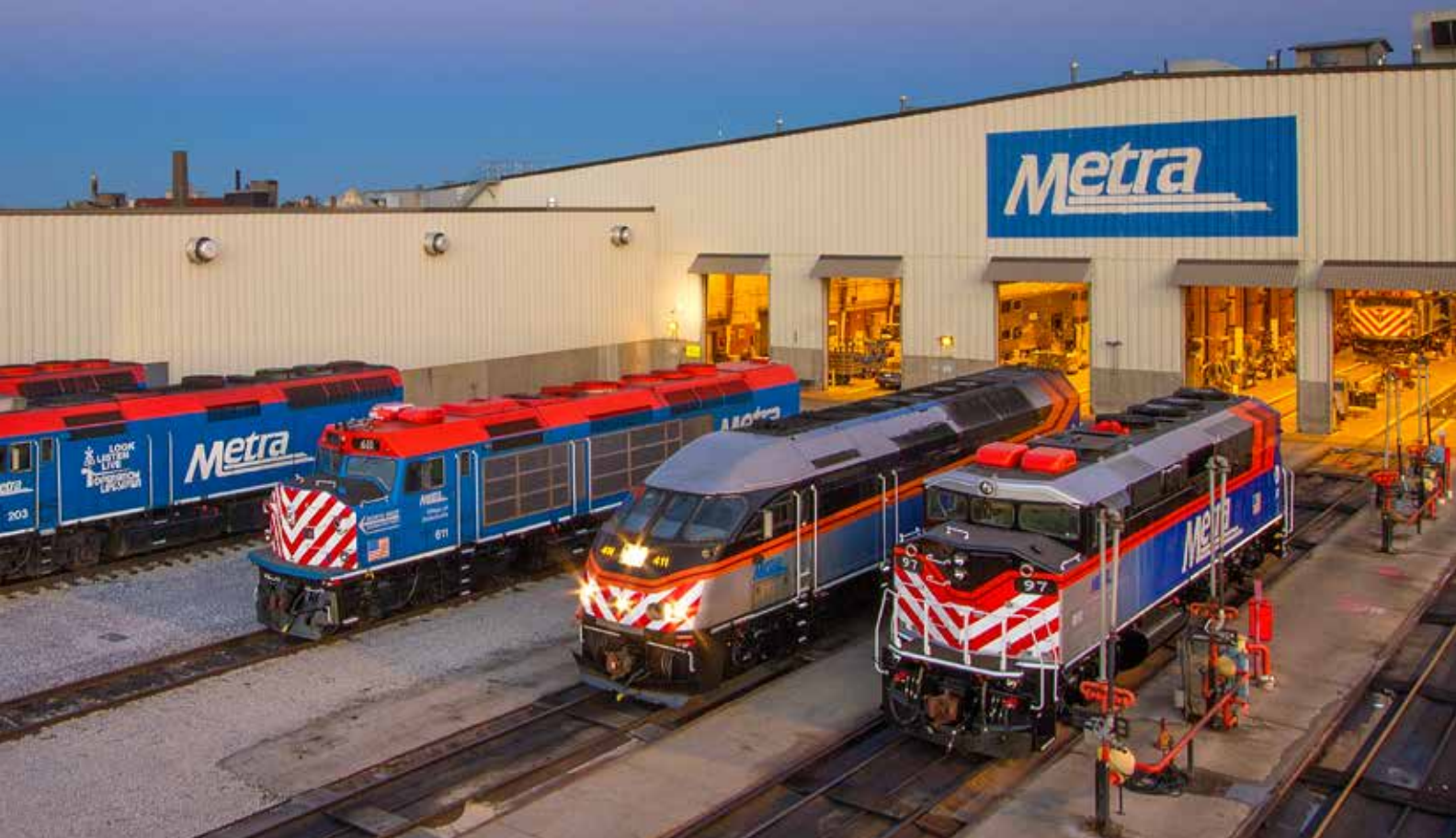
Each Metra road locomotive type has unique nose, windshield, and body configurations, as shown here outside the railroad's Western Avenue locomotive shop in October 2015.
