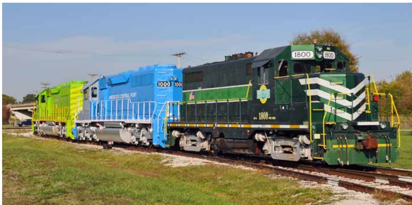
Port Harbor No. 1800 was one of 20 U.S. Army GP7s built with Type A switcher trucks. Acquired by the Alaska Railroad, it received Type B trucks from an RS1, and later, an upgrade to "GP8" specs at the Illinois Central Gulf shop in Paducah, Ky.
