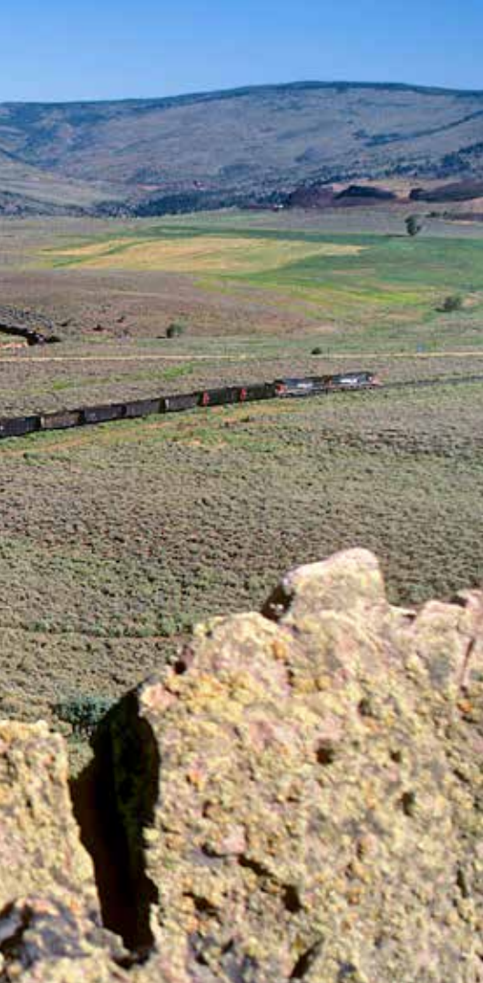
"Bigger trains plus more horsepower will make midtrain power mandatory." Two AC4400CWs up front, two midtrain, and one on the rear work an SP coal train through the Crater Loops near Crater, Colo. Mike Danneman
