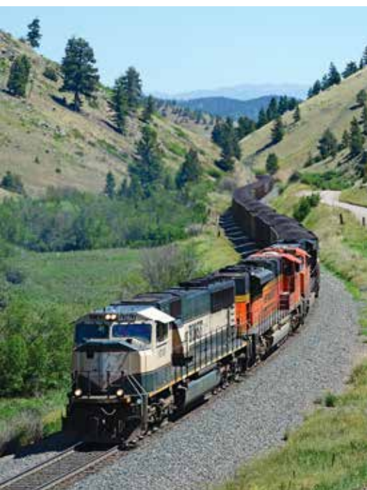
Coal's steepest climb to the Northwest is MRL's Mullan Pass. On July 2, 2012, three head-end units (BNSF Nos. 9740, 9227, and 5919, left), a quartet of MRL SD70ACe midtrain helpers (center) and rear distributed power unit BNSF No. 5761 tackle Mullan's 2.2 percent with 125 loads from Montana's Signal Peak Mine to the export terminal at Roberts Bank, B.C.
