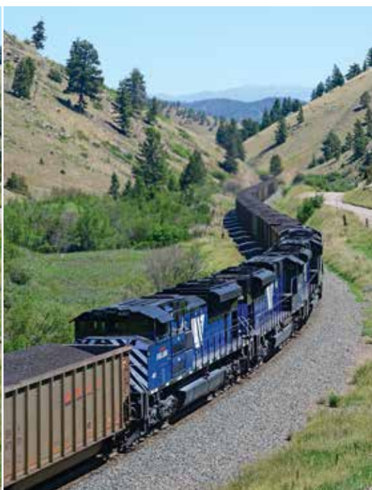
Coal's steepest climb to the Northwest is MRL's Mullan Pass. On July 2, 2012, three head-end units (BNSF Nos. 9740, 9227, and 5919, left), a quartet of MRL SD70ACe midtrain helpers (center) and rear distributed power unit BNSF No. 5761 tackle Mullan's 2.2 percent with 125 loads from Montana's Signal Peak Mine to the export terminal at Roberts Bank, B.C.
