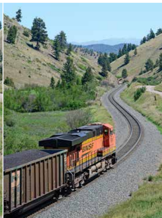
Coal's steepest climb to the Northwest is MRL's Mullan Pass. On July 2, 2012, three head-end units (BNSF Nos. 9740, 9227, and 5919, left), a quartet of MRL SD70ACe midtrain helpers (center) and rear distributed power unit BNSF No. 5761 tackle Mullan's 2.2 percent with 125 loads from Montana's Signal Peak Mine to the export terminal at Roberts Bank, B.C.
