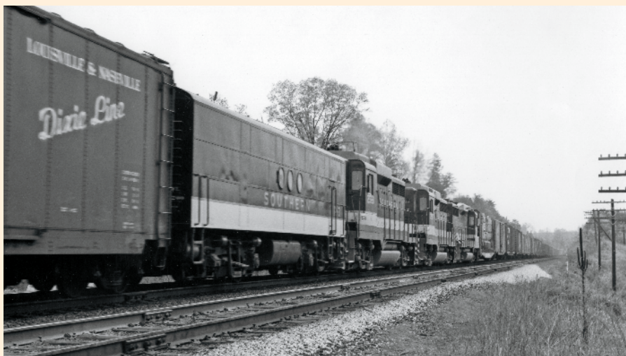
"Point of no return on couplers." Midtrain power (former FTB remote control receiver and three GP30s) on Southern No. 154 at Chatham, N.C. Curt Tillotson Jr.
