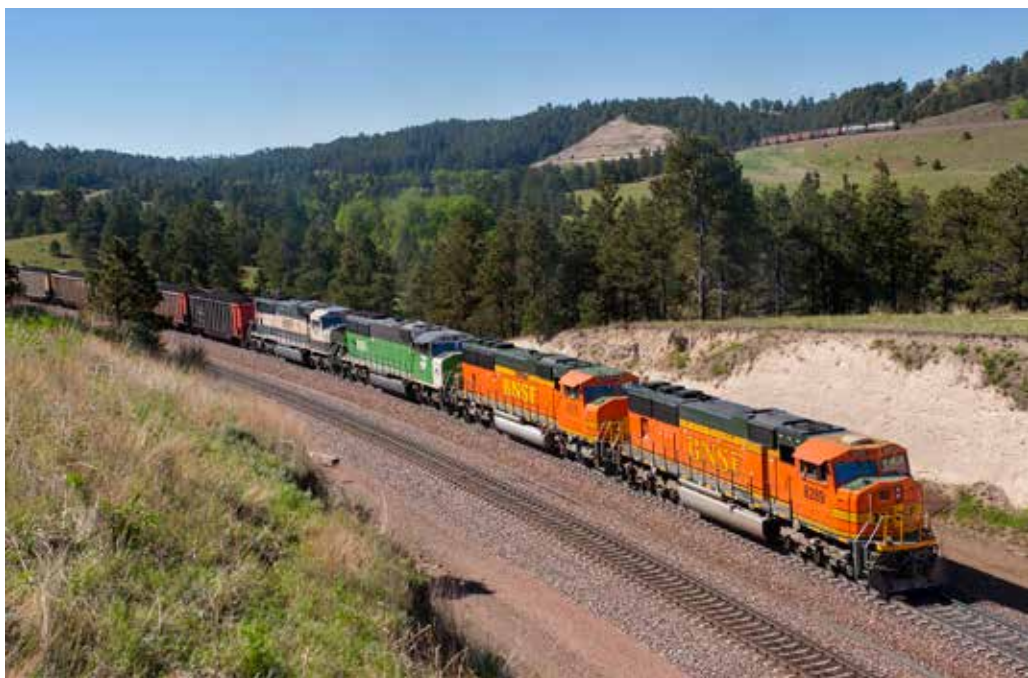
Three EMD models bring a coal train up Nebraska's Crawford Hill, on May 21, 2006. The train has two SD70MACs up front with another in DPU mode. The SD75I/SD60M/SD60M trio is a manned helper set. Tom Danneman
