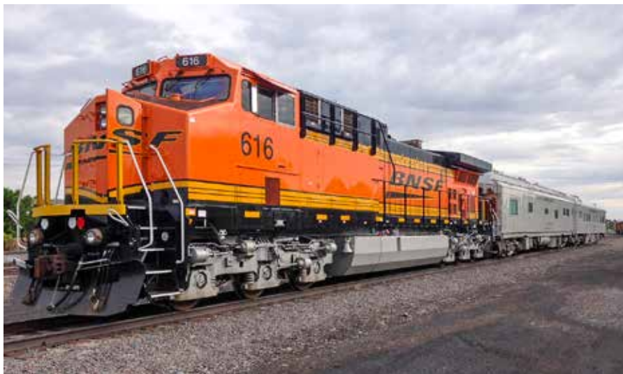
8. BNSF and NS are experimenting with A.C. conversions of D.C. locomotives. Built as a Dash 9-44CW, BNSF 616 was upgraded to an A1A-A1A "AC44C4M." GE
