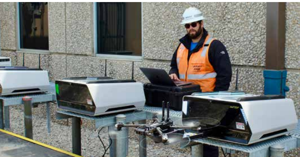
Pilot Stephen Bossert watches as a quadcopter launches from its dock at BNSF's Alliance, Texas, intermodal terminal to survey container locations and empty parking spaces — part of an effort to get drivers in and out of the facility more quickly.
