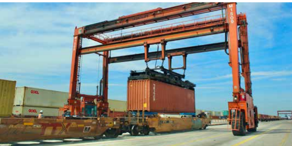
A crane lifts an international container off a stack train at BNSF Railway's terminal in Alliance, Texas, in March 2023. BNSF aims to keep production tracks clear of congestion as a way to boost capacity. Two photos, Bill Stephens
