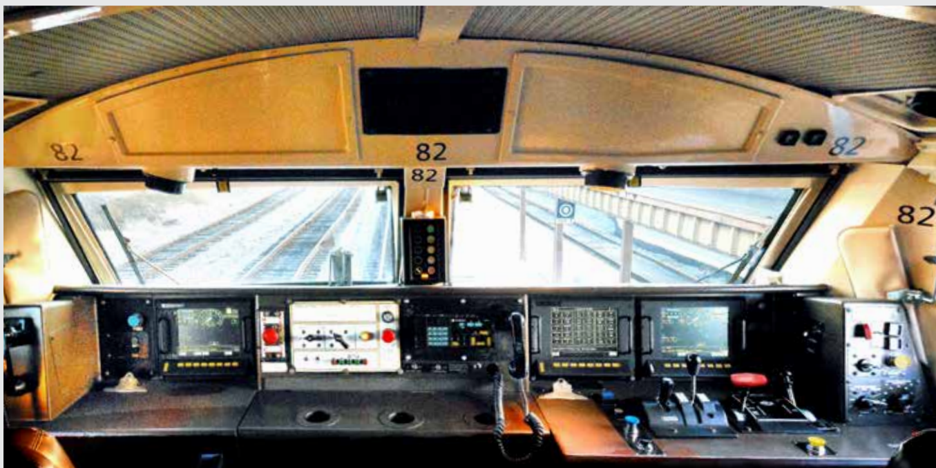
Locomotive controls have continued to evolve with the passage of time, but one of the most radical changes, at least for Amtrak engineers, came with the delivery of General Electric's Genesis locomotives. Two photos, Doug Riddell
