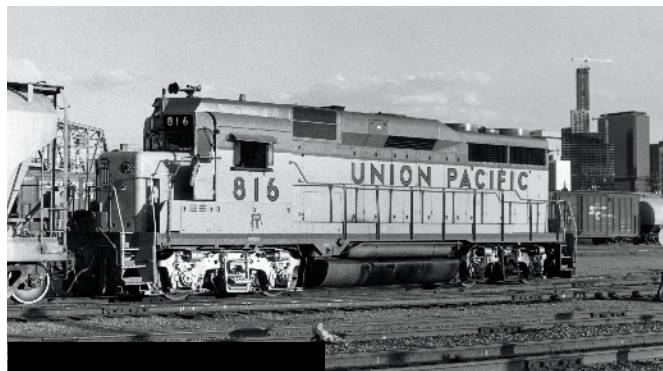
A GP30 in Denver in July 1982 is an example of UP using road units in yard work. J. David Ingles
