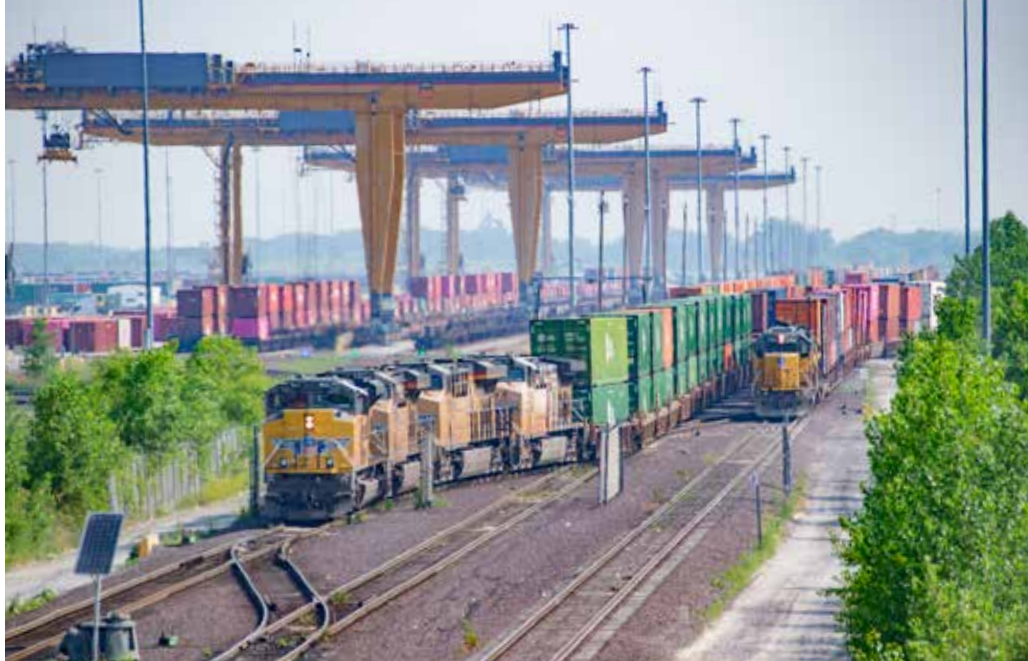
An arriving intermodal train delivers cuts of container well cars to the tracks at UP’s Global 4 terminal in Joliet, Ill., on June 17, 2023, as a switch crew works on an adjacent track. UP is testing electric wide-span cranes at the facility as part of upgrades leading to greater efficiency.
