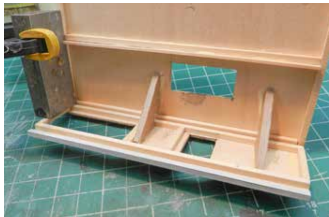
5 Hip to be square. Frank clamped his walls to rectangular metal slabs to ensure the joints would dry square.
