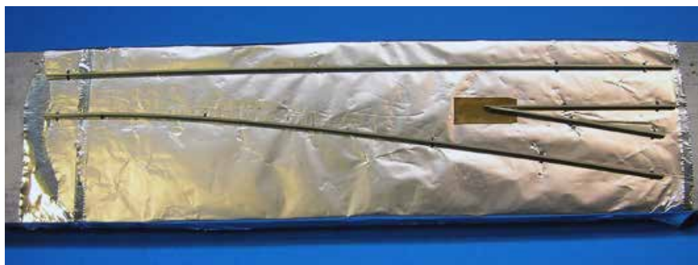
3 The stock rails are then spiked to the base to establish the outside shape of the turnout.
