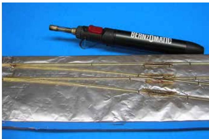
8 The frog, guardrail, and point tabs are soldered using a small propane torch. The four layers of foil help to dissipate the heat.
