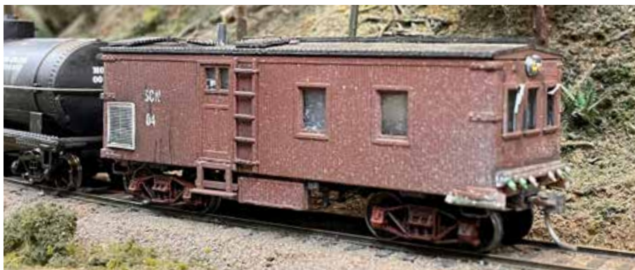
Since the weed sprayer was a rush job to make a deadline, after its first appearance on Paul's layout, Jim took the model back and added some much-needed extra details, including a headlight, windshield wipers, grab irons, and a big air intake vent to equipment end of the car.
