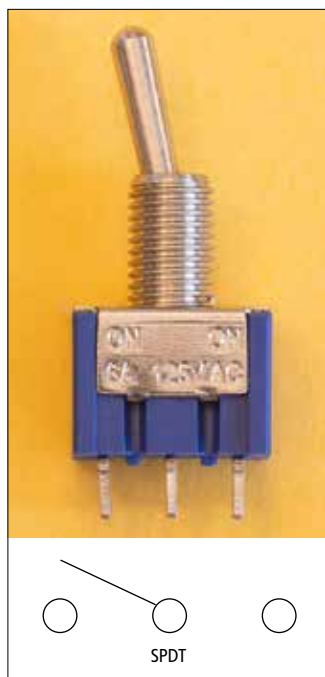
3 A single-pole double-throw (SPDT) switch. Some switches will have information stamped on the sides indicating what kind of switch it is and what the maximum operating current and voltage is.
