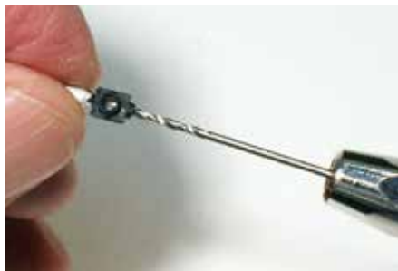
2 Using a \frac{3}{64} " drill bit, Tom drilled a hole in the mounting post of the casting which will accommodate the wires for the LED light.
