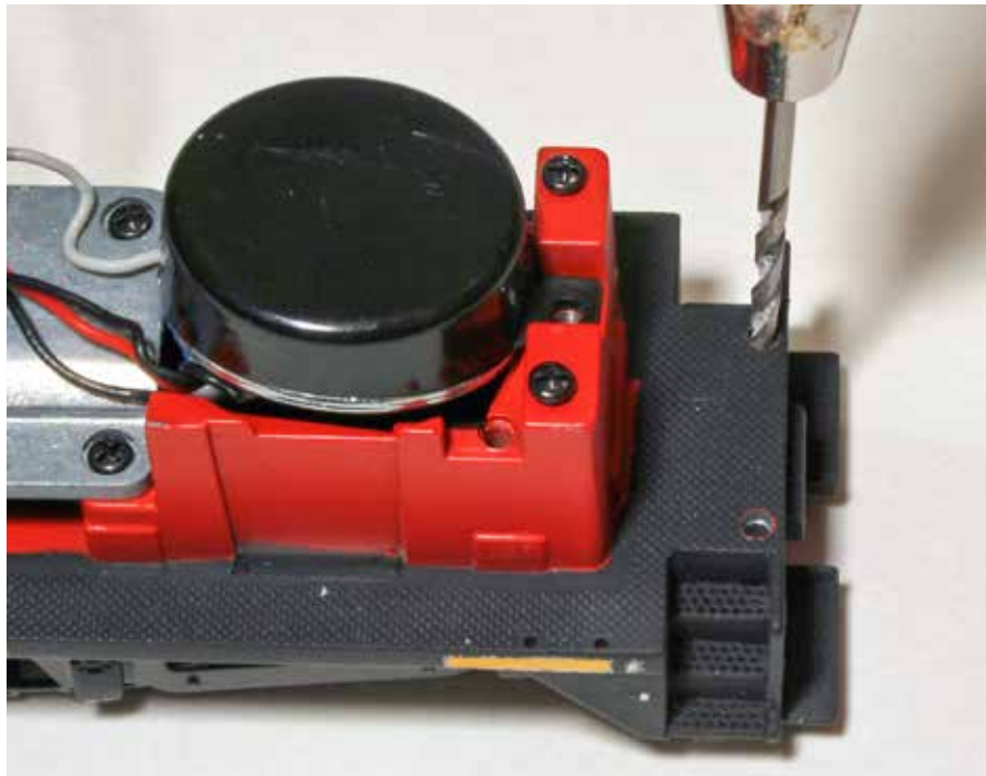
1 Tom used a \frac{5}{64} " drill bit to enlarge the hole in the frame to accommodate the mounting post of the ditch light.
