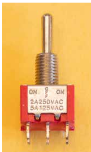
5 A double-pole double-throw (DPDT), center-off switch. Alan uses this switch for his programming track.
