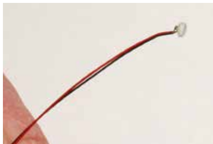
4 Placing a slight bend in the wires on the back of the LED helps it to sit flush in the housing and directs the wires down the shaft of the casting.
