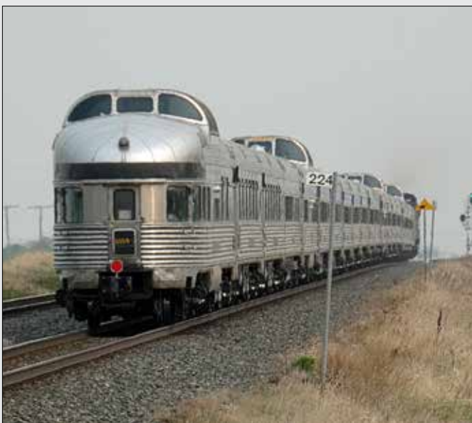
BUFFERS NO MORE The first VIA Rail Canada Canadian to operate without buffer cars rolls through Spy Hill, Saskatchewan, on May 21, 2023. Transport Canada rescinded its order requiring the buffer cars following a series of structural tests that gutted several vintage Budd-built cars; test results were not released and the agency and VIA have never explained what prompted the buffer-car order. David Maiers
