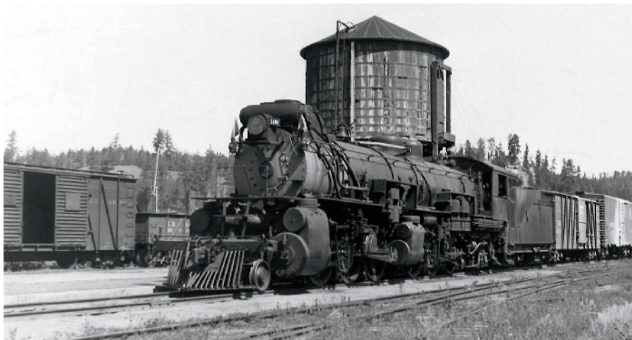
The Burlington had 10 of these T2 class 2-6-6-2s built by Baldwin in 1910. The T2s, among only a handful of CB&Q articulated locomotives, were assigned to Edgemont-Deadwood service. One of them, No. 4106, is shown at the Hill City water tower in this undated photo. C.T. Steeb
