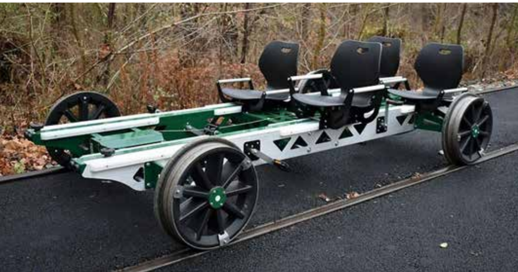
The Rail Glider is a new type of railcycle designed by the Colebrookdale Railroad. The railroad also manufactures the cycles, providing jobs for the community. Two photos, Colebrookdale Railroad
