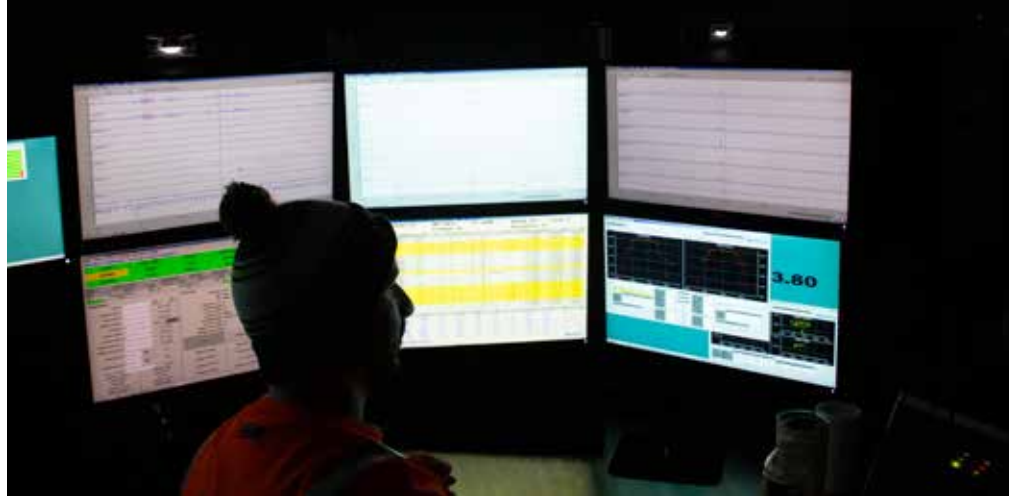
Alexander Grace watches the displays for the various inspection systems as the car runs east from Bridgeport, Conn. While information from every system is displayed, his focus is on the screen that displays “exceptions” — possible track defects — which he assesses for possible further action.
