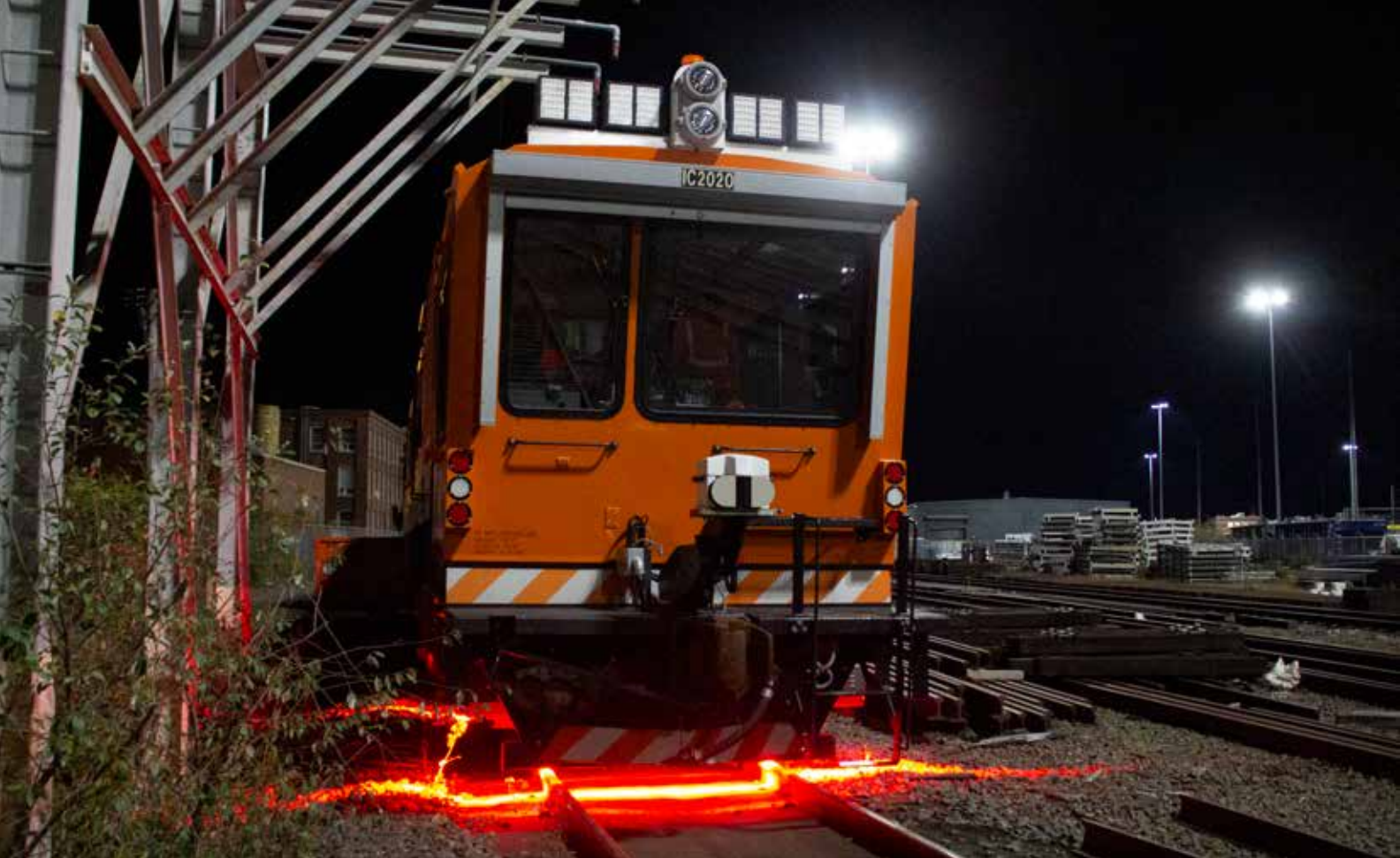
The laser for the clearance measurement system — projected from the arm in front of the car — lights the ground in front of the car in East Bridgeport. Note the spotlights — the row of white squares, turned off at this point — on either side of the headlight at the top of the car.
