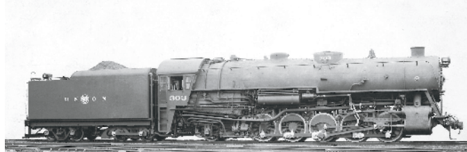
This profile view of Union 303 shows its immense size. It had 61-inch drivers and an 88-inch diameter boiler. Baldwin, Classic Trains collection
