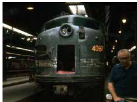
The nose of E8 4087 at La Salle shows the scars of its run-in at Delta earlier in the trip.
