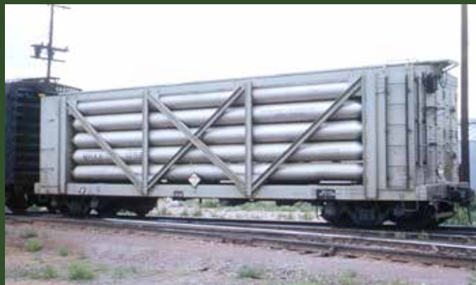
This is MHAX No. 1098, part of the Department of Interior/Bureau of Mines fleet, as it appeared in 1959. The cars were quite heavy with a light weight of 234,000 pounds. However, a full load of 279,000 cubic feet of helium weighed just 3,000 pounds. John S. Ingles, Jeff Wilson collection
