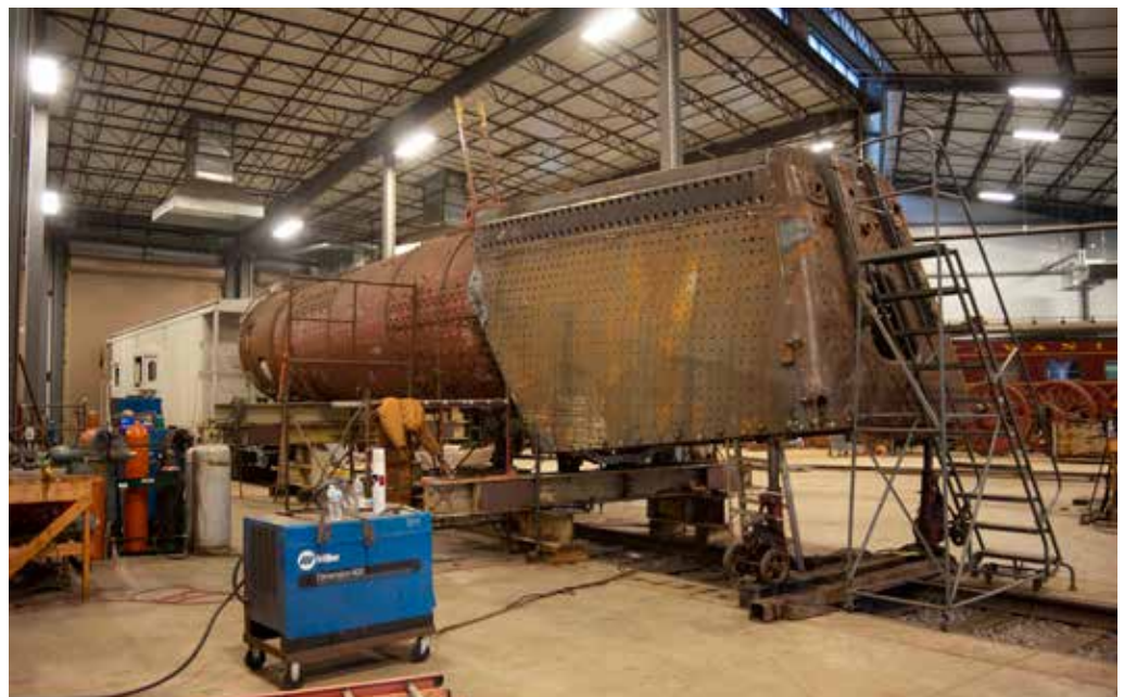
This December 2022 left-side view shows the left wrapper sheet and left Belpaire plate positioned against the round boiler courses of Pennsylvania Railroad K4s-class 4-6-2 steam locomotive No. 1361 in the Railroaders Memorial Museum roundhouse at Altoona. Dan Cupper
