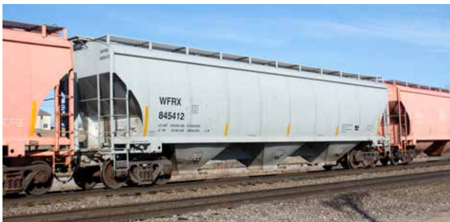
5 Non-railroad owners. Wells Fargo Rail Corp. No. 845412 is a lease car shown on the Canadian National at Ackerville, Wis., on March 7, 2020. The jack pad, which overlaps the sill above the trucks, features holes for pulling and lifting the car. This style of jack pad is used on all phases of the 5161 covered hopper.
