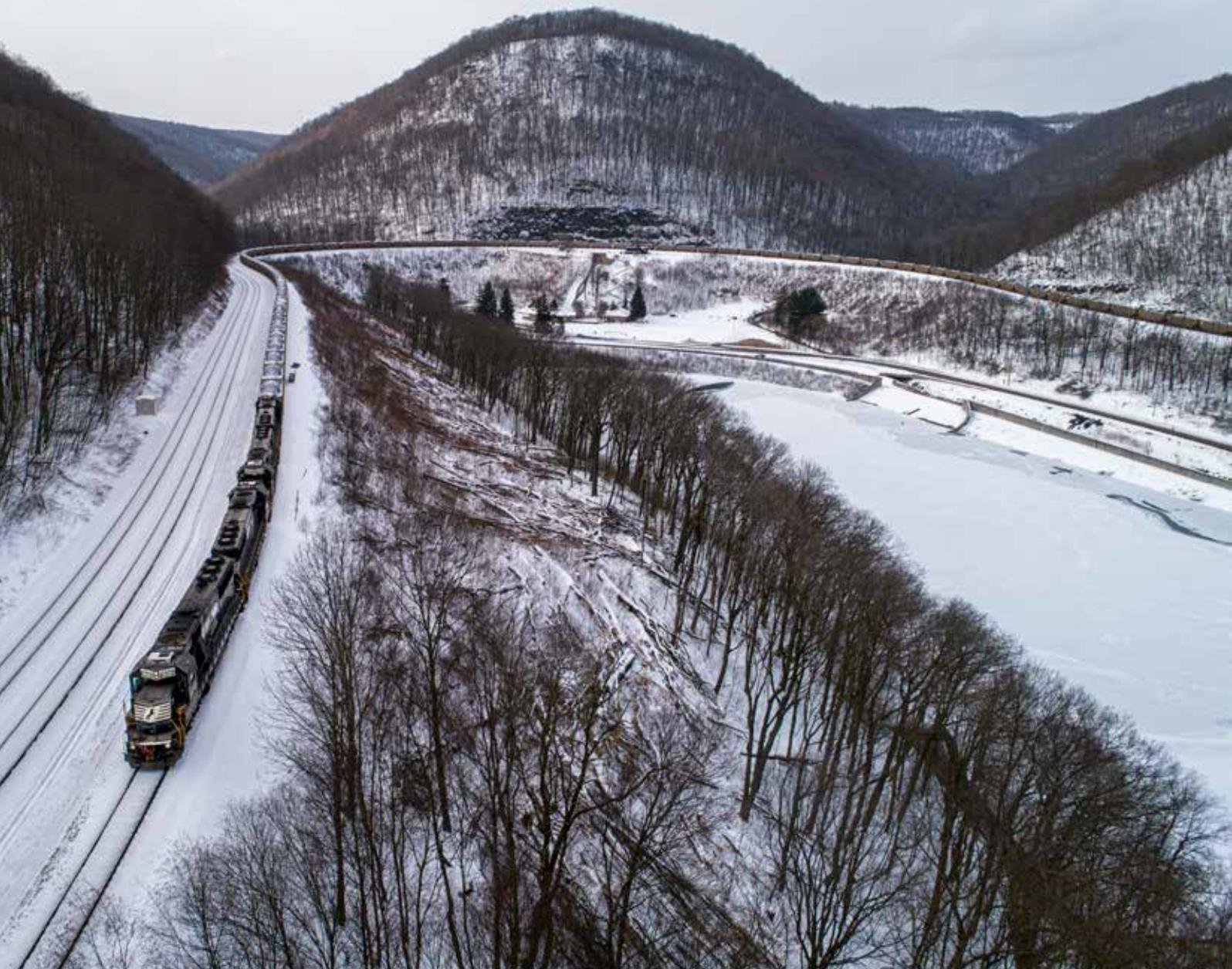
▲ A four-pack of helpers add their regenerative braking power to the rear of a heavy coal train heading down the mountain and through Horseshoe Curve on Jan. 26, 2019. The SD40E's role as the line's primary helper developed in the wake of a rebuilding program between 2008 and 2013.
