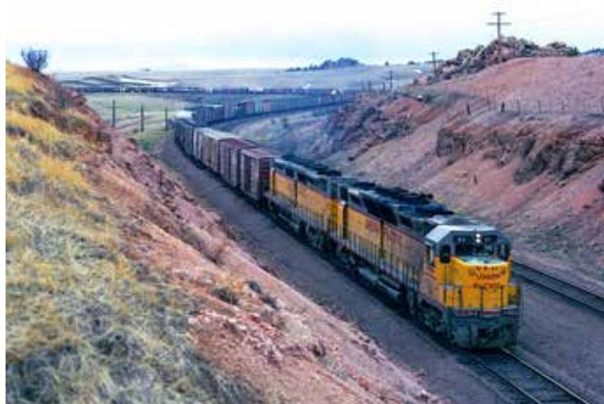
**First, EMD built the cabless DD35, second in this consist. Union Pacific asked for a cabled version, as well. Here DD35A No. 84 leads its train up Wyoming's Sherman Hill on May 12, 1968. Steve Patterson**
