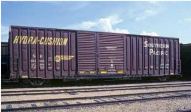
In the 1960s the boxcar grew in two dimensions — length and height. The length grew to 60 feet, while the interior height expanded from a standard 10 feet, 11 inches to a new hi-cube height of 13 feet.
