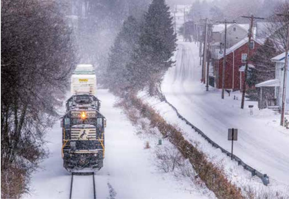
◀ Just yards from the crest of the Alleghenies on the west side of the New Portage Tunnel at Gallitzin, this helper set is transitioning from pushing up the mountain to a braking role as it helps an eastbound intermodal over the summit on Jan. 26, 2019.
