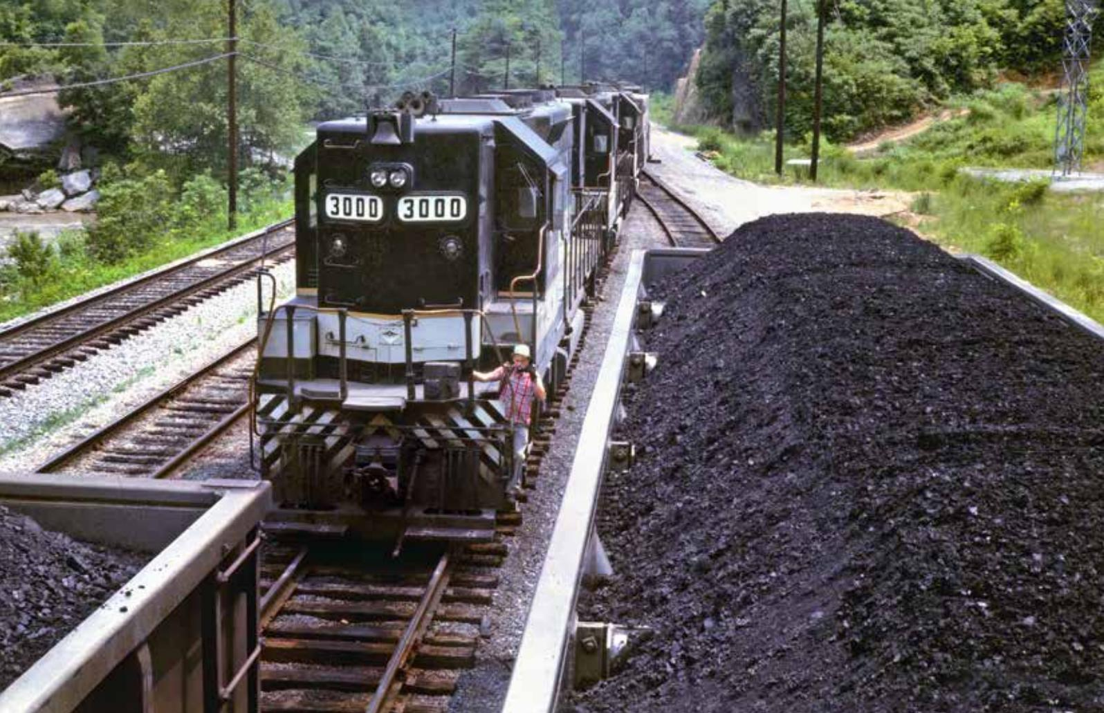
**Previously employed by Southern Railway, the author captured the Belmont unit train being made up at Appalachia, Va., on July 7, 1969. Head brakeman Billy Lawson talks the engineer back to couple the mid-train units and "radio car" to the rear of the train.**
