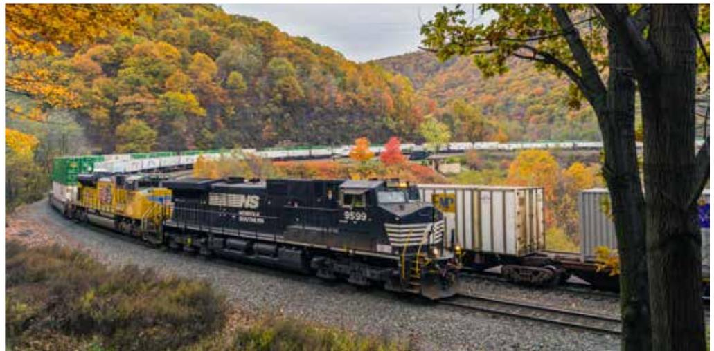
On a curve, whether ascending, descending, or level, steel wheels on steel rails can emit a squealing sound. One will often hear such sounds from trains on Norfolk Southern's Horseshoe Curve. Nolan Majcher
