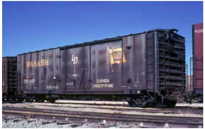
The 40-foot boxcar grew to 50-foot long in the early 1930s. Car doors became larger affording more convenient loading and unloading. The added length increased capacity to 70 tons. L.E. Raby, Tom Kline collection
