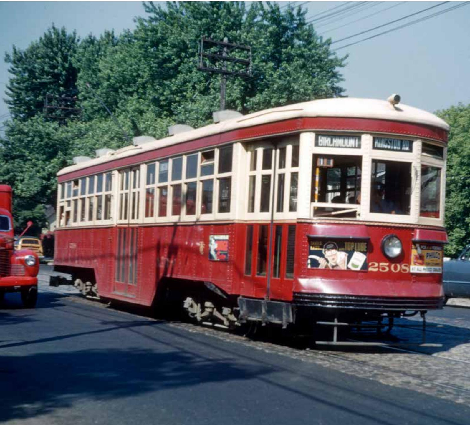
The 2508, a member of the 1921 order of “Big Witts” from Canadian Car & Foundry was among the cars that allowed TTC to retire many former Toronto Railway cars, top right. Operation of the Witts on the Kingston route began in 1939 and was made possible by shifts in car assignments due to the delivery of TTC’s new PCC cars. Rush service on the Yonge Street route required up to 70 Peter Witt motor-trailer trains, bottom right.
