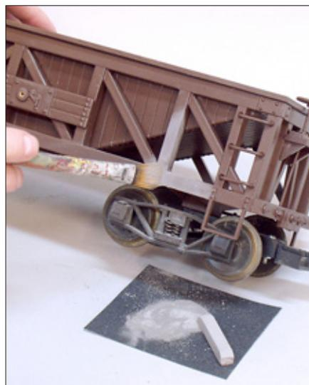
5. After first coating the trucks with chalk powder, the author then applied the powder to the body of the hopper car.
