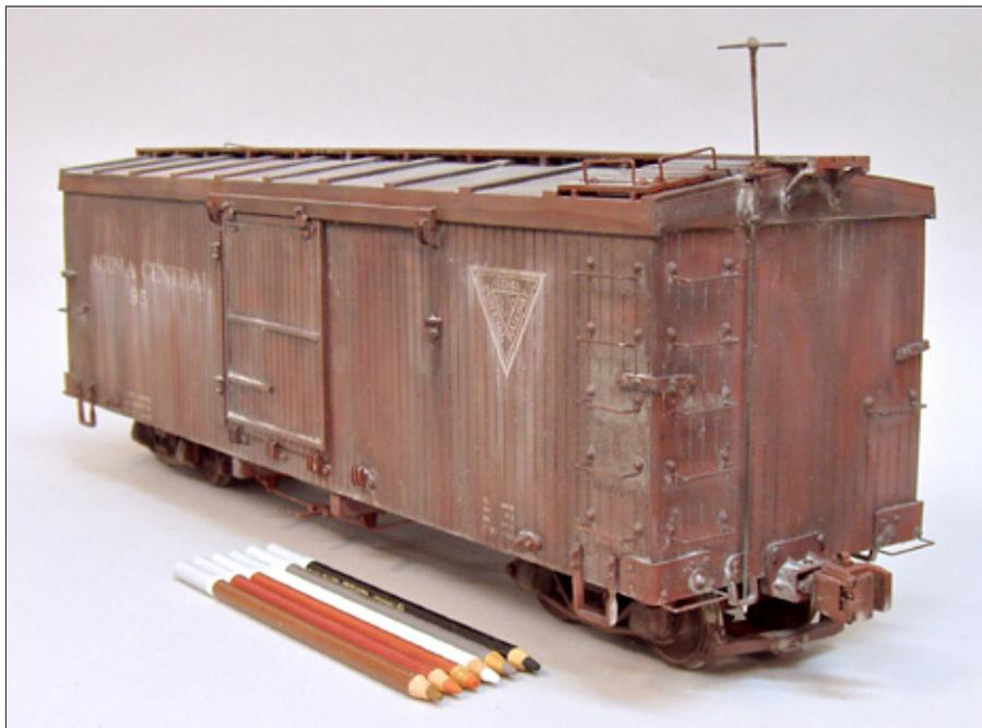
7. This car was built from a kit. When finished, it was given a coat of red-oxide primer and weathered entirely with the selection of chalk pencils shown beside it.
