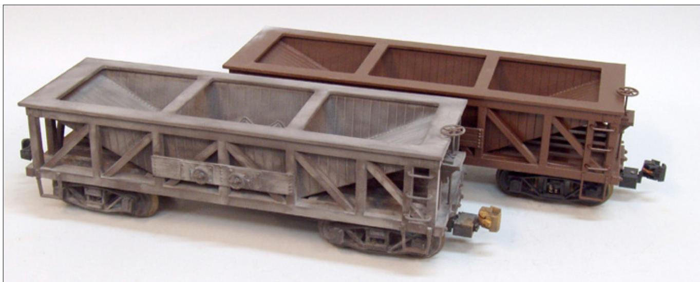
6. A comparison between a stock hopper sprayed with Dullcote and one that has been weathered with chalk. The various details of the weathered car have become much more noticeable and it looks like the car has seen some hard service in the real world.
