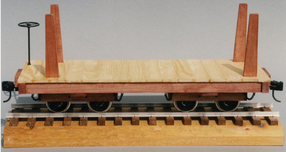
This is a generic, 7/8"-scale pulpwood car. It is based on cars built for the S.D. Warren Company and has features found in those 2'-gauge cars. The model is 14 1/4" long x 5" wide. This scales out to a car that is 17' long, which is a typical dimension for cars used by industrial railroads.
