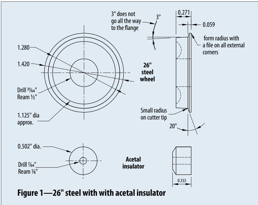
**Figure 1—26" steel with with acetal insulator**
