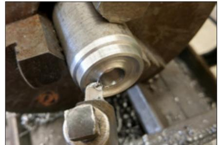
**3. The round-end cutter has been ground for this job from 5/16" high-speed steel. Tools are cheap and you can regrind them again and again when they wear. Push the cutter into the face of the part until you are happy with the look.**
