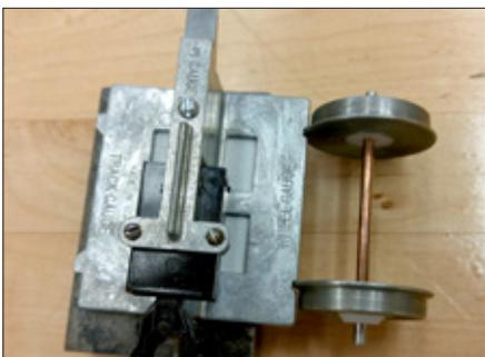
**8. A completed wheelset. The flanges should have a little play in the gauge. If one flange is tight to the right, the other flange should also be tight to the right.**
