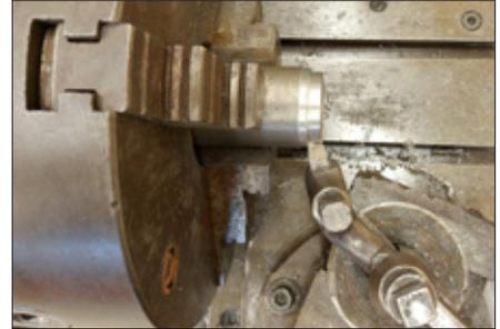
**2. The compound rest is turned 20° to the vertical. Note how close the carriage is to the chuck jaws. Always check for clearance when working close to the chuck.**
