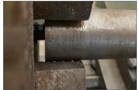
**1. This photo illustrates what *not* to do—the piece is not gripped properly. No matter how tight you make the chuck, if you take too heavy a cut with your piece like this, it is going to go flying.**
