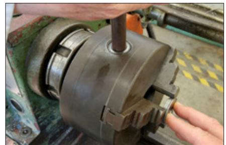
**4. When you reverse the wheel to end-face the saw cut, it is important that the wheel spins true before cutting. Close the chuck on the wheel, back it off a little, then push with two fingers while gently tightening the chuck. Turn on the lathe and check that it is visually running true. Take a cut and measure in a couple of places. If you are within .002", it is good.**
