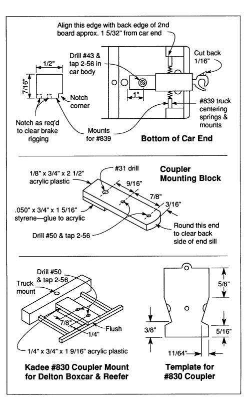
block. This must be a rigid piece without flex. Styrene can be used for all other pieces, and a piece slightly thicker than 1/8" would be a little better for the spring
