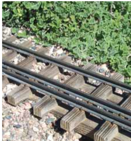
Redwood is more rot-resistant than other woods, making it a prime candidate for ties used in hand-laid track. It's still a good idea to periodically treat it with a preservative.
