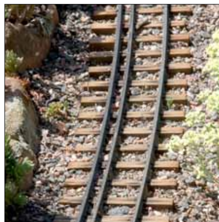
3. This three-rail track incorporates two different gauges—0 gauge and 1-gauge. Trains in 16mm-scale (1:19) and 15mm-scale (1:20.3) are equally at home on these rails.
