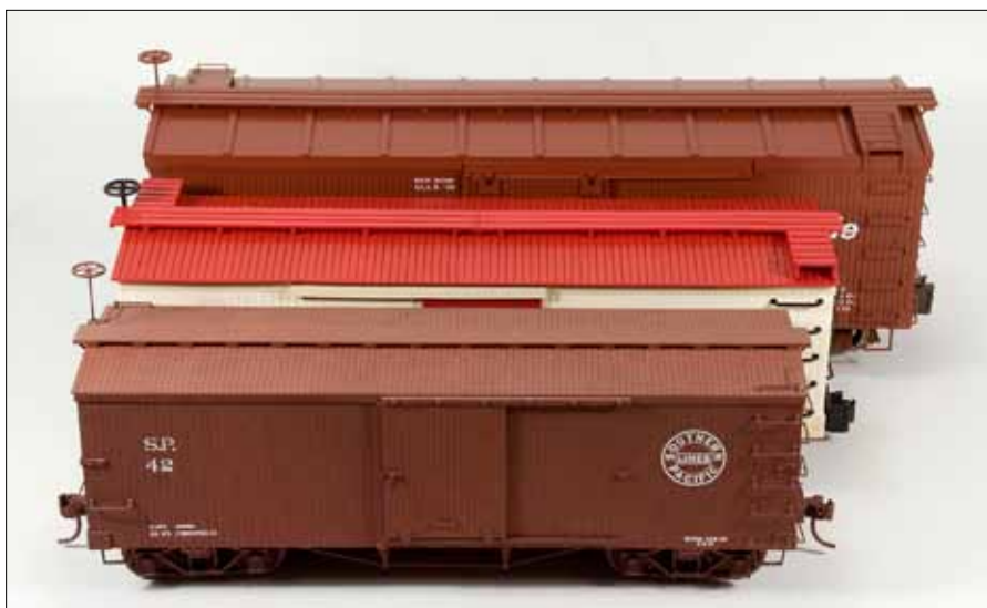
2. These three models are all of similar prototypes—3’-narrow-gauge boxcars. In the foreground is an early Hartford Products car in 1:24 scale; in the middle is a Bachmann boxcar in 1:22.5 scale; and in the rear is another Bachmann car, this one in 1:20.3 scale. All run on gauge-1 track but only the 1:20.3-scale car is the correct scale for that gauge.
