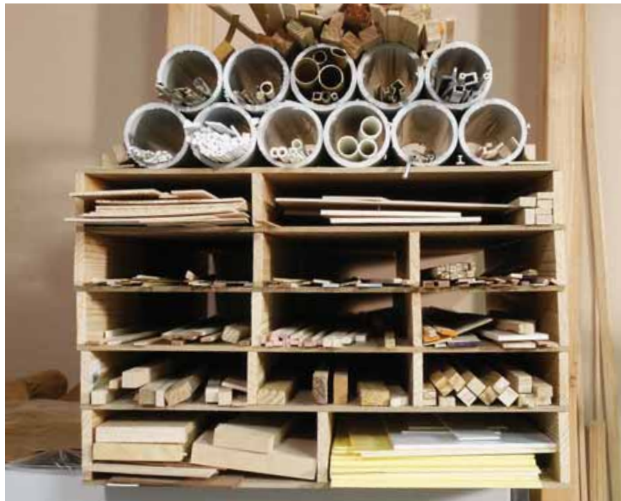
It's always a good idea to organize the raw materials in your workshop. A stock shelf like this allows you to quickly locate material of the correct size and type.
