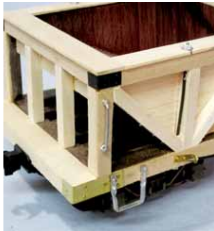
There's nothing wrong with mixing materials. The base of this hopper car is a commercial plastic hopper. The timbers are wood and the braces and details are metal, with the exception of the square, plastic nuts at the ends of the steel rods.
