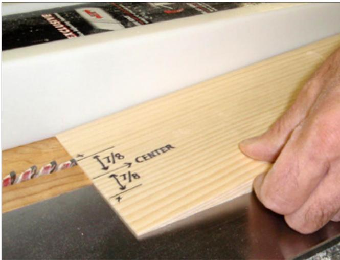
4. With a table saw, cut the grooves that will fit over the rails. Using a  $\frac{1}{8}$ "-wide blade, raise it to  $\frac{1}{2}$ " then line it up with the outside of the right-hand mark. Once this cut has been made, move the fence and set it to the outside of the left-hand mark for the second cut. Note the dimensions marked on the ramp—they are important.
