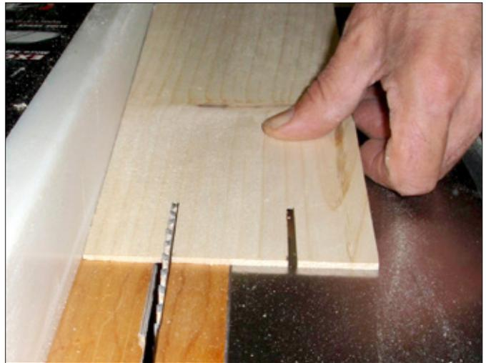
5. This shows the ramp after the grooves have been cut.
