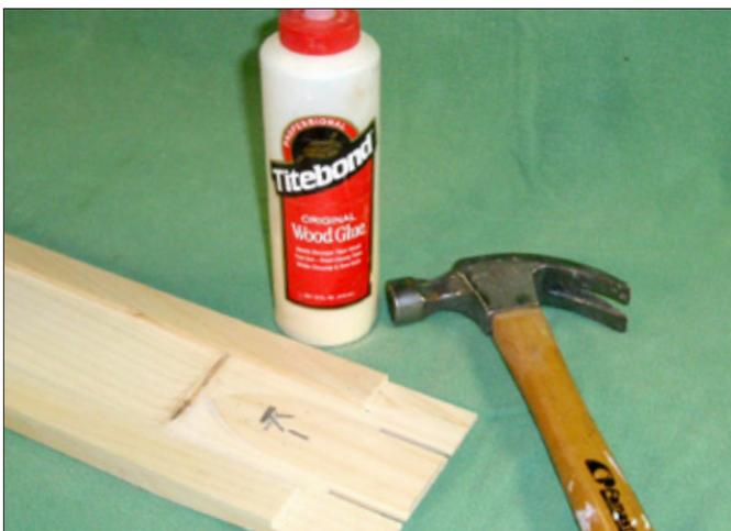
8. Center the inner wheel guide on the ramp. Glue and tack it in place. Note the taper of both sides of the upper  $1\frac{1}{2}$ " of the guide.
