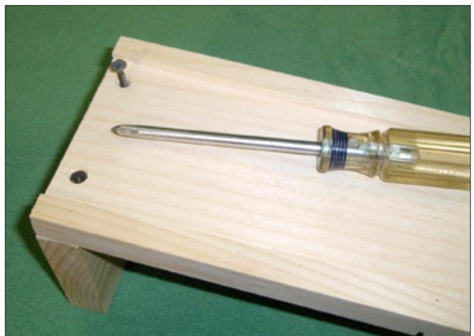
9. Drill and screw (or nail) the riser block to the upper end of the ramp. The block should have its top edge cut at a  $6^\circ$  angle to match the angle of the ramp.
