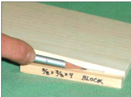
2. Use a  $\frac{3}{8}$ " x  $\frac{3}{8}$ " x 4" block to scribe the trim line on the bottom edge of the ramp. The block is positioned flush with the ramp end, then the ramp is raised until its bottom edge is even with the top edge of the block.
