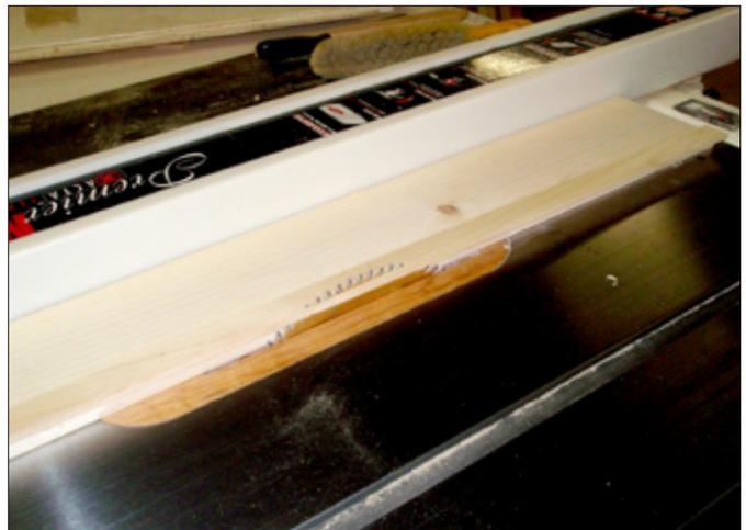
7. Glue one outer wheel guide to the ramp. At the top end, it should overhang the ramp about half its width. When the glue has dried, set the saw fence to the width of the ramp and cut off the overhang. Now repeat the process for the other side.
