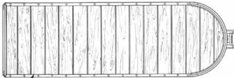
Platform boards are 3/4" oak, chassis and rack are of all-steel construction
