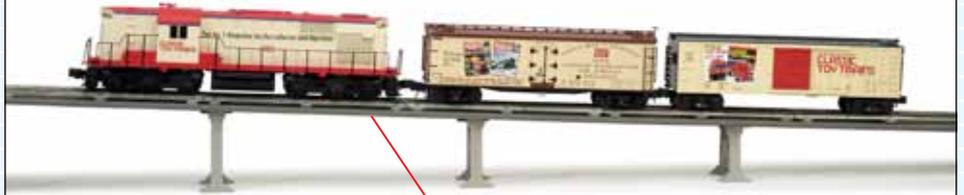
**Grades.** A grade greater than 5 percent (a 5-inch rise over a 100-inch run) can present a challenge to operation. For more reliable running, keep the grade to 4 percent or less.
